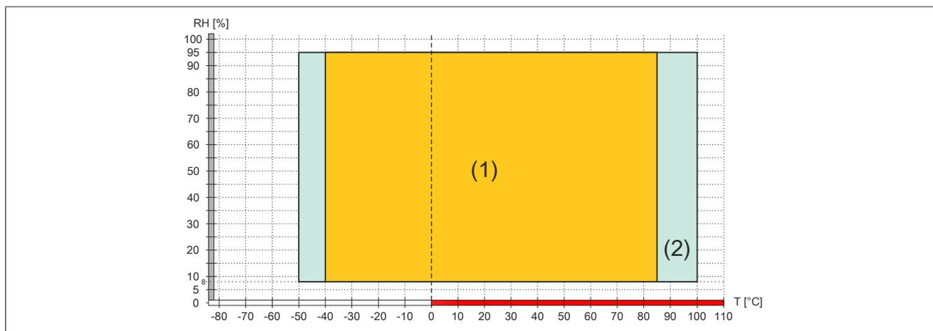
Figure 2: 0CFCRD.xxxxE.01 CompactFlash cards - Temperature/Humidity diagram
