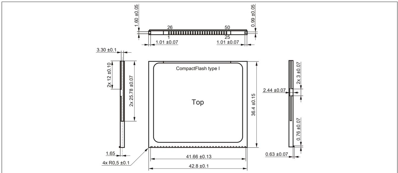
Figure 1: CompactFlash card type I dimensions
