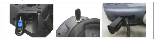
Figure 31: USB interface - Connecting the USB device
