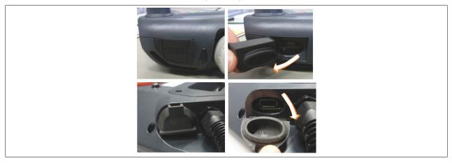
Figure 29: USB interface - Opening the protective cover
