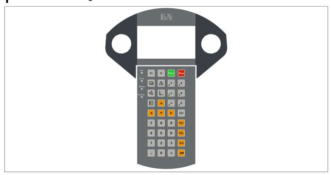
Figure 7: MP7120 - Membrane keypad
