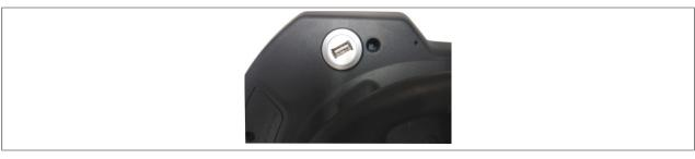
Figure 30: USB interface - Freely accessible interface
