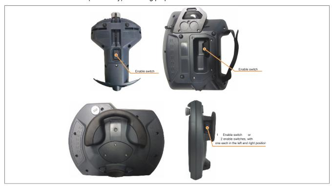
Figure 3: Enabling control device
