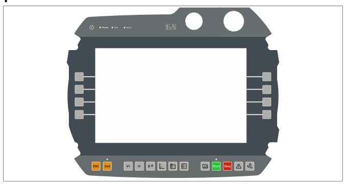
Figure 11: MP7151 - Membrane keypad
