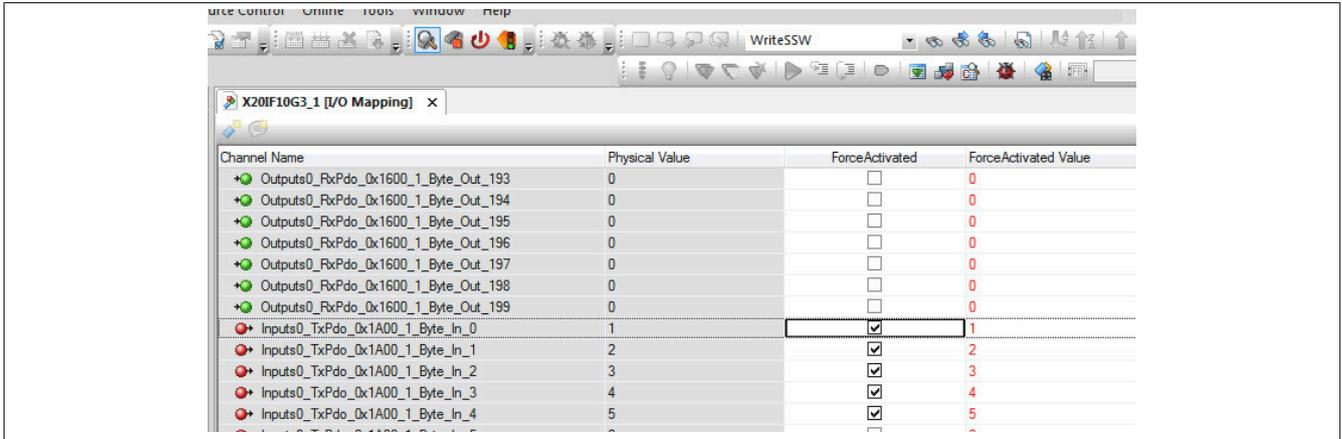
● The input data in the TwinCAT environment can be read for verification. To do so, double-click on TxPDO (input data) of the EtherCAT slave to open it. The input data can be read in column "Online".
