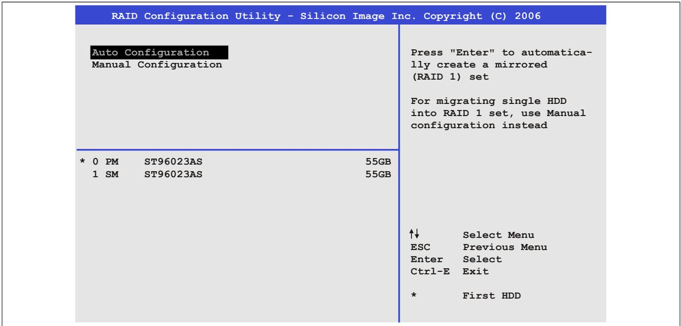
Abbildung 75: RAID Configuration Utility - Create RAID set - Mirrored
