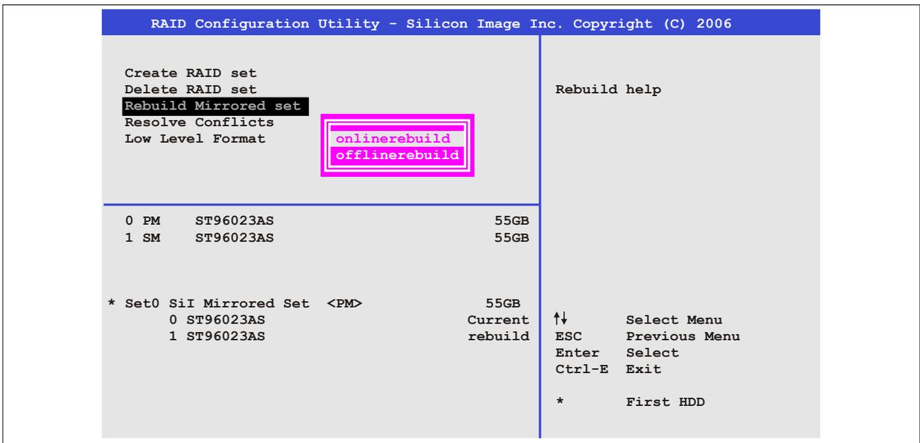
Abbildung 77: RAID Configuration Utility - Rebuild Mirrored set
