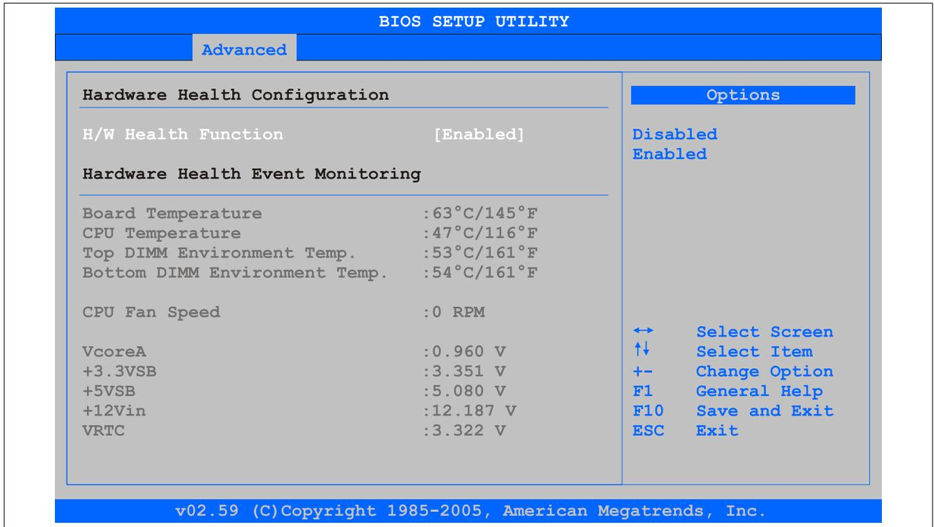
Abbildung 100: GM45 Advanced CPU Board Monitor
