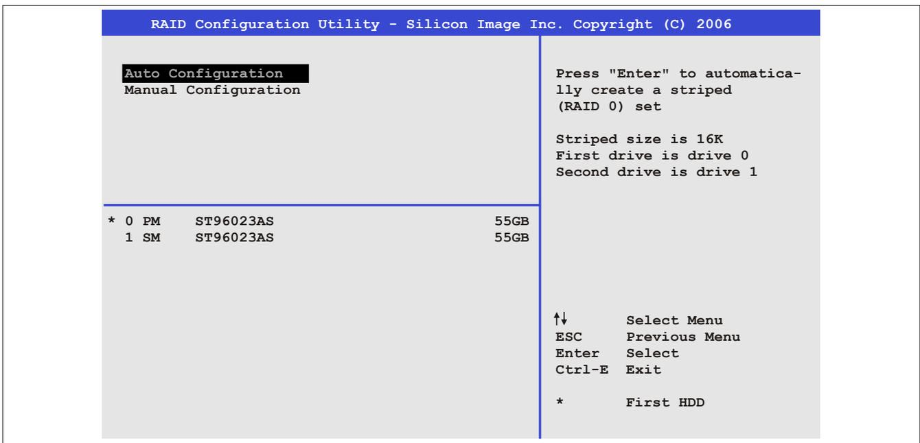
Abbildung 74: RAID Configuration Utility - Create RAID set - Striped
