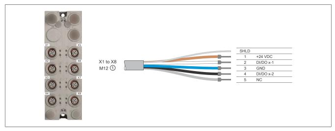
① X67CA0A41.xxxx: M12 sensor cable, straight X67CA0A51.xxxx: M12 sensor cable, angled
