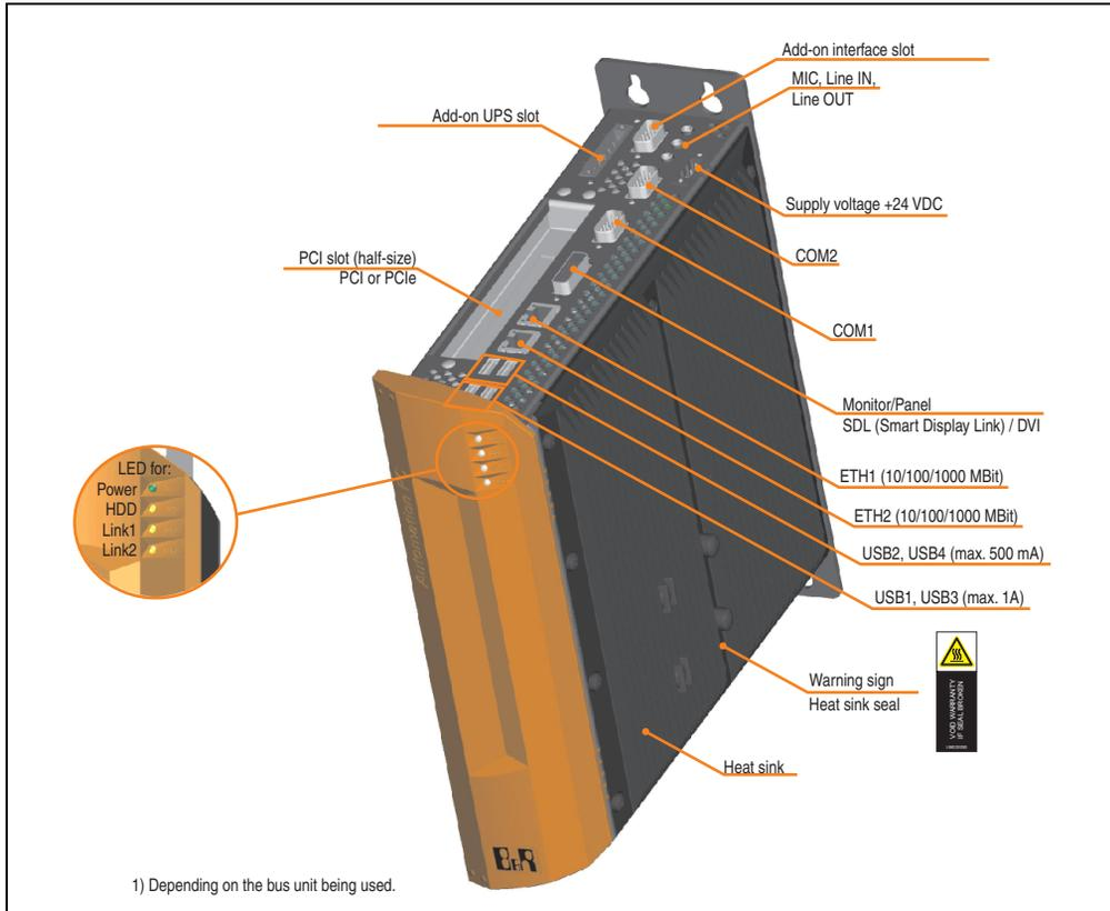
Figure 5: Interface overview - APC810, 1 card slot variant (top)
