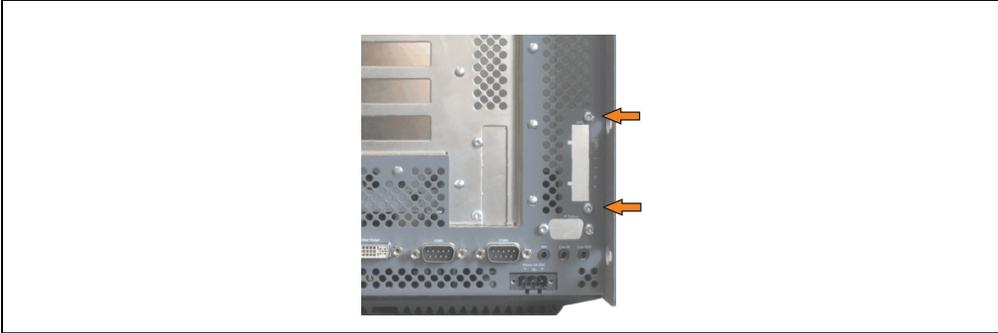
Figure 238: Remove UPS module cover
