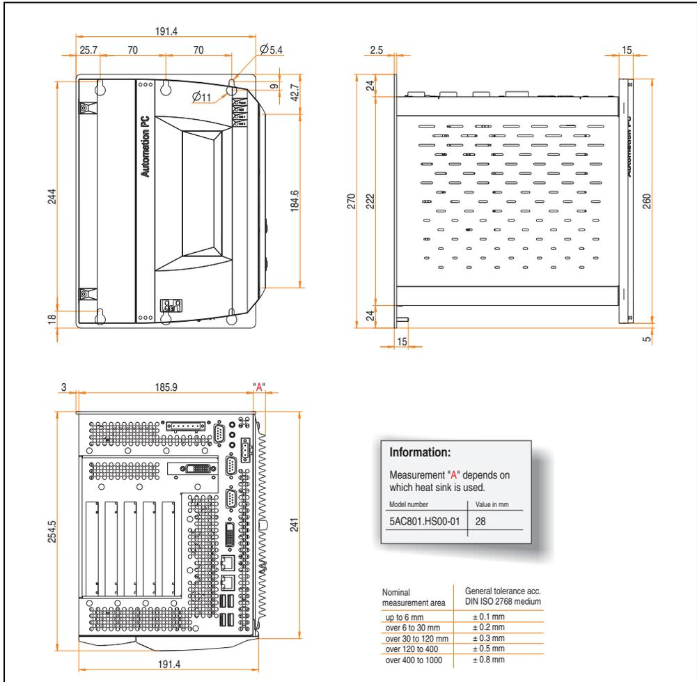
Figure 13: Dimensions - APC810 5 card slot variant
