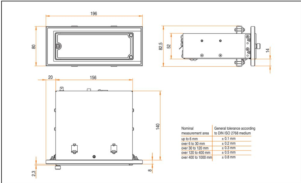
Figure 161: Dimensions - USB Media Drive with front cover
