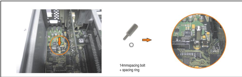
Figure 233: Screw in spacing bolt and spacing ring
