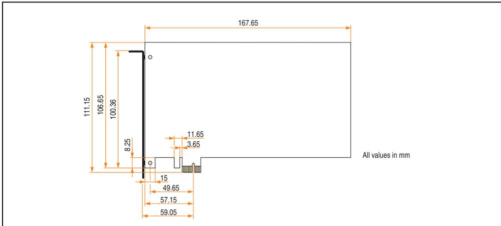
Figure 32: Dimensions - Standard half-size PCIe card
