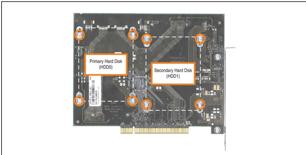
Figure 266: Screw layout on the back side of the SATA RAID controller 5ACPCI.RAIC-03
