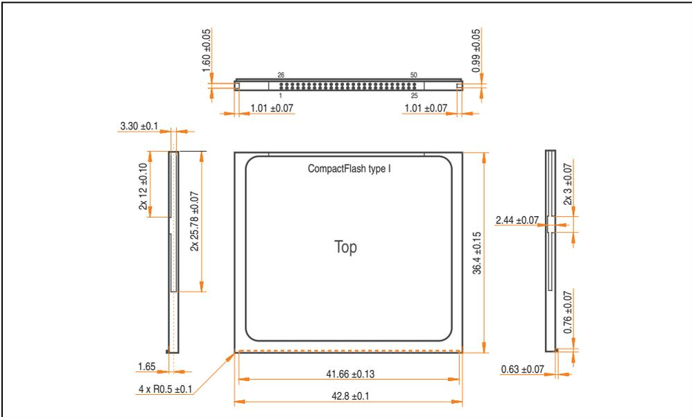
Figure 158: Dimensions - CompactFlash card Type I
