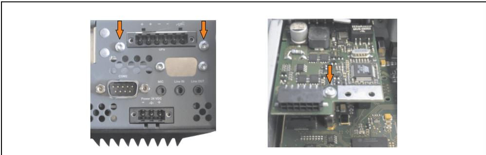
Figure 229: Install UPS module
