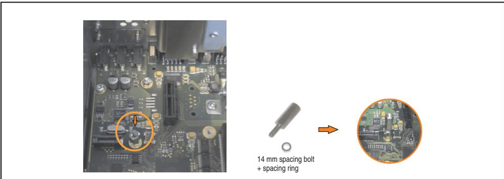
Figure 239: Screw in spacing bolt and spacing ring
