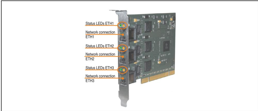
Figure 181: PCI Ethernet card 10/100 - 5ACPCI.ETH3-01
