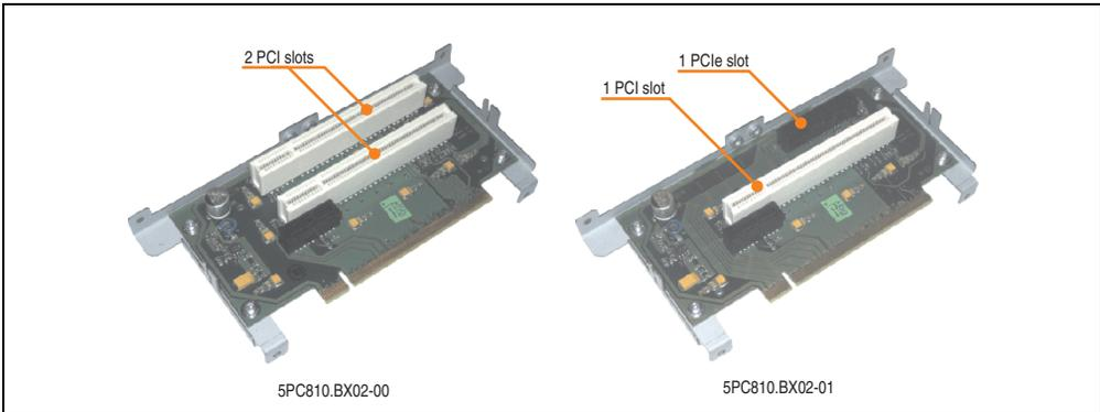
Figure 35: 2 slot bus units
