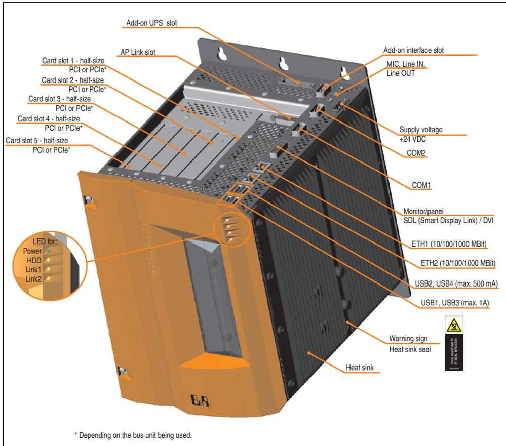
Figure 11: Interface overview - APC810, 5 card slot variant (top)
