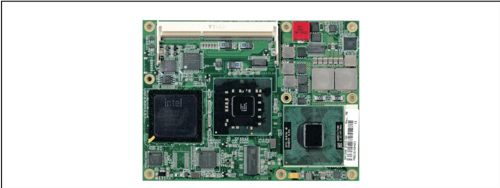
Figure 37: BM45 CPU board
