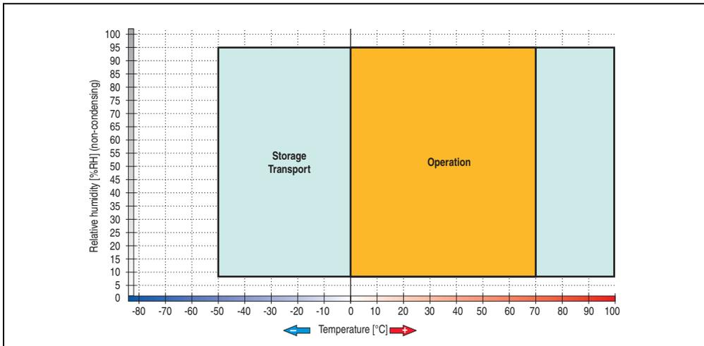
Figure 157: Temperature humidity diagram - CompactFlash cards 5CFCRD.xxxx-03
