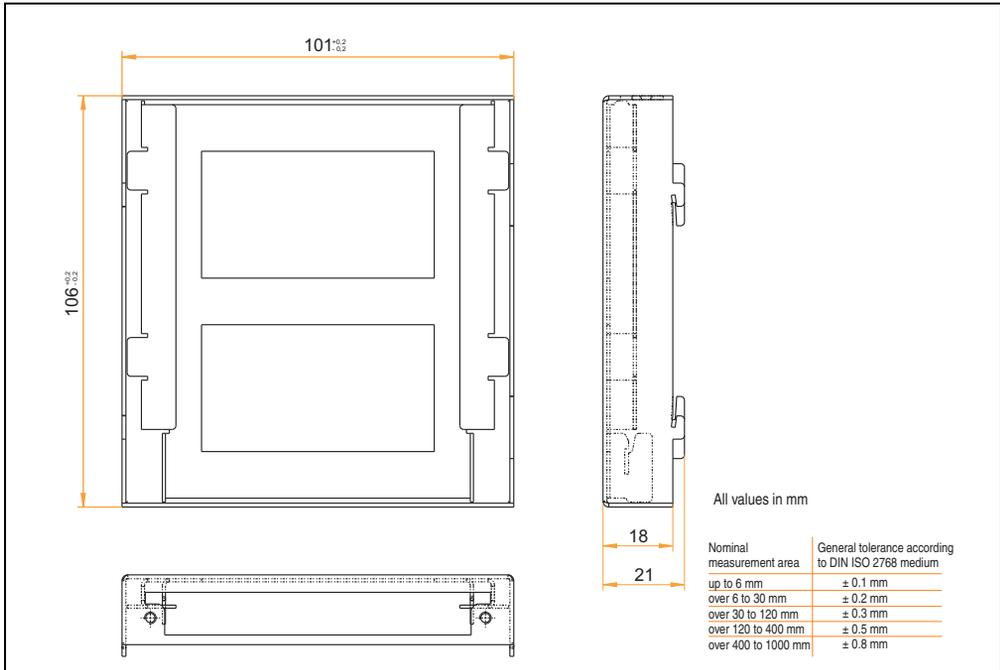
Figure 211: Dimensions - HDD replacement disk tray
