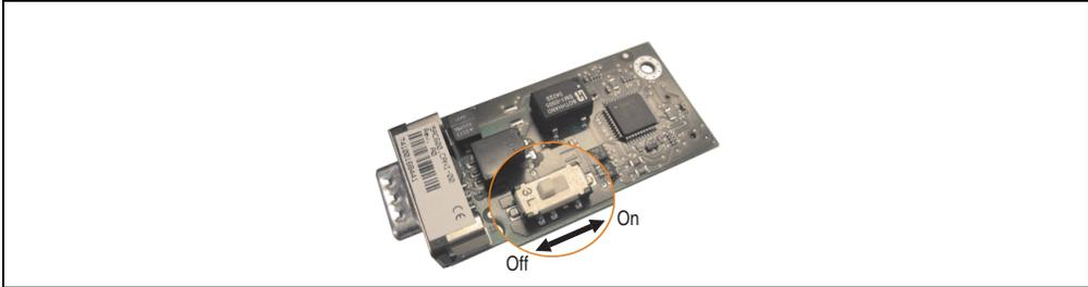
Figure 67: Terminating resistor - Add-on CAN interface 5AC600.CANI-00
