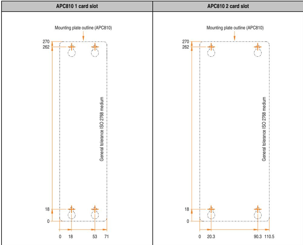
Table 79: Drilling templates - 1 and 2 card slot system units
