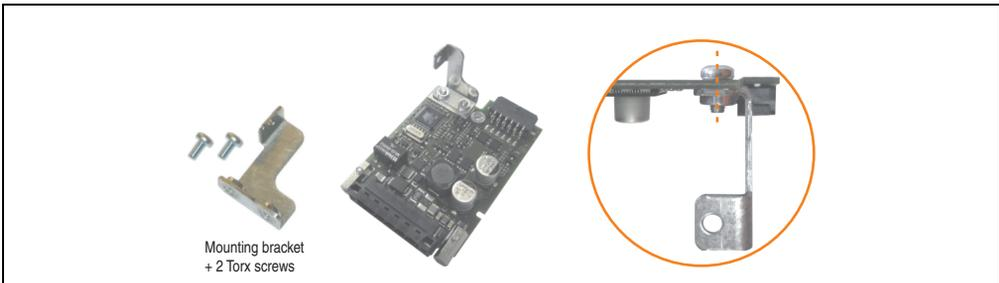
Figure 257: Install mounting bracket
