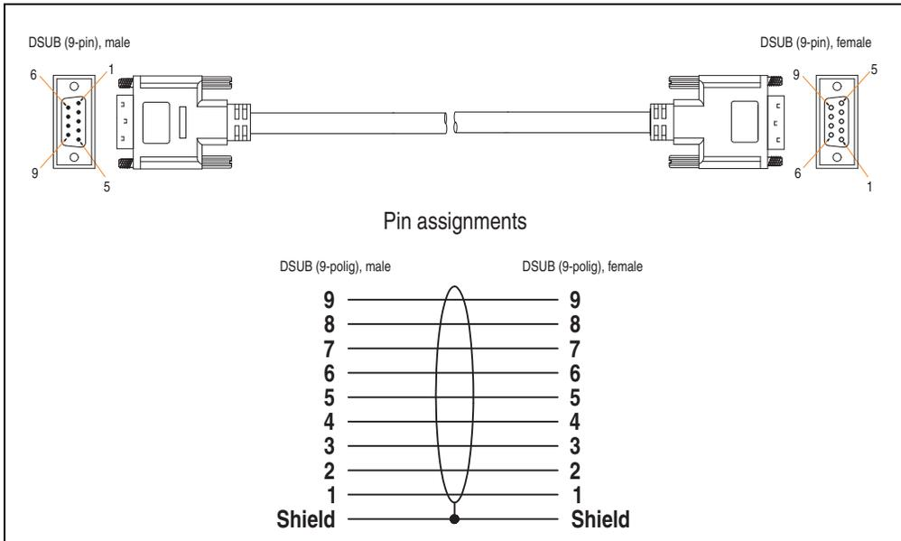
Figure 206: Pin assignments - RS232 cables 9A0014.xx
