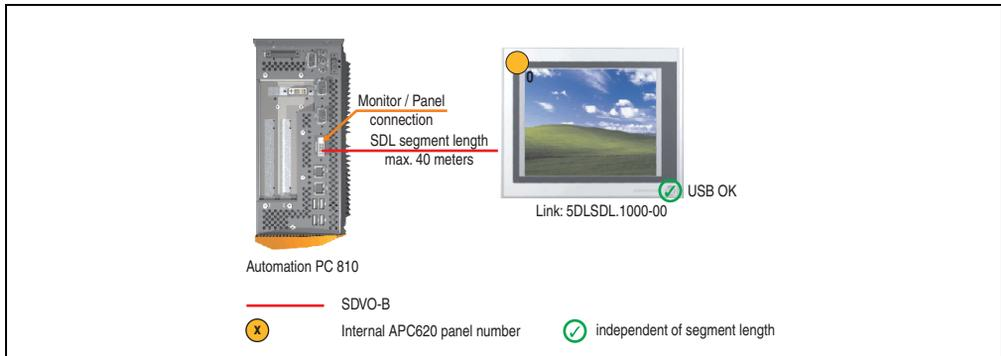
Figure 78: Configuration - An Automation Panel 900 via SDL (onboard)
