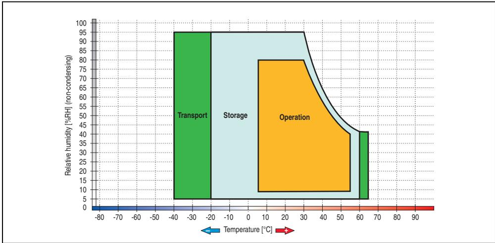
Figure 52: Temperature humidity diagram - Slide-in DVD-ROM/CD-RW - 5AC801.DVDS-00
