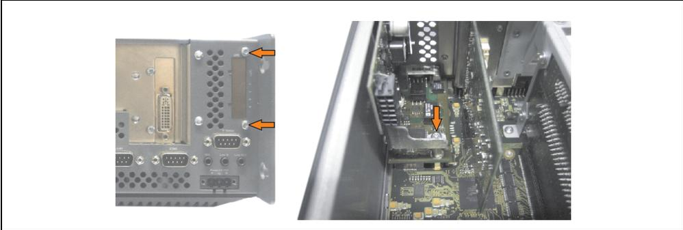
Figure 252: Install UPS module
