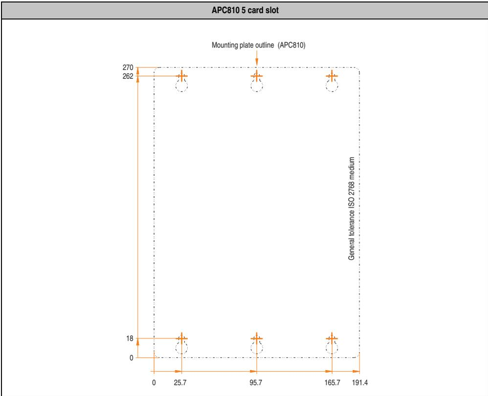
Table 80: Drilling template - 5 card slot system unit
