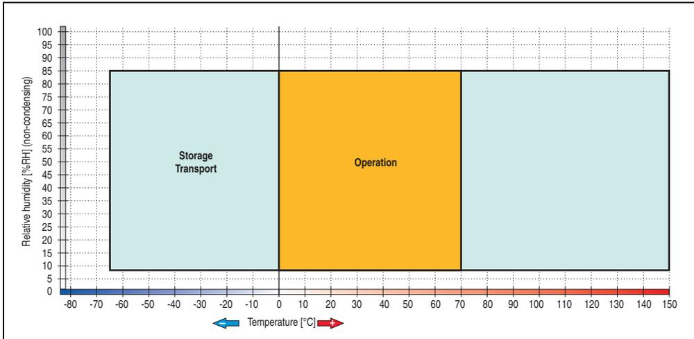
Figure 153: Temperature humidity diagram - CompactFlash cards 5CFCRD.xxxx-04
