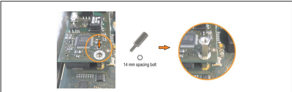
Figure 245: Screw in spacing bolt
