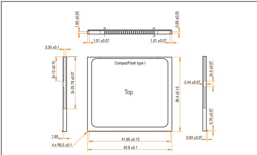
Figure 154: Dimensions - CompactFlash card Type I
