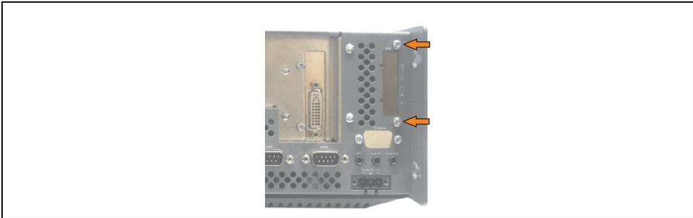
Figure 232: Remove UPS module cover
