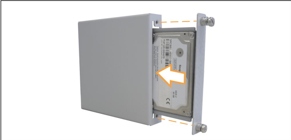
Figure 268: Installing the replacement hard disk in the replacement disk tray
