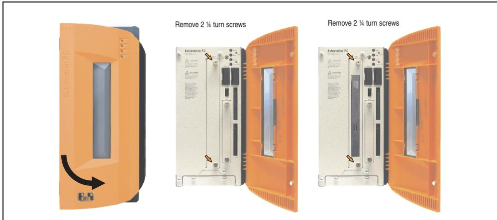
Figure 218: Loosening the ¼ turn screws
