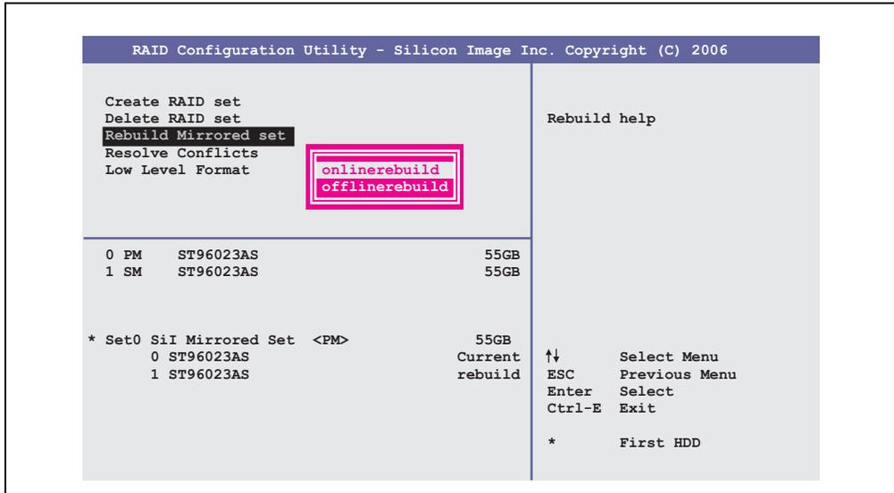
Figure 96: RAID Configuration Utility - Rebuild mirrored set
