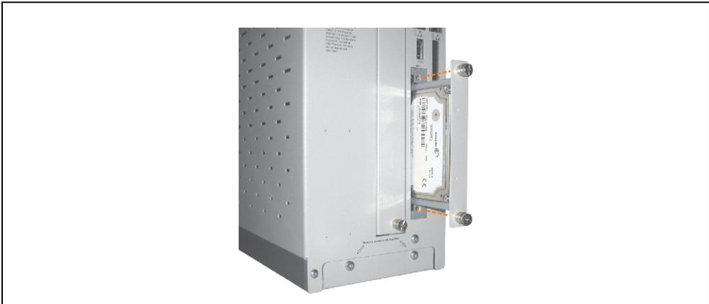
Figure 217: Inserting the compact SATA drive
