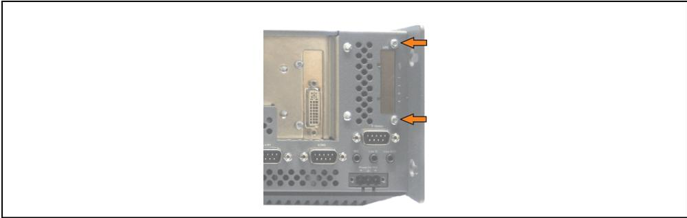
Figure 255: Remove UPS module cover
