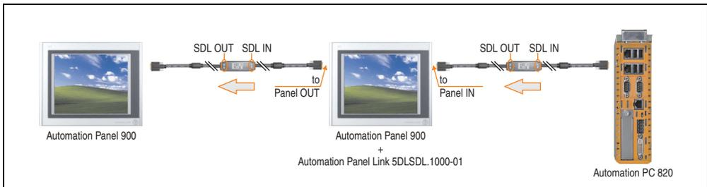
Figure 203: Example of signal direction display - SDL flex cable with extender
