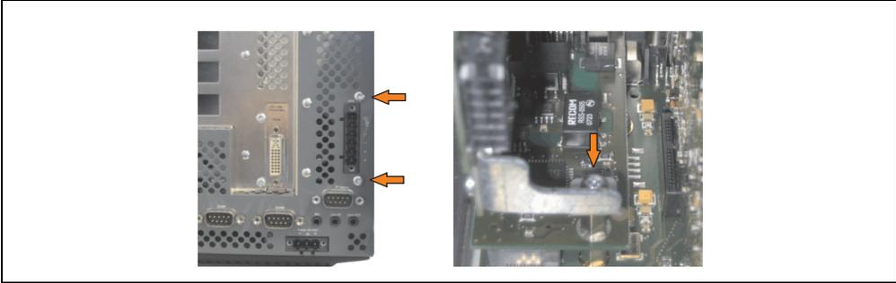
Figure 258: Install UPS module
