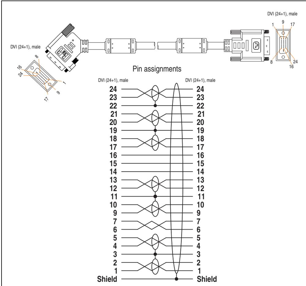
Figure 194: Pin assignments - SDL cable with 45° plug 5CASDL.0xxx-01
