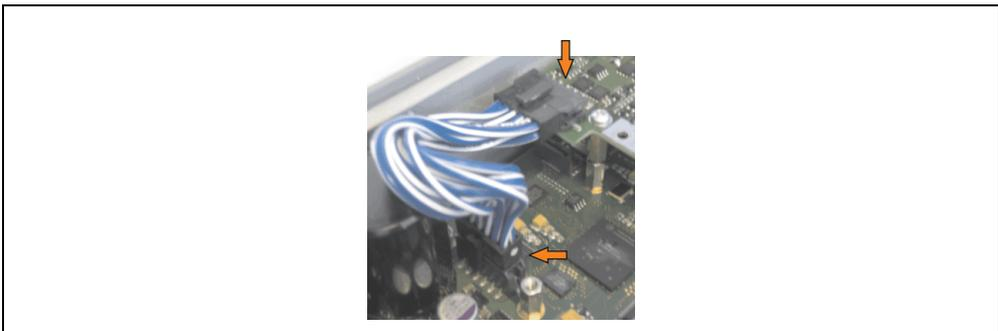
Figure 230: Plug in connection cable
