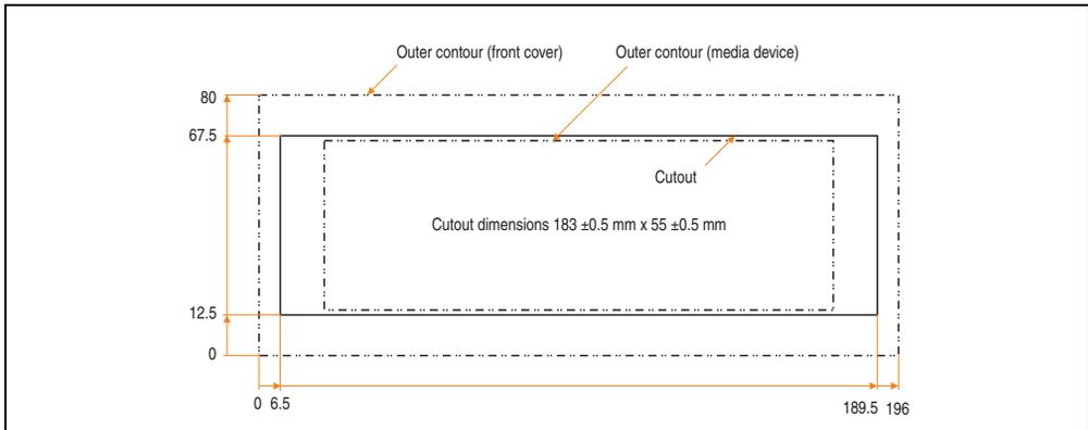
Figure 162: Installation cutout - USB Media Drive with front cover
