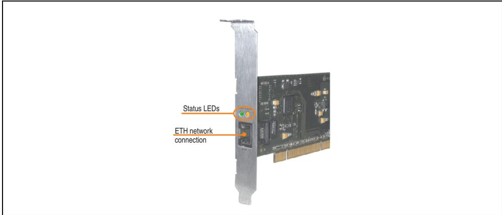
Figure 179: PCI Ethernet card 10/100 - 5ACPCI.ETH1-01
