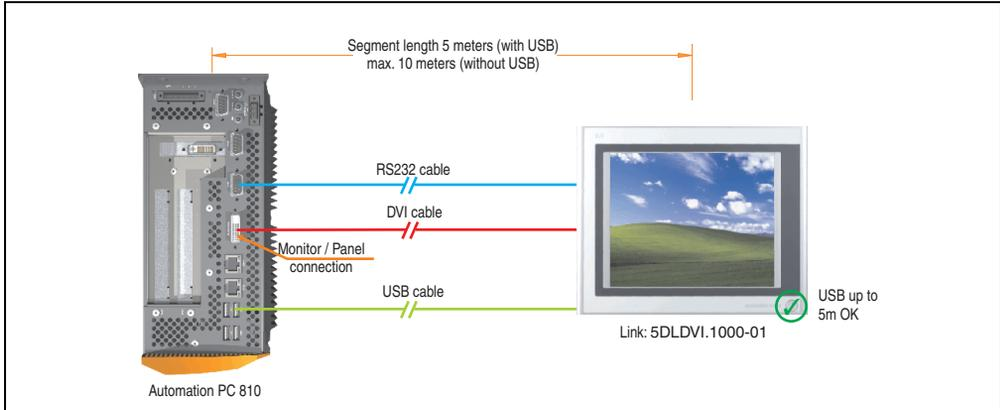
Figure 77: Configuration - One Automation Panel 900 via DVI (onboard)
