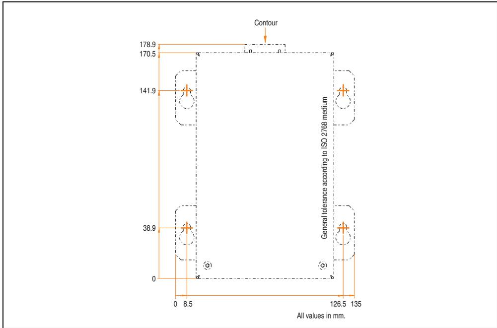
Figure 176: Drilling template for the battery unit
