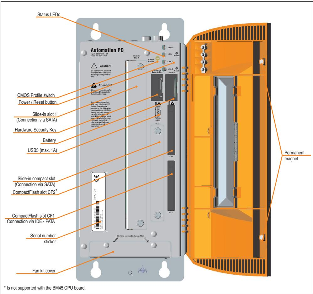
Figure 9: Interface overview - APC810, 2 card slot variant (bottom)
