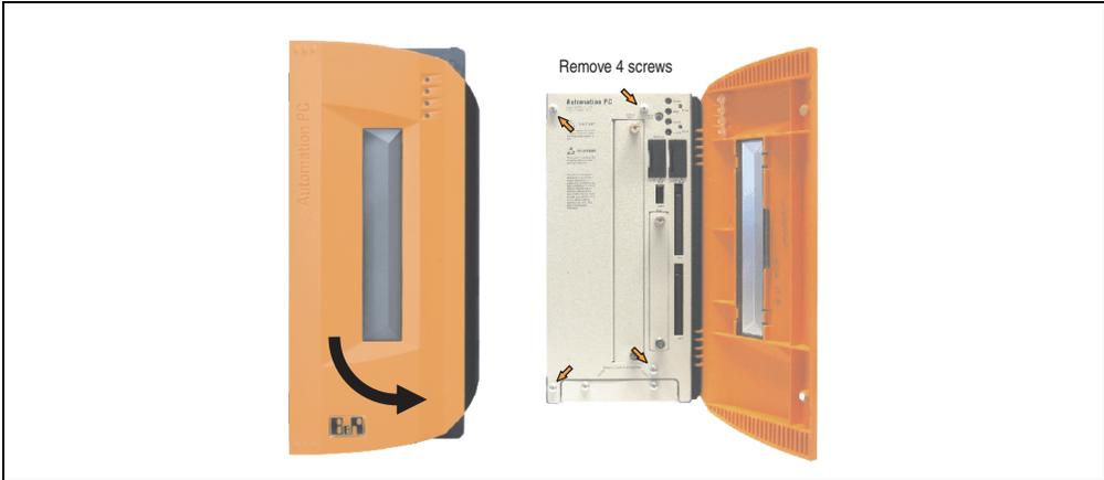
Figure 262: Mounting the side cover - APC810 2 card slot
