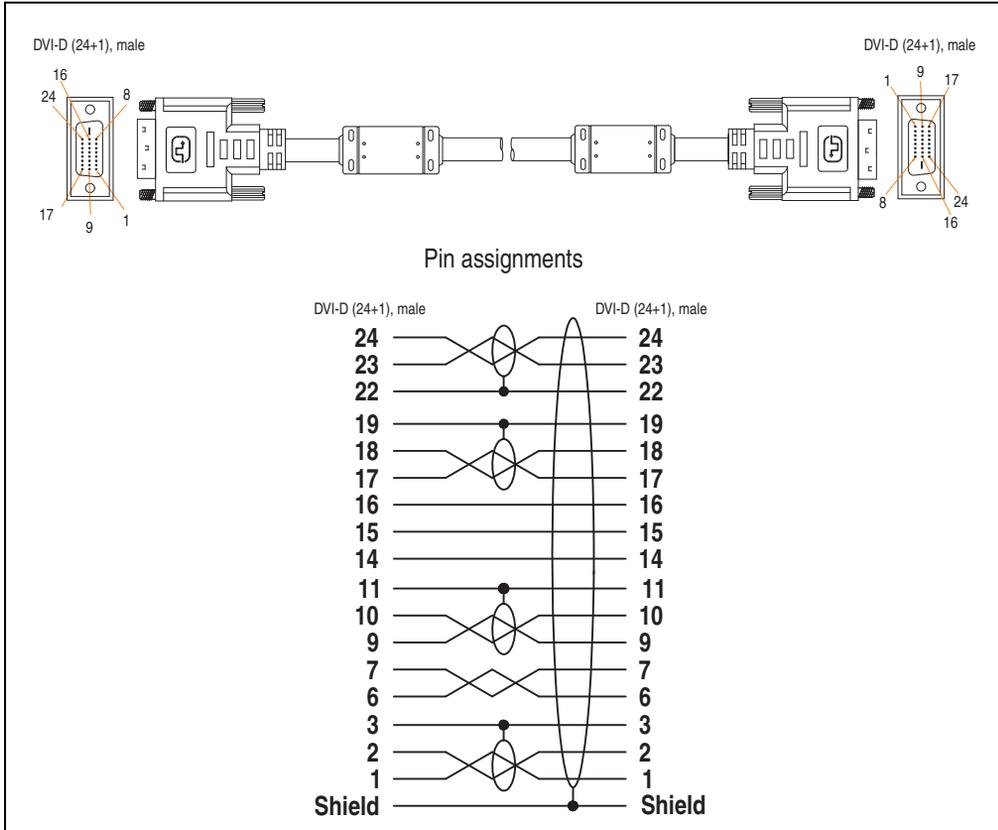
Figure 186: Pin assignments - DVI cable 5CADVI.0xxx-00
