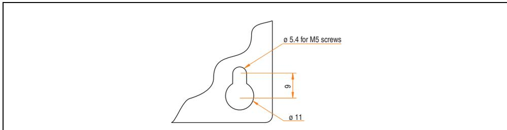
Figure 71: Mounting plates
