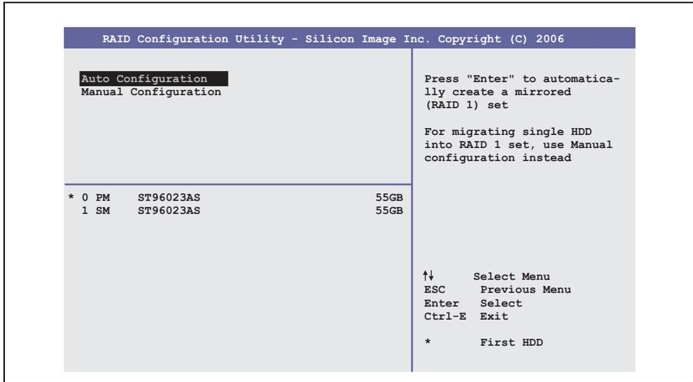
Figure 94: RAID Configuration Utility - Create RAID set - Mirrored
