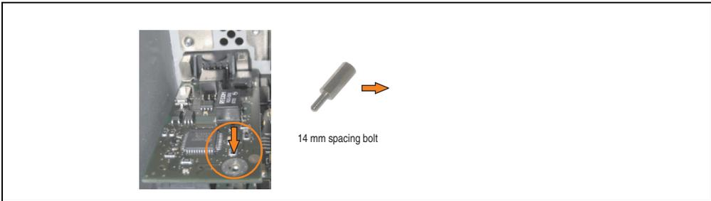
Figure 256: Screw in spacing bolt
