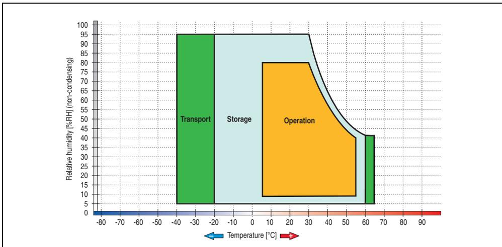
Figure 54: Temperature humidity diagram - Slide-in DVD-R/RW, DVD+R/RW - 5AC801.DVRS-00
