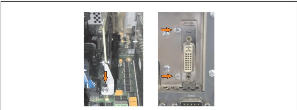
Figure 265: Install AP Link module
