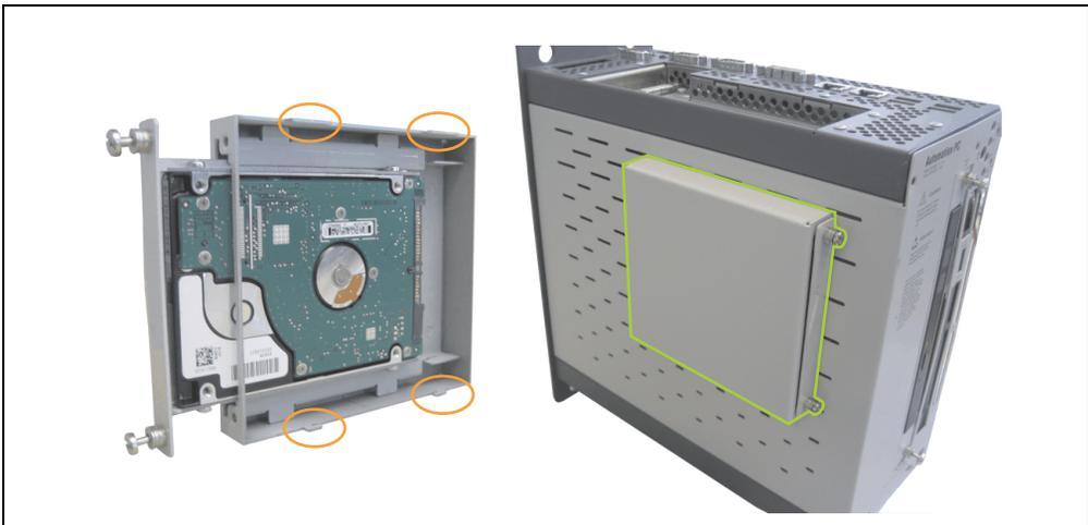
Figure 269: Installing the replacement disk tray in the APC810
