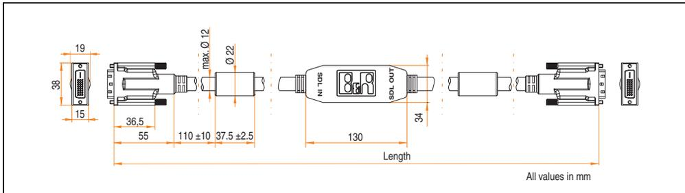
Figure 201: Dimensions - SDL flex cable with extender 5CASDL.0xx0-13
