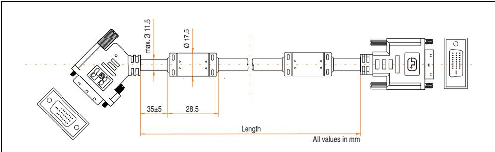
Figure 193: Dimensions - SDL cable with 45° plug 5CASDL.0xxx-01
