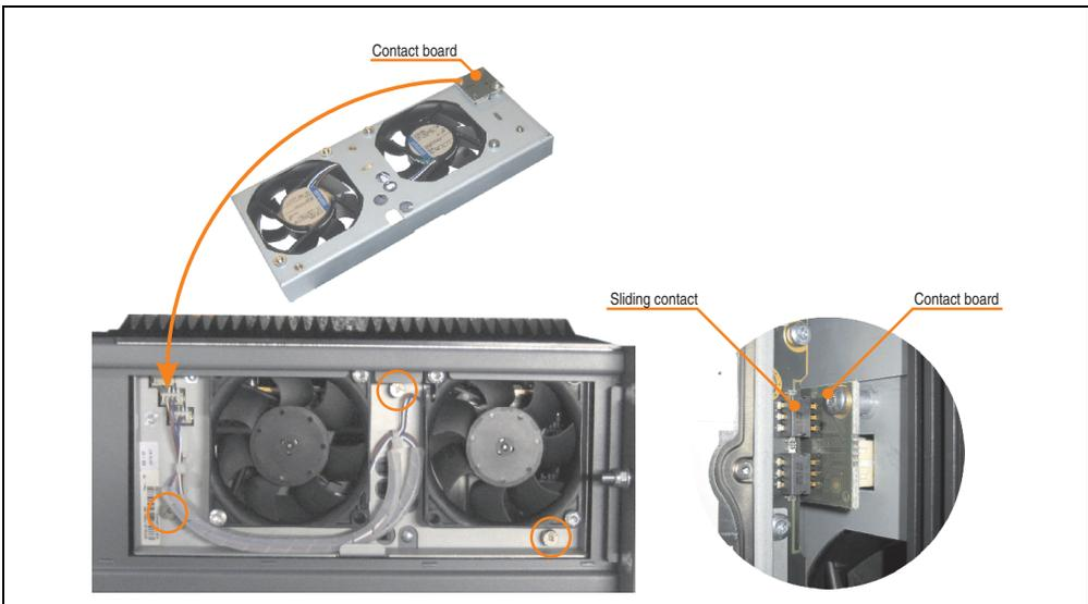
Figure 224: Inserting and fastening the fan kit
