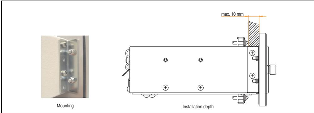
Figure 167: Front cover mounting and installation depth
