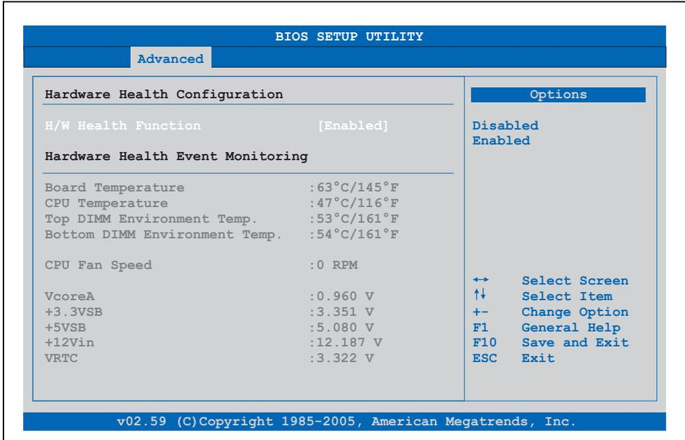
Figure 119: BM45 - Advanced CPU board monitor
