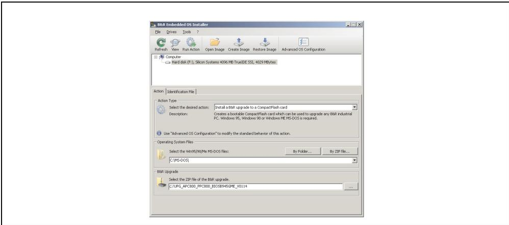
Figure 140: Creating a CompactFlash card for B&R upgrade files
