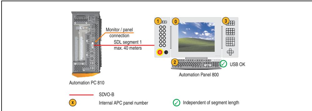
Figure 79: Configuration - An Automation Panel 800 via SDL (onboard)
