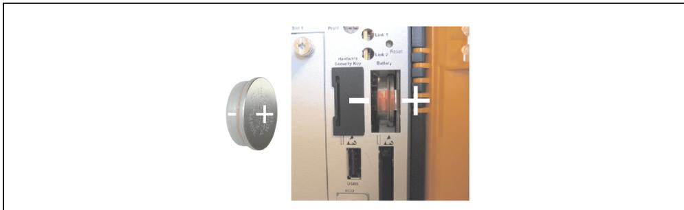
Figure 215: Battery polarity
