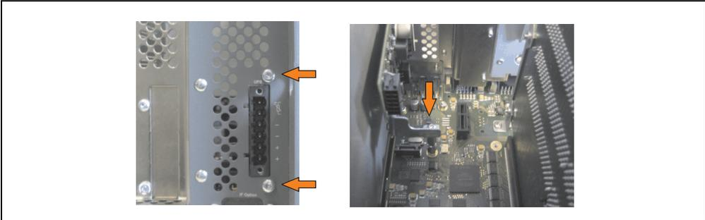
Figure 241: Install UPS module
