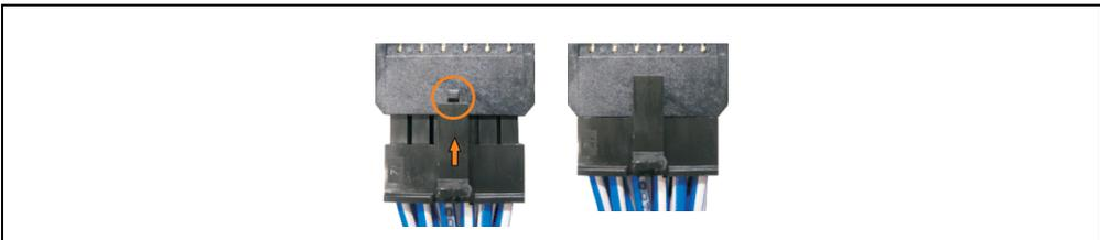
Figure 243: Connector locking mechanism
