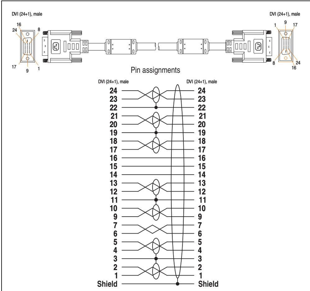
Figure 190: Pin assignments - SDL cable 5CASDL.0xxx-00
