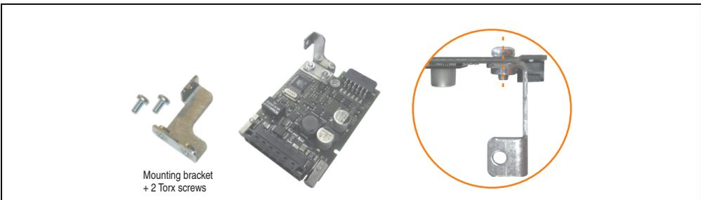
Figure 240: Install mounting bracket
