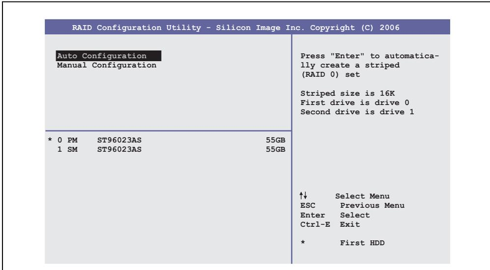
Figure 93: RAID Configuration Utility - Create RAID set - Striped
