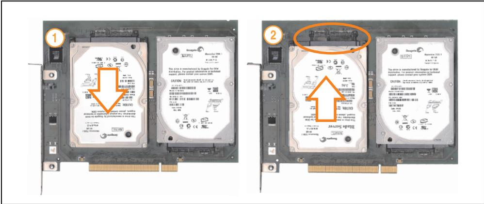
Figure 267: Hard disk exchange
