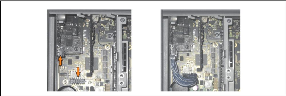
Figure 253: Plug in connection cable
