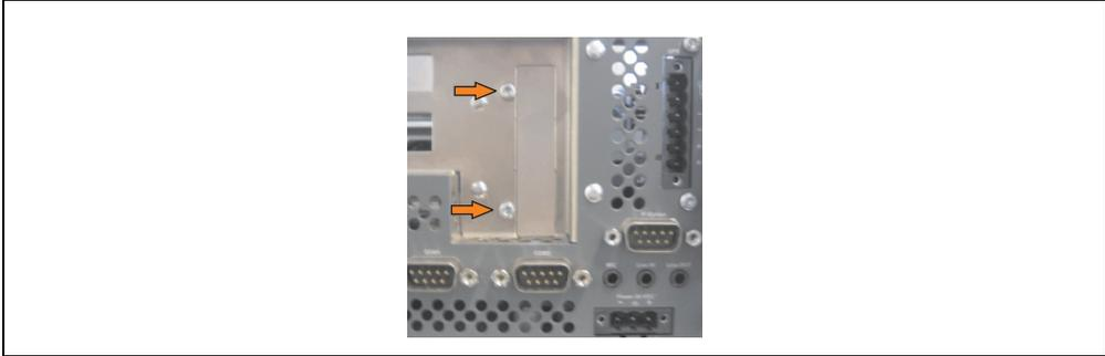
Figure 264: Remove AP Link module cover
