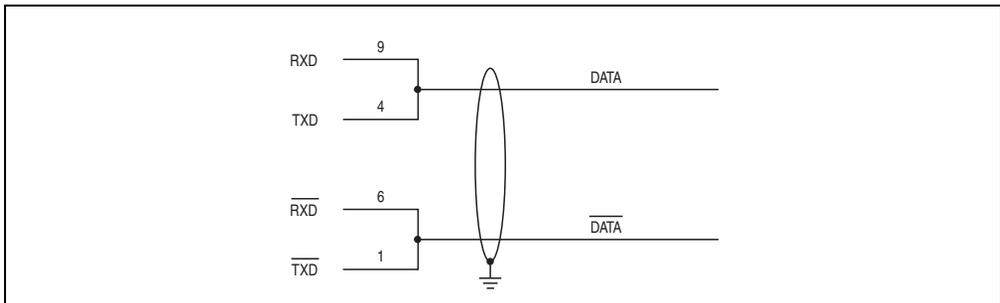
Figure 69: Add-on RS232/422/485 interface - operated in RS485 mode
