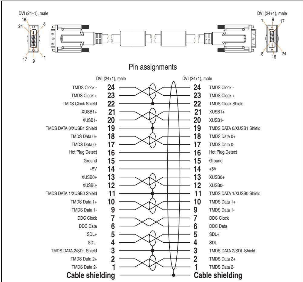
Figure 198: Pin assignments - SDL flex cable 5CASDL.0xxx-03
