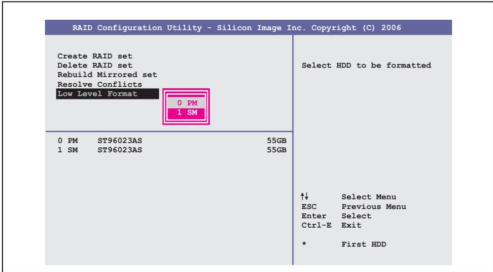
Figure 98: RAID Configuration Utility - Low level format
