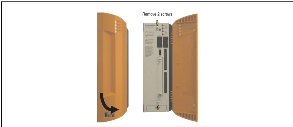
Figure 261: Mounting the side cover - APC810 1 card slot
