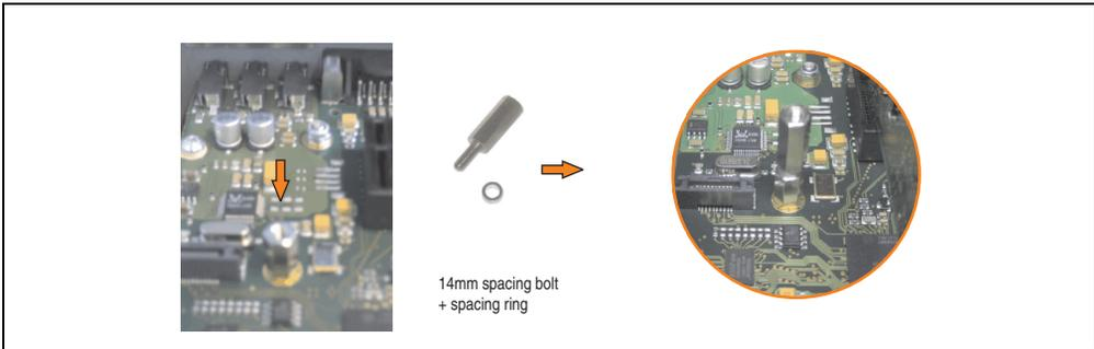
Figure 228: Screw in spacing bolt and spacing ring
