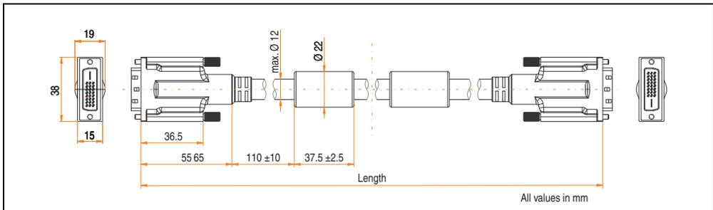
Figure 197: Dimensions - SDL flex cable 5CASDL.0xxx-03
