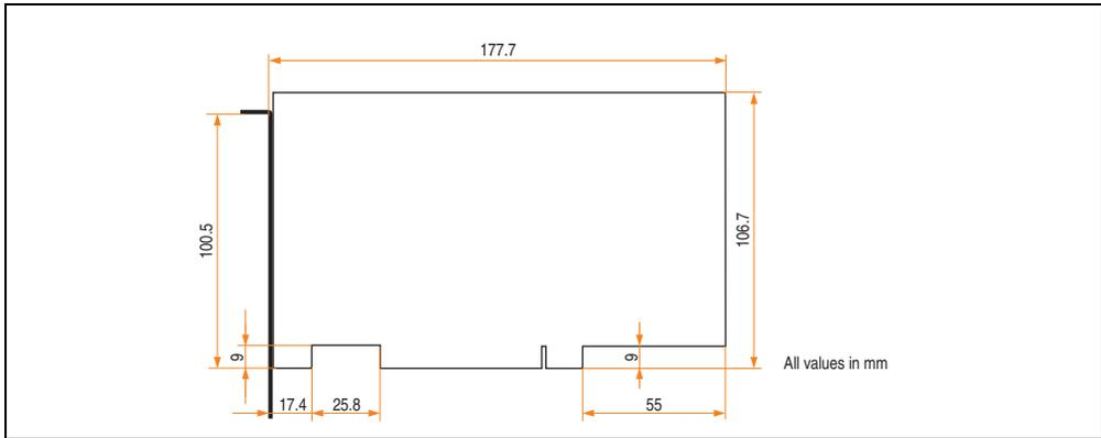
Figure 31: Dimensions - Standard half-size PCI card
