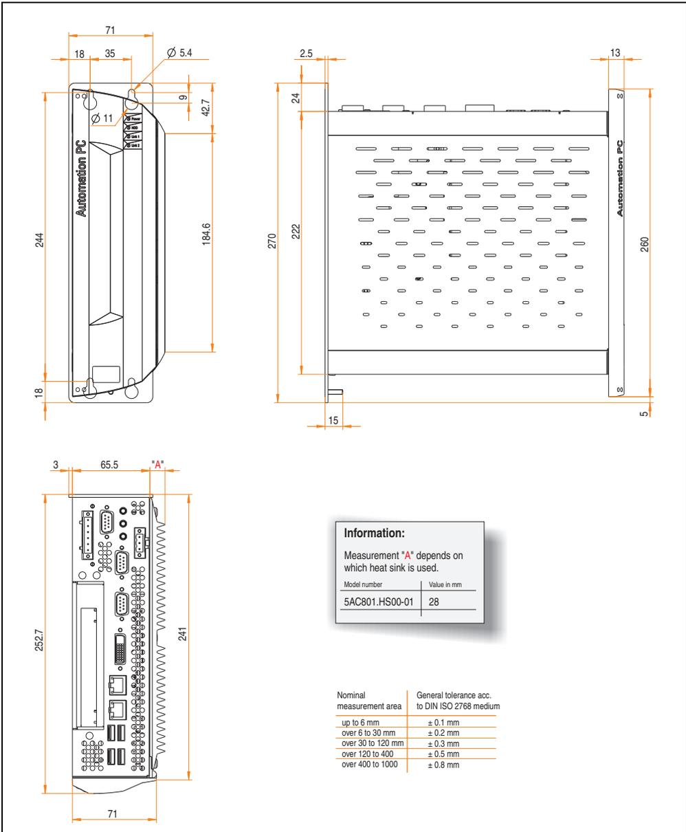
Figure 7: Dimensions - APC810 1 card slot variant
