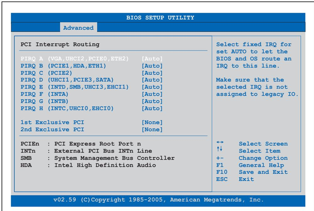
Figure 105: BM45 - Advanced PCI interrupt routing
