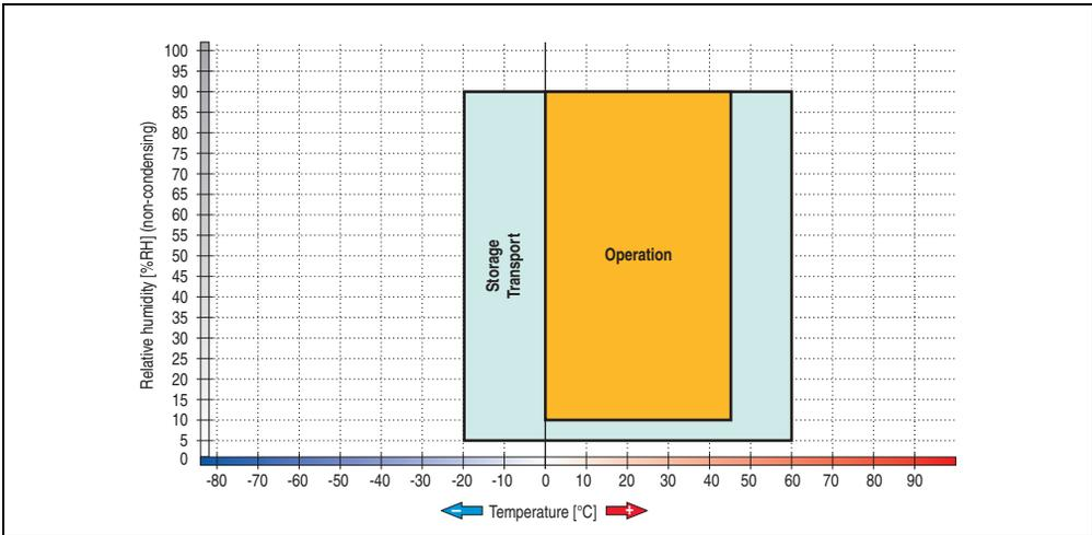
Figure 168: Temperature humidity diagram - USB flash drive - 5MMUSB.2048-00
