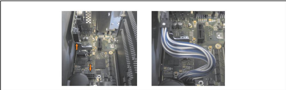
Figure 242: Plug in connection cable
