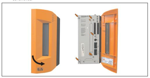
Figure 320: Mounting the side cover - APC620, 2 PCI slot
