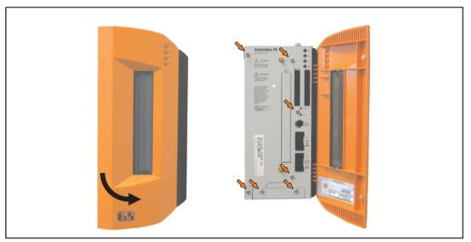
Figure 256: APC620 2PCI slots - Remove screws to install/ remove filter kit
