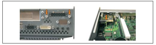
Figure 283: Install UPS module
