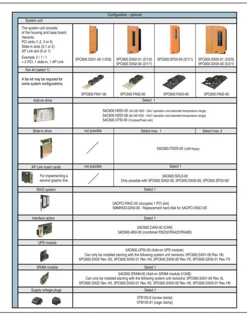
Figure 5: Selection guide - APC620 optional components with 1, 2, 3, and 5 PCI slots
