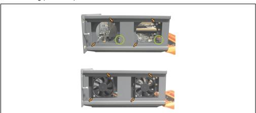
Figure 259: APC620 2PCI slots - Fan installation
