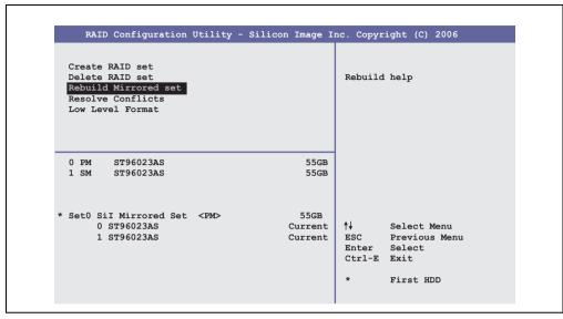
Figure 115: RAID Configuration Utility - Rebuild mirrored set
