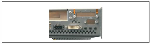
Figure 281: Remove UPS module cover
