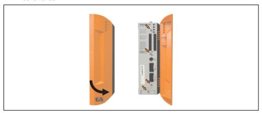
Figure 251: APC620 1PCI slot - Remove screws to install/ remove filter kit
