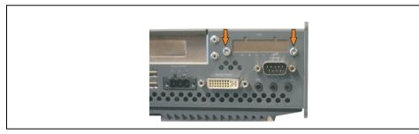
Figure 300: Remove UPS module cover
