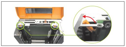
Figure 277: Release the slide-in slot releasing mechanisms
