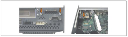
Figure 302: Install UPS module
