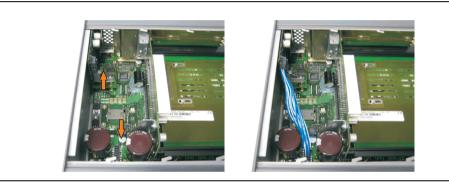
Figure 310: Plug in connection cable
