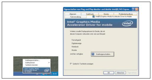
Figure 165: Accessing the graphics driver via Control Panel
