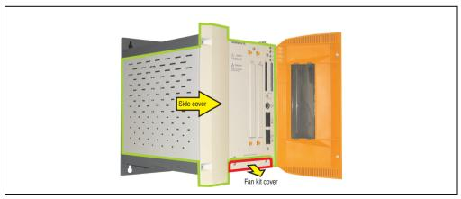
Figure 269: APC620 5PCI slot - Remove side cover and fan kit cover
