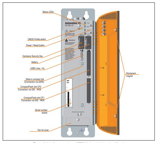
Figure 6: Interface overview - APC810, 1 card slot variant (front)
