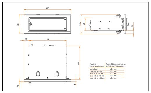
Figure 187: Dimensions - USB Media Drive with front cover
