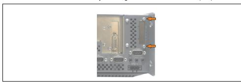
Figure 282: Remove UPS module cover
