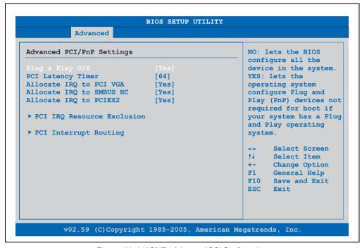
Figure 126: 945GME - Advanced PCI Configuration
