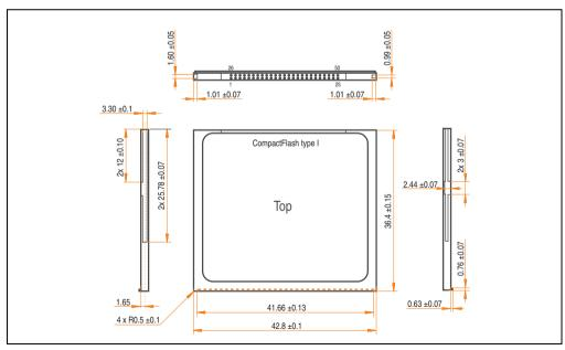
Figure 184: Dimensions - CompactFlash card Type I
