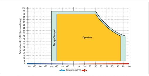
Figure 74: Temperature humidity diagram - SATA RAID hard disk 5ACPCI.RAIC-03
