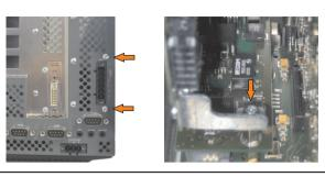
Figure 285: Install UPS module
