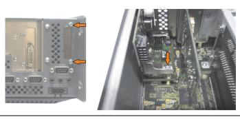
Figure 279: Install UPS module
