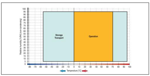
Figure 59: Temperature humidity diagram - 5AC801.SSDI-00
