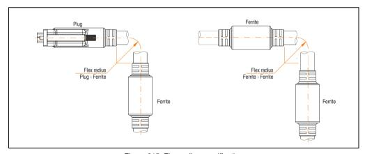
Figure 215: Flex radius specification
