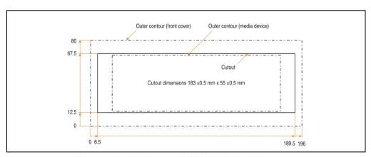
Figure 188: Installation cutout - USB Media Drive with front cover
