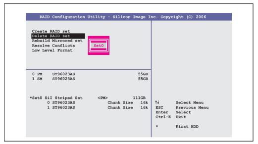
Figure 118: RAID Configuration Utility - Delete RAID set
