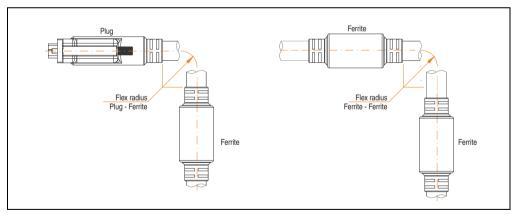
Figure 219: Flex radius specification
