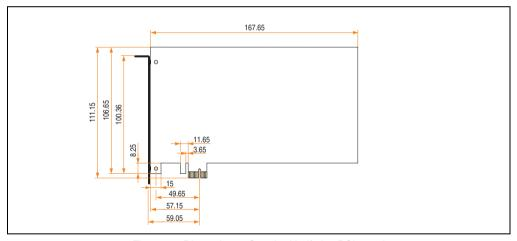
Figure 41: Dimensions - Standard half-size PCIe card
