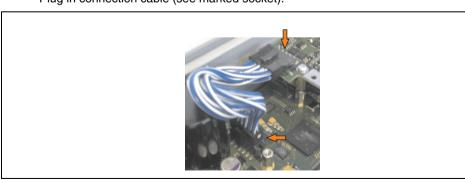
Figure 257: Plug in connection cable
