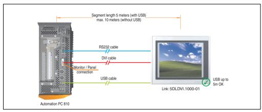
Figure 100: Configuration - One Automation Panel 900 via DVI (onboard)
