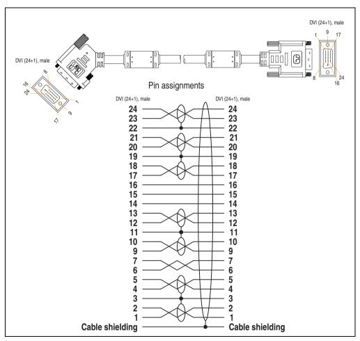
Figure 221: Pin assignments - SDL cable with 45° plug 5CASDL.0xxx-01
