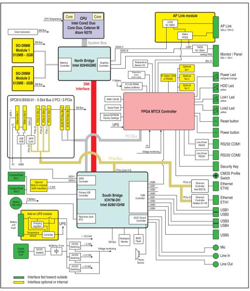
Figure 38: Block diagram 5PC810.SX05-00 + 5PC810.BX05-01
