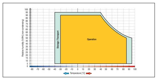
Figure 51: Temperature humidity diagram - 5AC801.HDDI-00
