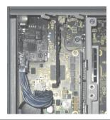
Figure 263: Plug in connection cable
