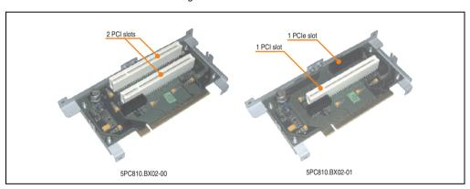
Figure 44: 2 slot bus units
