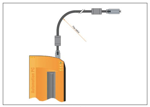
Figure 98: Flex radius - Cable connection
