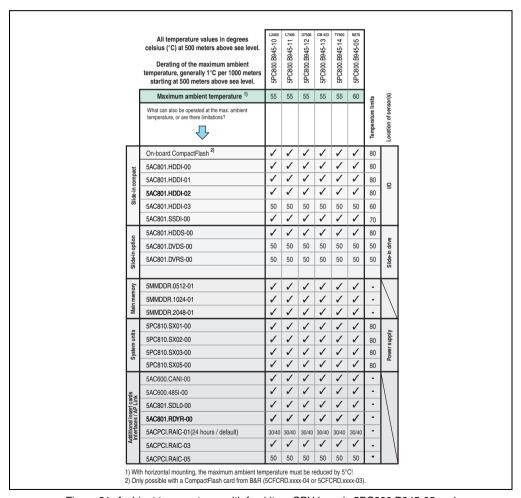
Figure 21: Ambient temperatures with fan kit on CPU boards 5PC800.B945-05 and 5PC800.B945-1x
