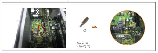
Figure 298: Screw in spacing bolt and spacing ring
