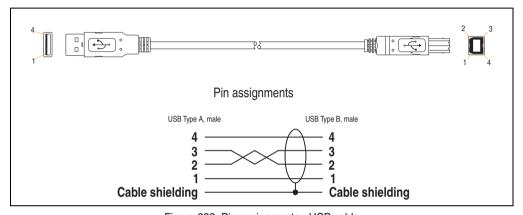
Figure 233: Pin assignments - USB cable
