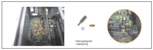
Figure 260: Screw in spacing bolt and spacing ring
