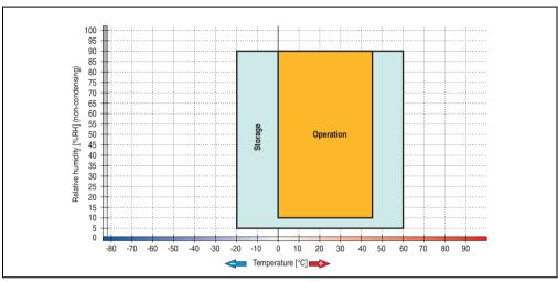
Figure 194: Temperature humidity diagram - USB flash drive - 5MMUSB.2048-00
