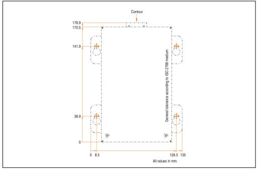
Figure 203: Drilling template for the battery unit
