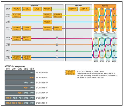
Figure 156: PCI and PCIe routing with activated APIC CPU boards B945GME (COM Express) for BIOS version 1.14
