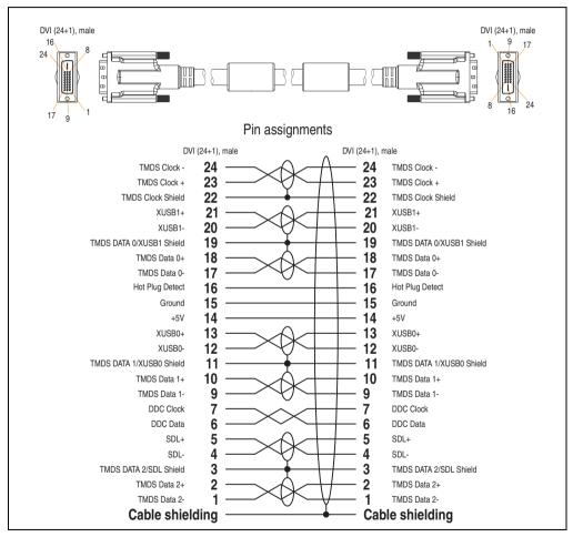
Figure 225: Pin assignments - SDL cable 5CASDL.0xxx-03
