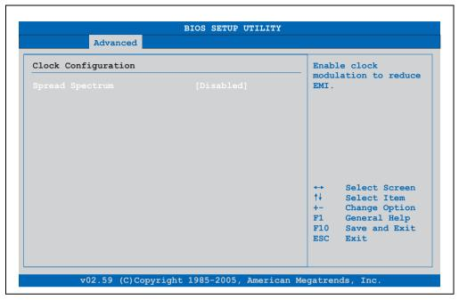
Figure 134: 945GME Advanced Clock Configuration
