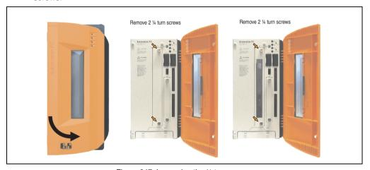
Figure 247: Loosening the 1/4 turn screws
