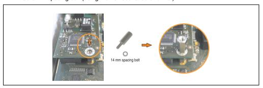
Figure 272: Screw in spacing bolt
