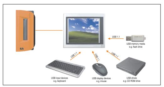
Figure 112: Remote connection of USB peripheral devices to the APC800/900 via SDL
