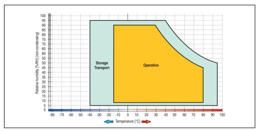
Figure 55: Temperature humidity diagram - 5AC801.HDDI-02
