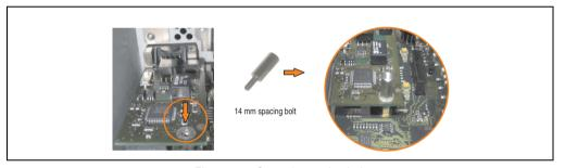
Figure 283: Screw in spacing bolt
