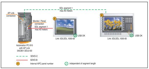
Figure 107: Configuration - Two Automation Panel 900 units via SDL (onboard) and SDL (AP Link)
