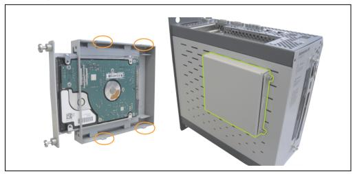
Figure 296: Installing the replacement disk tray in the APC810
