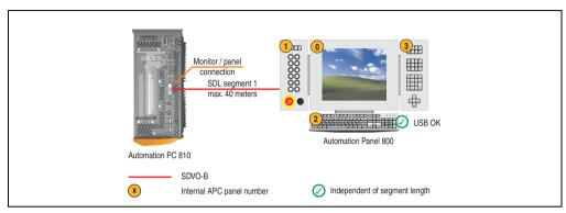
Figure 102: Configuration - An Automation Panel 800 via SDL (onboard)
