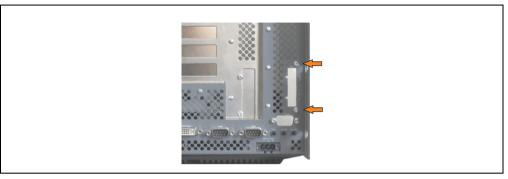
Figure 265: Remove UPS module cover
