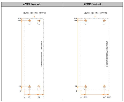
Table 95: Drilling templates - 1 and 2 card slot system units
