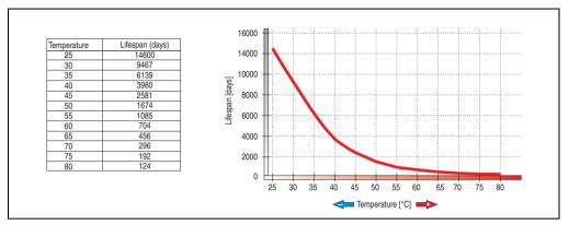
Figure 200: Temperature life span diagram
