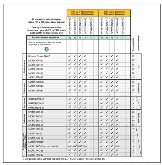
Figure 18: Ambient temperatures without a fan kit with heat sinks 5AC801.HS00-00 Rev. D0 and 5AC801.HS00-01 Rev. D0
