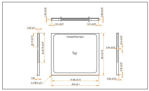
Figure 180: Dimensions - CompactFlash card Type I
