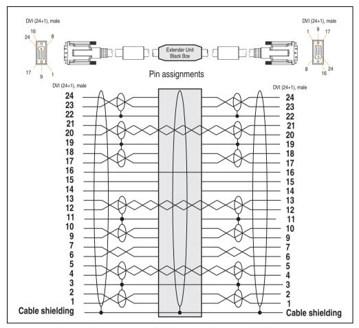
Figure 229: Pin assignments - SDL flex cable with extender 5CASDL.0x00-13
