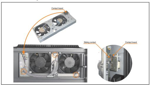
Figure 251: Inserting and fastening the fan kit
