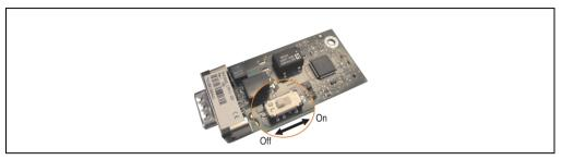
Figure 90: Terminating resistor - Add-on CAN interface 5AC600.CANI-00
