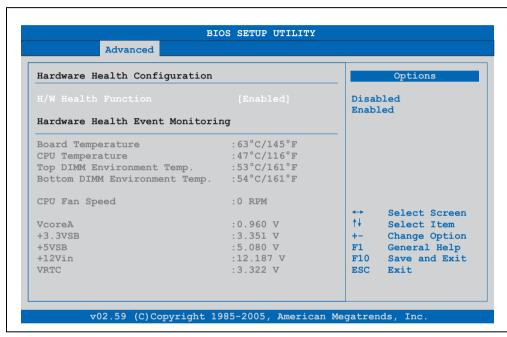
Figure 143: 945GME Advanced CPU board monitor
