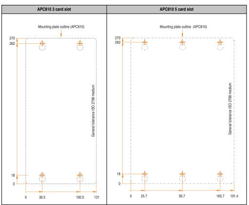
Table 96: Drilling templates - 3 and 5 card slot system units
