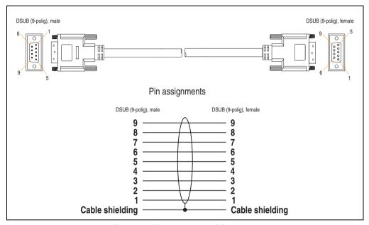
Figure 231: Pin assignments - RS232 cable
