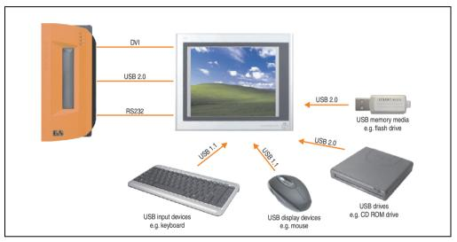
Figure 111: Remote connection of USB peripheral devices to the APC900 via DVI
