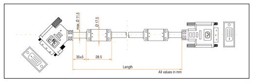
Figure 220: Dimensions - SDL cable with 45° plug 5CASDL.0xxx-01
