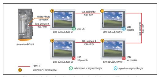
Figure 104: Configuration - Four Automation Panel 900 units via SDL (onboard)
