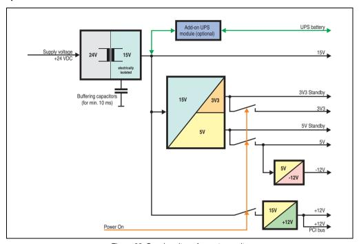
Figure 22: Supply voltage for system units
