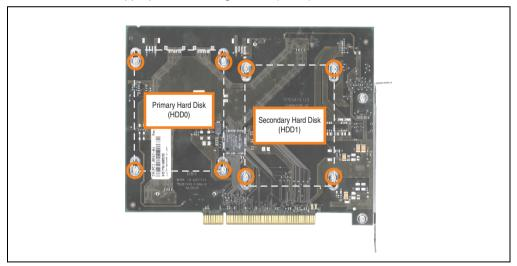
Figure 293: Screw layout on the back side of the SATA RAID controller 5ACPCI.RAIC-03
