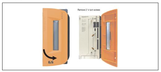
Figure 243: Loosening the 1/4 turn screws
