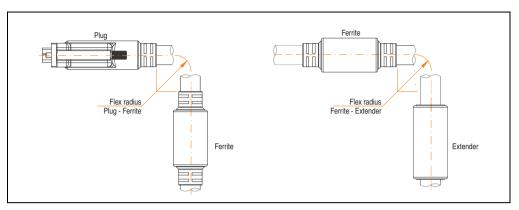
Figure 227: Flex radius specification
