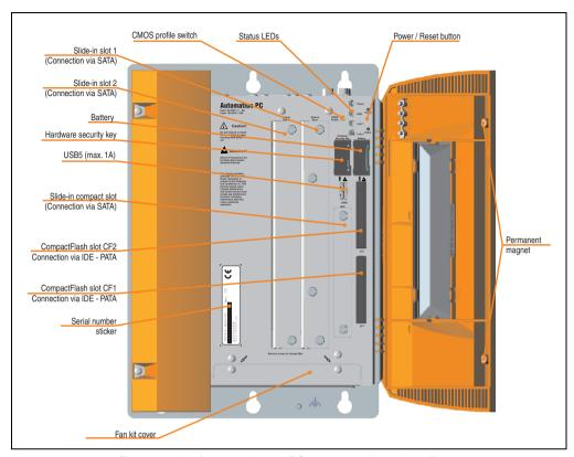
Figure 15: Interface overview - APC810, 5 card slot variant (front)
