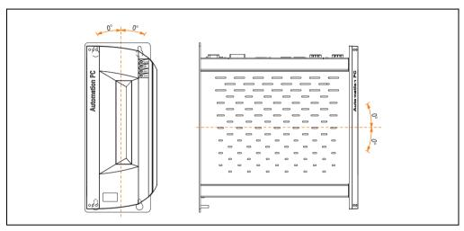
Figure 95: Standard mounting - vertical
