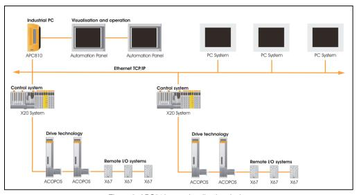
Figure 2: APC810 as a visualization device
