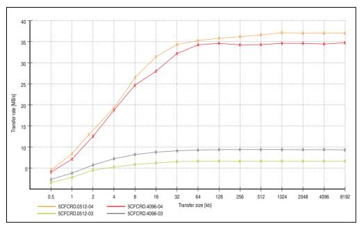
Figure 181: ATTO disk benchmark v2.34 comparison (reading)
