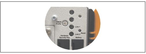
Figure 154: CMOS profile hex switch
