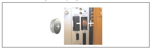
Figure 242: Battery polarity
