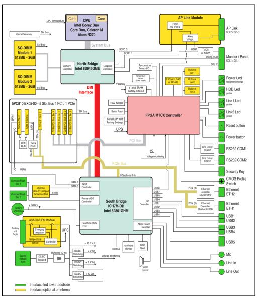
Figure 37: Block diagram 5PC810.SX05-00 + 5PC810.BX05-00
