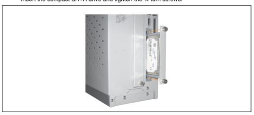
Figure 244: Inserting the compact SATA drive
