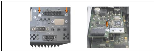
Figure 256: Install UPS module
