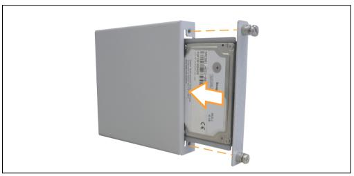
Figure 295: Installing the replacement hard disk in the replacement disk tray
