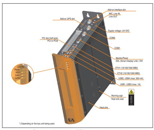
Figure 5: Interface overview - APC810, 1 card slot variant (top)
