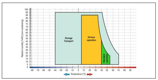
Figure 72: Temperature humidity diagram - SATA RAID hard disk 5ACPCI.RAIC-02
