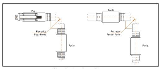
Figure 211: Flex radius specification
