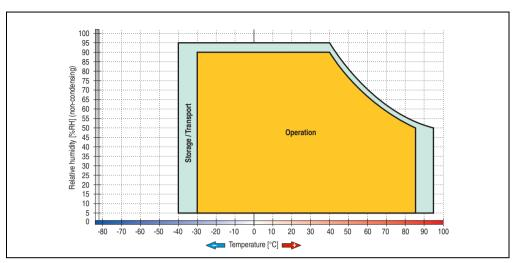
Figure 64: Temperature humidity diagram - 5AC801.HDDS-00
