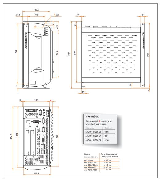
Figure 10: Dimensions - APC810 2 card slot variant
