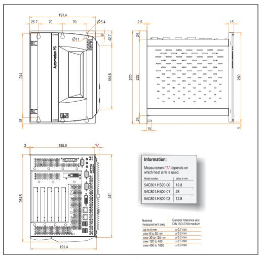
Figure 16: Dimensions - APC810 5 card slot variant
