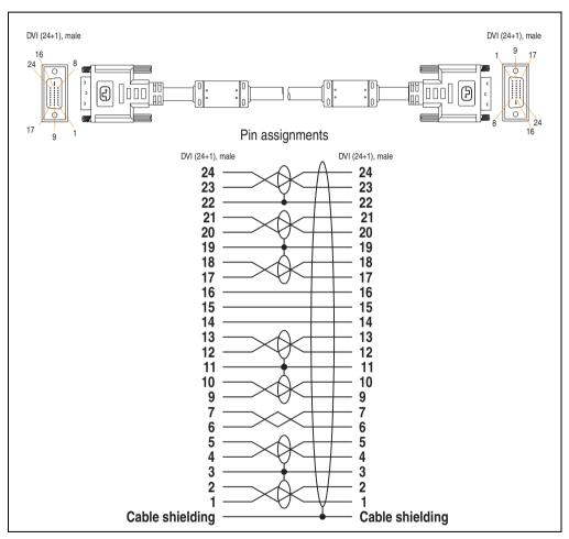
Figure 217: Pin assignments - SDL cable 5CASDL.0xxx-00
