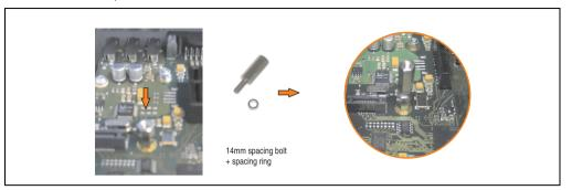
Figure 255: Screw in spacing bolt and spacing ring
