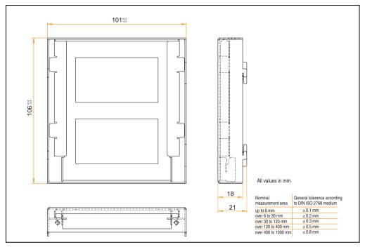
Figure 236: Dimensions - HDD replacement disk tray
