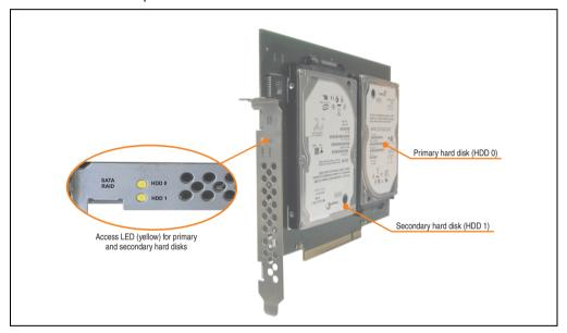
Figure 73: PCI SATA RAID controller - 5ACPCI.RAIC-03
