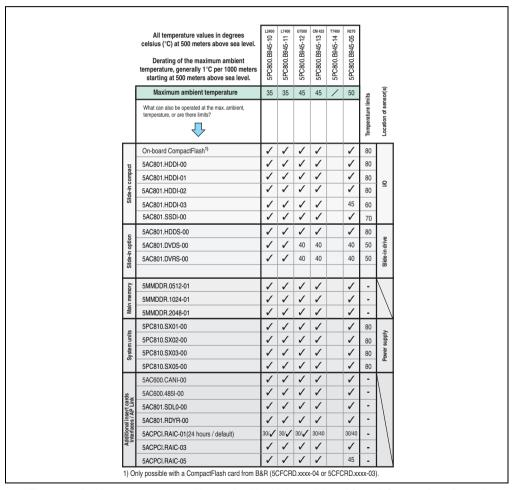
Figure 19: Ambient temperatures without a fan kit with heat sinks 5AC801.HS00-00 Rev. D0 and 5AC801.HS00-01 Rev. D0 and 5AC801.HS00-02
