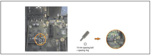
Figure 266: Screw in spacing bolt and spacing ring
