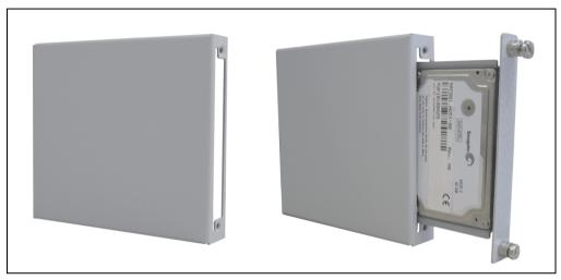
Figure 235: HDD replacement disk tray - 5AC801.FRAM-00
