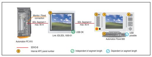
Figure 103: Configuration - One AP900 and an AP800 via SDL (onboard)
