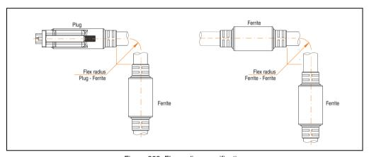
Figure 223: Flex radius specification
