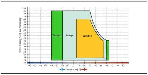
Figure 68: Temperature humidity diagram - Slide-in DVD-R/RW, DVD+R/RW - 5AC801.DVRS-00
