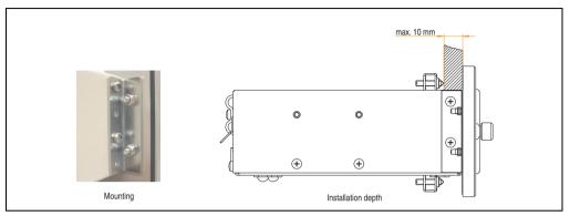
Figure 193: Front cover mounting and installation depth
