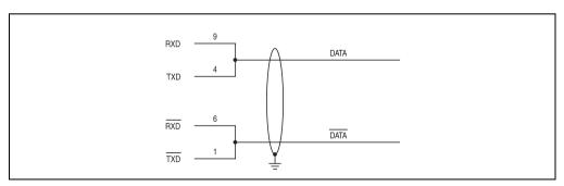
Figure 92: Add-on RS232/422/485 interface - operated in RS485 mode
