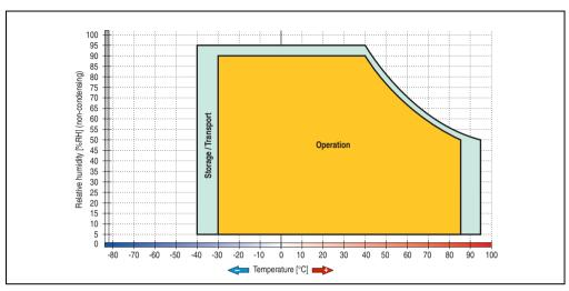
Figure 76: Temperature humidity diagram - SATA RAID hard disk 5ACPCI.RAIC-04
