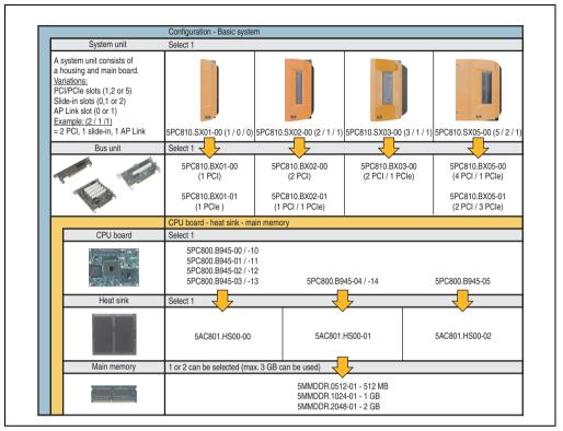
Figure 3: Configuration - Basic system
