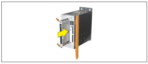
Figure 246: Installing the slide-in drive
