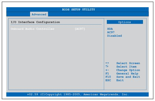
Figure 133: 945GME Advanced I/O Interface Configuration
