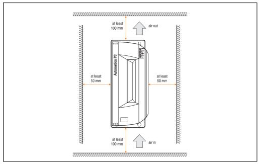
Figure 97: Standard mounting - Mounting distances
