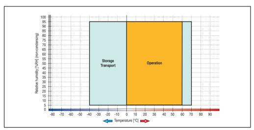
Figure 57: Temperature humidity diagram - 5AC801.HDDI-03
