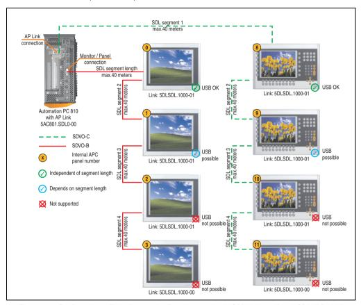
Figure 108: Configuration - Eight Automation Panel 900 units via SDL (onboard) and SDL (AP Link)
