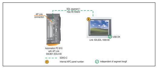
Figure 105: Configuration - One Automation Panel 900 via SDL (AP Link)
