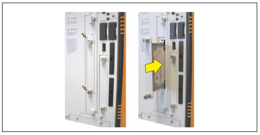
Figure 249: Inserting the slide-in compact drive
