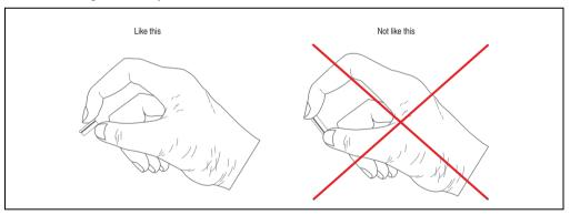
Figure 241: Battery handling
