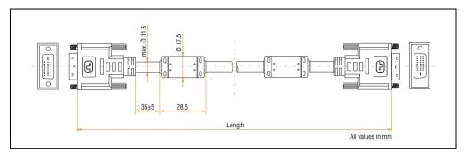
Figure 216: Dimensions - SDL cable 5CASDL.0xxx-00
