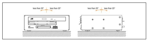
Figure 190: Mounting orientation - 5MD900.USB2-01
