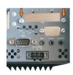
Figure 297: Remove UPS module cover
