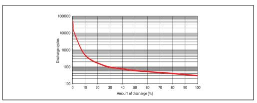
Figure 201: Deep discharge cycles
