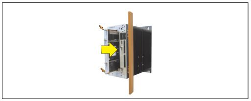
Figure 248: Installing the slide-in compact adapter
