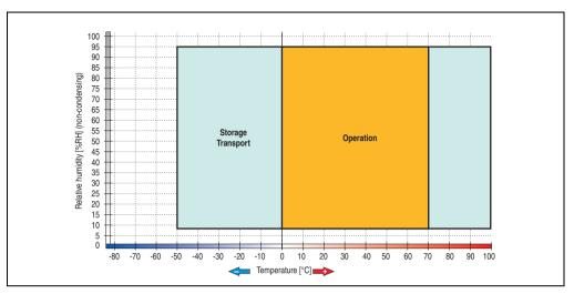
Figure 183: Temperature humidity diagram - CompactFlash cards 5CFCRD.xxxx-03
