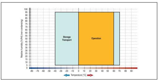
Figure 78: Temperature humidity diagram - SATA RAID Hard Disk - 5ACPCI.RAIC-05
