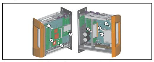
Figure 301: Temperature sensor locations
