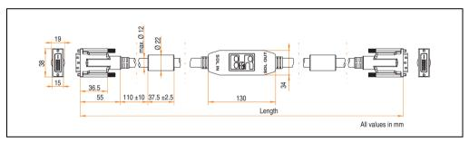
Figure 228: Dimensions - SDL flex cable with extender 5CASDL.0x00-13
