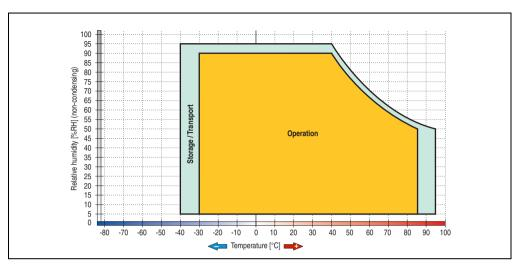
Figure 53: Temperature humidity diagram - 5AC801.HDDI-01
