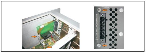
Figure 299: Installing the ready relay
