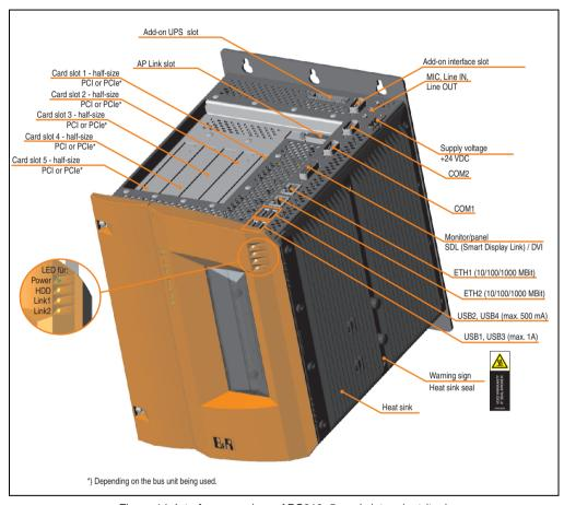
Figure 14: Interface overview - APC810, 5 card slot variant (top)
