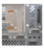
Figure 291: Remove AP Link module cover
