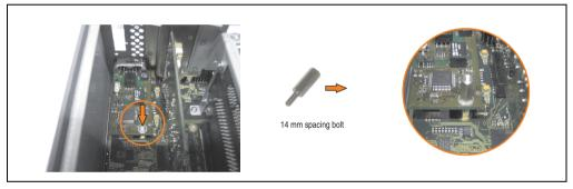
Figure 277: Screw in spacing bolt
