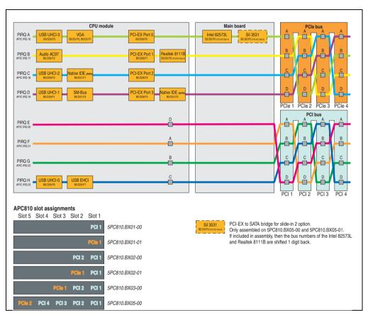
Figure 155: PCI and PCIe routing with activated APIC CPU boards B945GME (COM Express) for BIOS version ≤ 1.12
