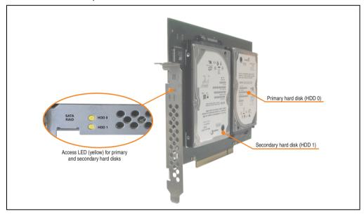
Figure 77: PCI SATA RAID controller - 5ACPCI.RAIC-05
