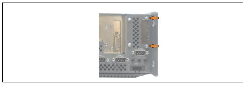
Figure 276: Remove UPS module cover
