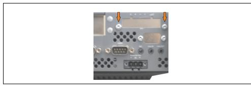
Figure 254: Remove UPS module cover
