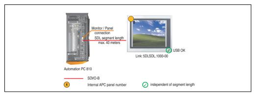
Figure 101: Configuration - An Automation Panel 900 via SDL (onboard)
