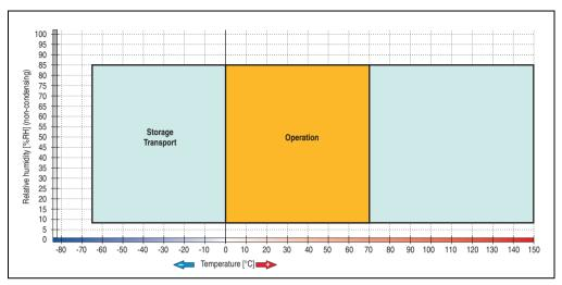
Figure 179: Temperature humidity diagram - CompactFlash cards 5CFCRD.xxxx-04
