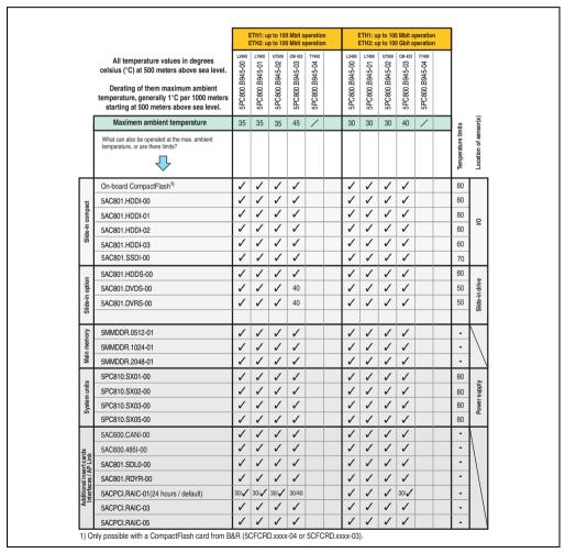
Figure 17: Ambient temperatures without a fan kit with heat sink < Rev. D0
