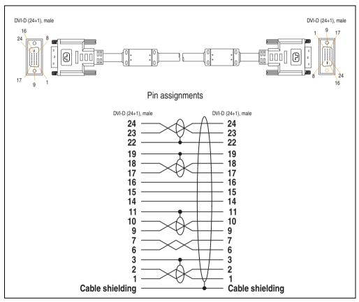
Figure 213: Pin assignments - DVI cable
