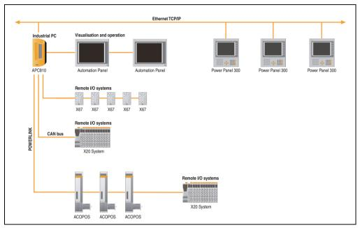
Figure 1: APC810 for central control and visualization
