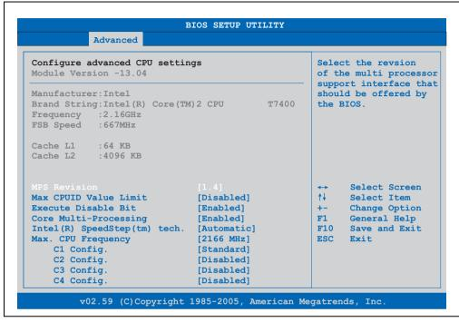
Figure 131: 945GME - Advanced CPU Configuration
