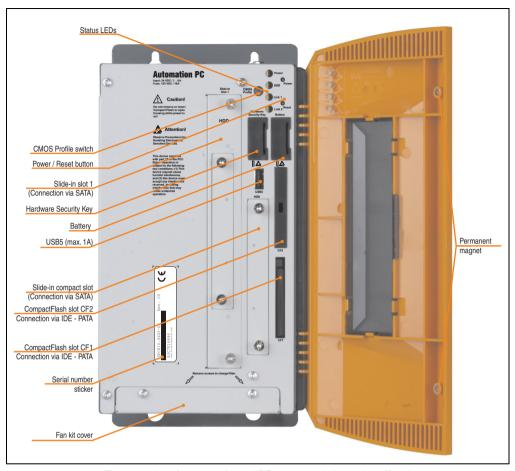
Figure 12: Interface overview - APC810, 3 card slot variant (front)
