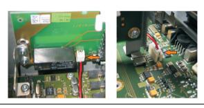
Figure 300: Plug in connection cable
