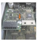
Figure 273: Install UPS module
