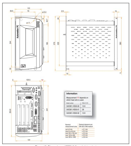
Figure 13: Dimensions - APC810 3 card slot variant
