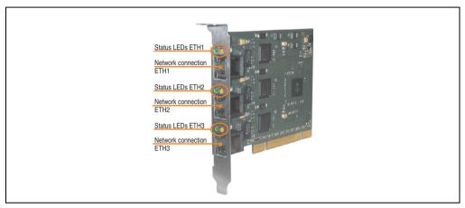
Figure 208: PCI Ethernet card 10/100 - 5ACPCI.ETH3-01
