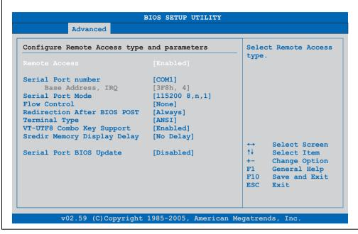
Figure 142: 945GME - Advanced Remote Access Configuration
