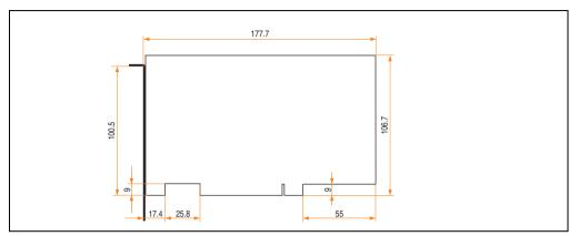
Figure 40: Dimensions - Standard half-size PCI card
