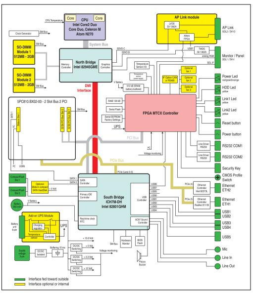
Figure 34: Block diagram 5PC810.SX02-00 + 5PC810.BX02-00
