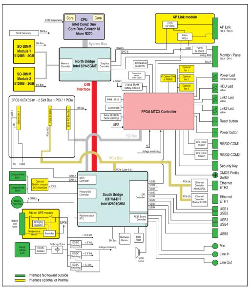
Figure 35: Block diagram 5PC810.SX02-00 + 5PC810.BX02-01
