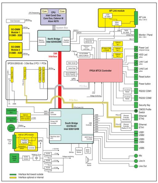
Figure 36: Block diagram 5PC810.SX03-00 + 5PC810.BX03-00
