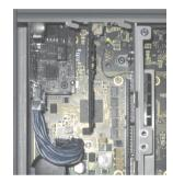
Figure 286: Plug in connection cable
