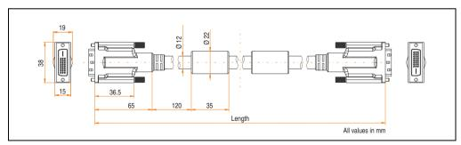
Figure 224: Dimensions - SDL cable 5CASDL.0xxx-03
