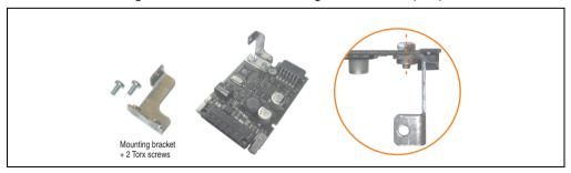
Figure 278: Install mounting bracket
