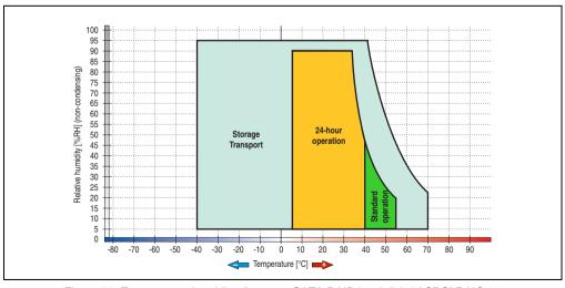
Figure 70: Temperature humidity diagram - SATA RAID hard disk 5ACPCI.RAIC-01
