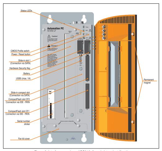
Figure 9: Interface overview - APC810, 2 card slot variant (front)
