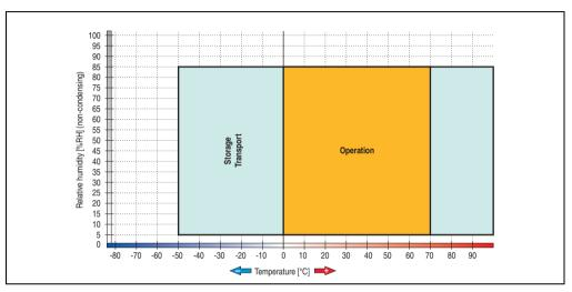
Figure 195: Temperature humidity diagram - USB flash drive - 5MMUSB.2048-01
