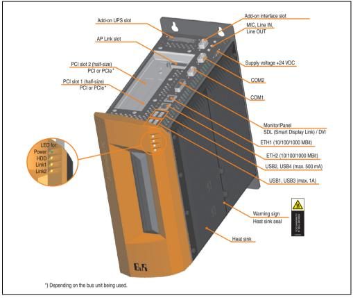
Figure 8: Interface overview - APC810, 2 card slot variant (top)
