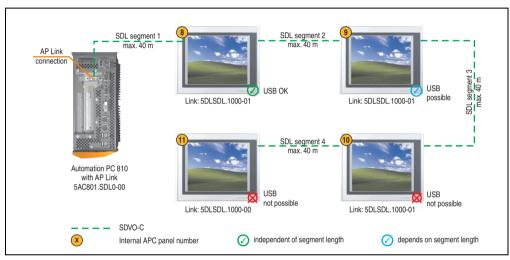
Figure 106: Configuration - Four Automation Panel 900 units via SDL (AP Link)
