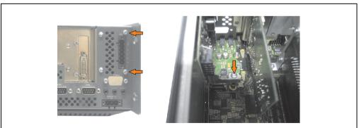
Figure 262: Install UPS module
