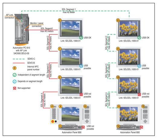
Figure 109: Configuration - Six AP900 and two AP800 devices via SDL (onboard) and SDL (AP Link)
