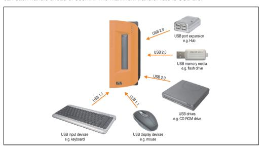
Figure 110: Local connection of USB peripheral devices on the APC810
