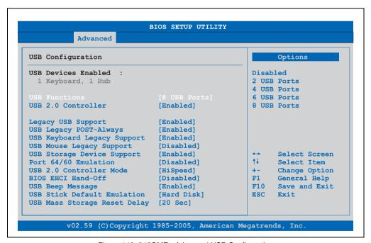
Figure 140: 945GME - Advanced USB Configuration
