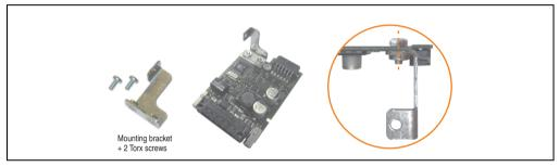
Figure 261: Install mounting bracket
