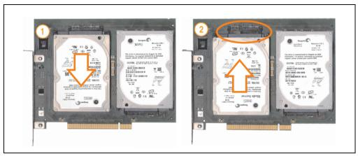
Figure 294: Hard disk exchange
