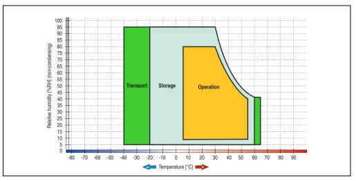
Figure 66: Temperature humidity diagram - Slide-in DVD-ROM/CD-RW - 5AC801.DVDS-00
