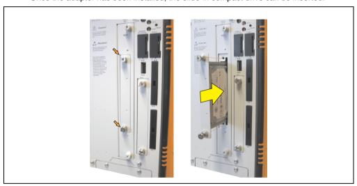
Figure 241: Inserting the slide-in compact drive
