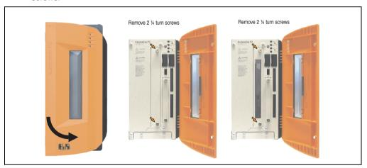
Figure 239: Loosening the 1/4 turn screws
