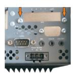
Figure 263: Remove UPS module cover
