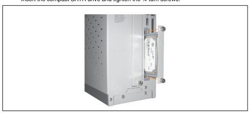
Figure 236: Inserting the compact SATA drive
