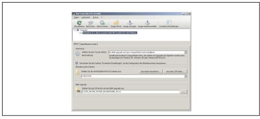
Figure 159: Creating a CompactFlash card for B&R upgrade files
