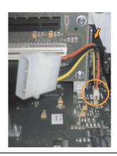
Figure 291: Connector location for external devices
