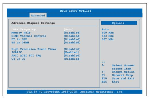
Figure 126: 945GME Advanced Chipset Configuration
