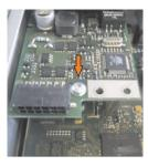
Figure 265: Install UPS module
