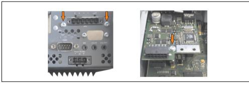
Figure 248: Install UPS module
