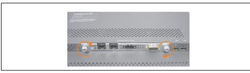
Figure 57: Fasten the PPC300 in the AP900
