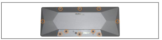
Figure 127: Remove screws
