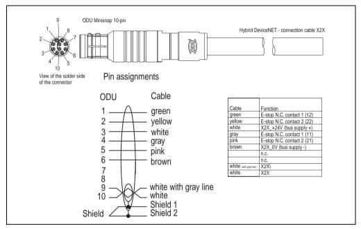
Figure 87: Pin assignments, X2X cable 5CAX2X.0xxx-20
