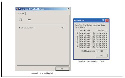
Figure 102: Example - Hardware number in the B&R Key Editor or in the B&R Control Center
