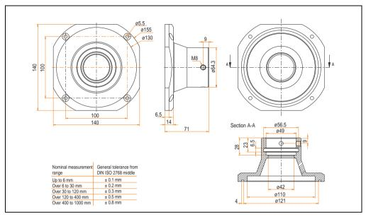
Figure 69: Dimensions - extension flange 5AC800.FLG1-00
