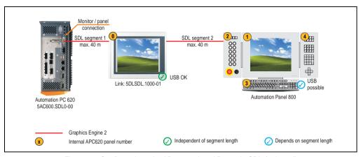
Figure 98: Configuration - An AP900 and an AP800 via SDL (onboard)
