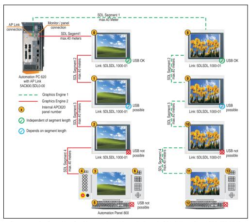
Figure 100: Configuration - Six AP900 and two AP800 devices via SDL (onboard) and SDL (AP Link)
