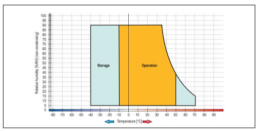
Figure 125: Temperature humidity diagram - Elo Accu touch screen 5-wire
