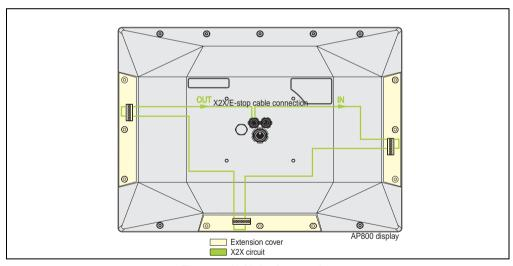
Figure 88: X2X circuit - rear view
