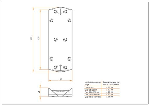
Figure 65: Dimensions - extension connector 5AC800.CON1-00
