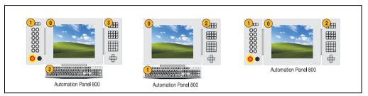
Figure 101: Examples - internal numbering of the extension units
