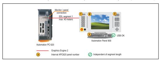
Figure 97: Configuration - An Automation Panel 800 via SDL (onboard)
