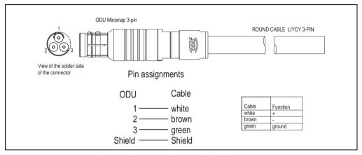
Figure 84: Pin assignments - voltage supply cable 5CAPWR.0xxx-20
