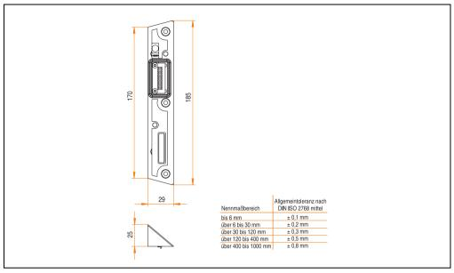
Figure 61: Dimensions - extension cover 5AC800.COV1-00
