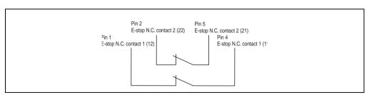
Figure 23: E-stop circuit connections
