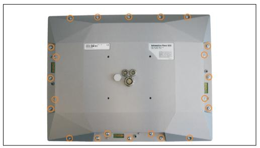
Figure 116: Remove screws
