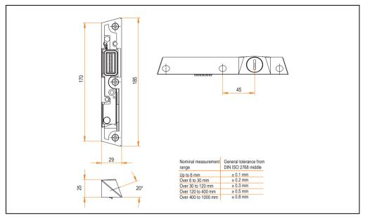
Figure 63: Dimensions - USB extension cover 5AC800.COV2-00
