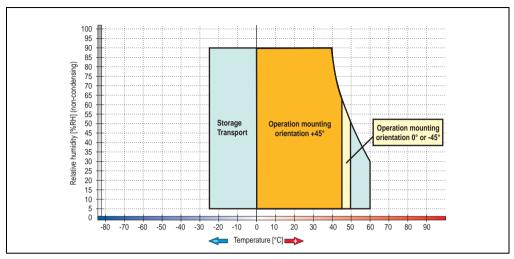
Figure 20: Temperature humidity diagram - 5AP880.1505-00
