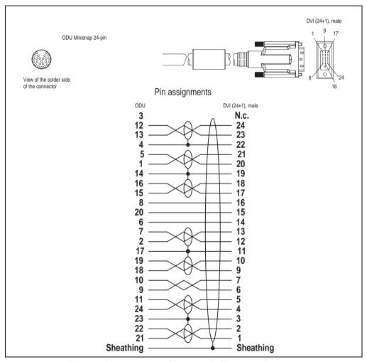
Figure 72: Pin assignments - SDL cable 5CASDL.0xxx-20 Rev. < A5
