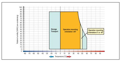
Figure 16: Temperature humidity diagram - 5AP820.1505-00
