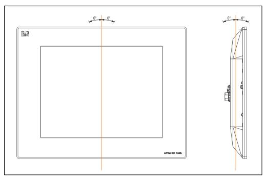
Figure 95: Mounting orientation 0°
