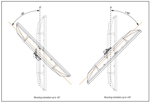
Figure 96: Mounting orientation -45° and +45°.
