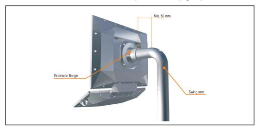
Figure 93: Swing arm system mounting
