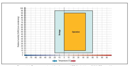
Figure 114: Temperature humidity diagram - USB flash drive - 5MMUSB.xxxx-00
