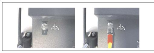
Figure 107: Functional grounding clip
