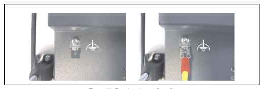
Figure 75: Functional grounding clip
