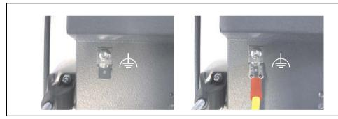
Figure 27: Functional grounding clip
