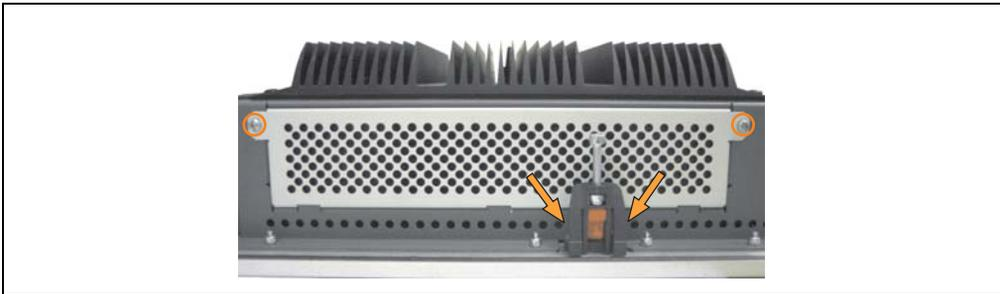
Figure 373: Removing the fan kit cover
