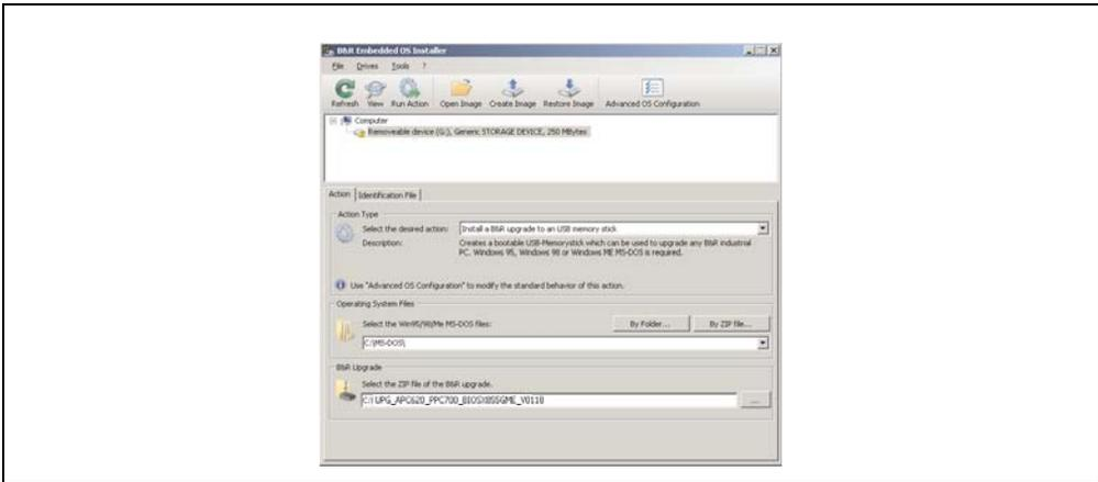
Figure 284: Creating a USB flash drive for B&R upgrade files
