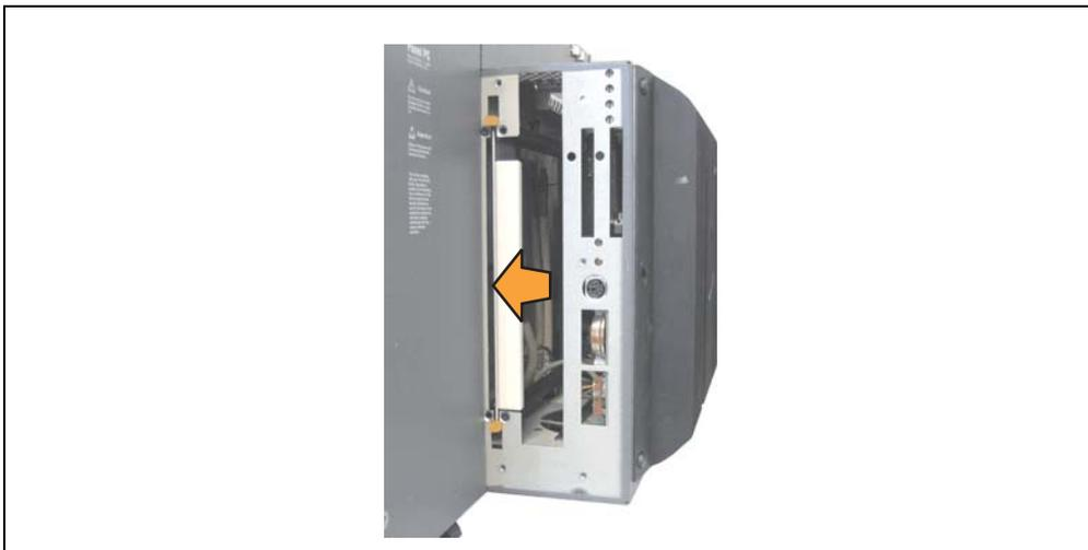
Figure 384: Removing the slide-in dummy module
