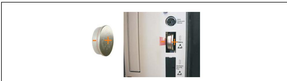
Figure 371: Battery polarity
