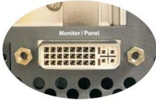
Figure 31: Monitor / Panel connection
