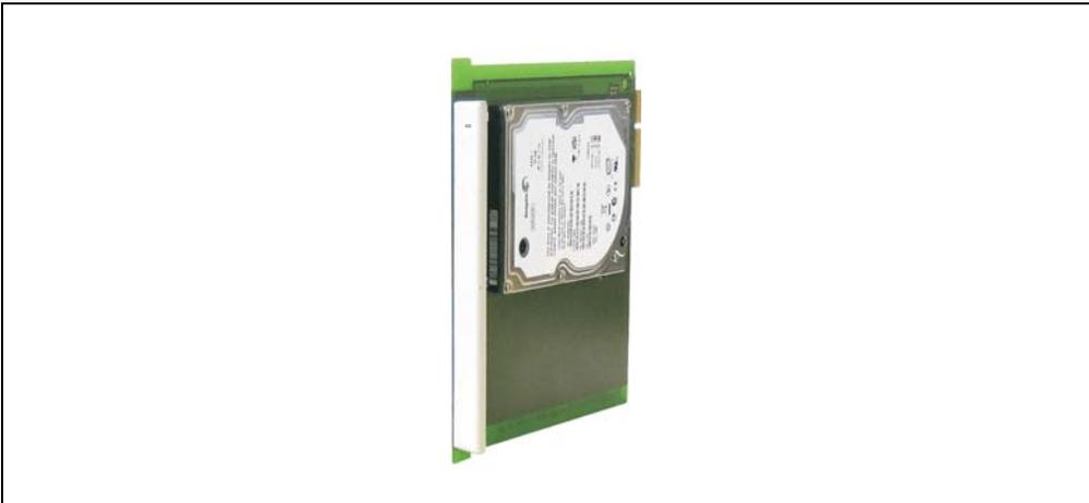
Figure 126: Slide-in hard disk 40 GB - 5AC600.HDDS-02
