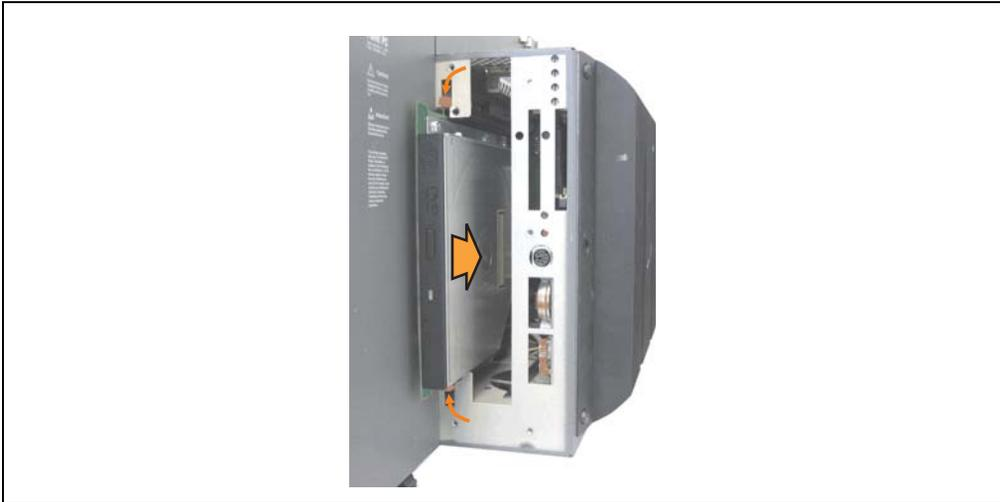
Figure 388: Installing the slide-in drive
