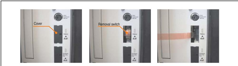
Figure 369: Battery removal
