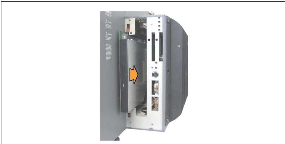
Figure 385: Installing the slide-in drive
