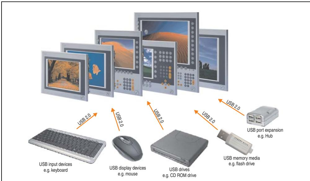
Figure 163: Local connection of USB peripheral devices on the PPC 700
