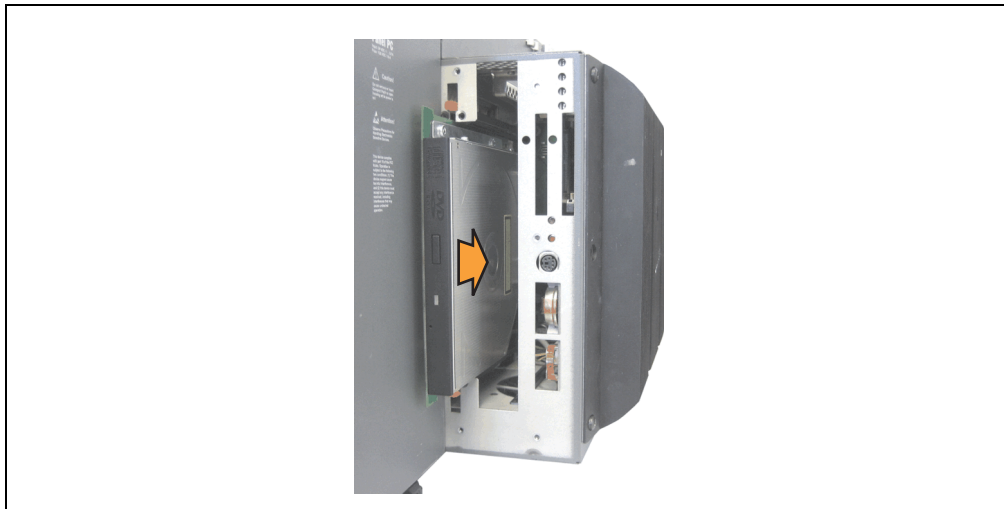
Figure 370: Installing the slide-in drive
