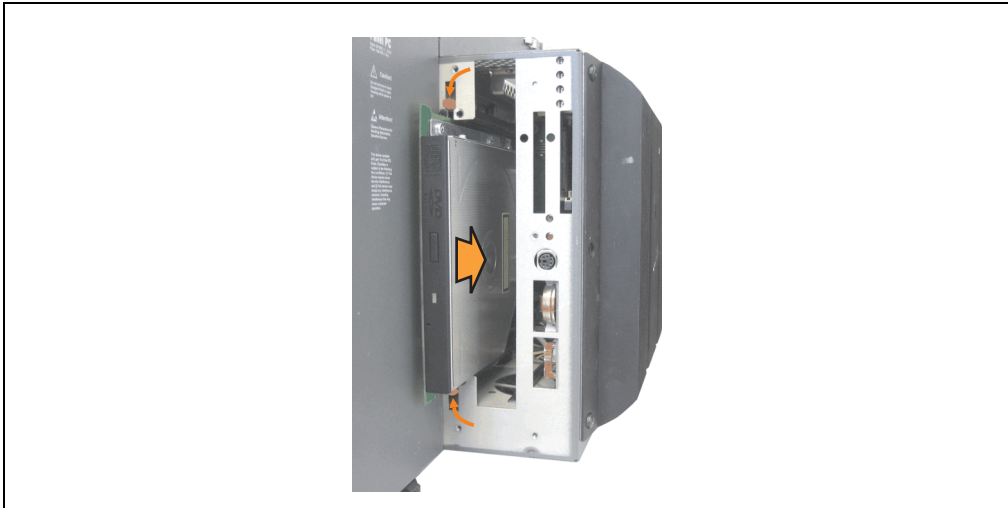
Figure 373: Installing the slide-in drive
