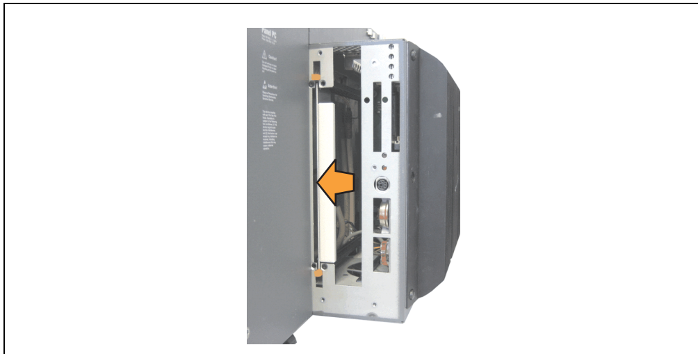
Figure 369: Removing the slide-in dummy module
