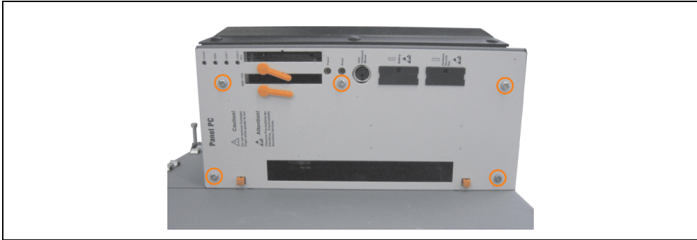
Figure 366: Removing the side cover
