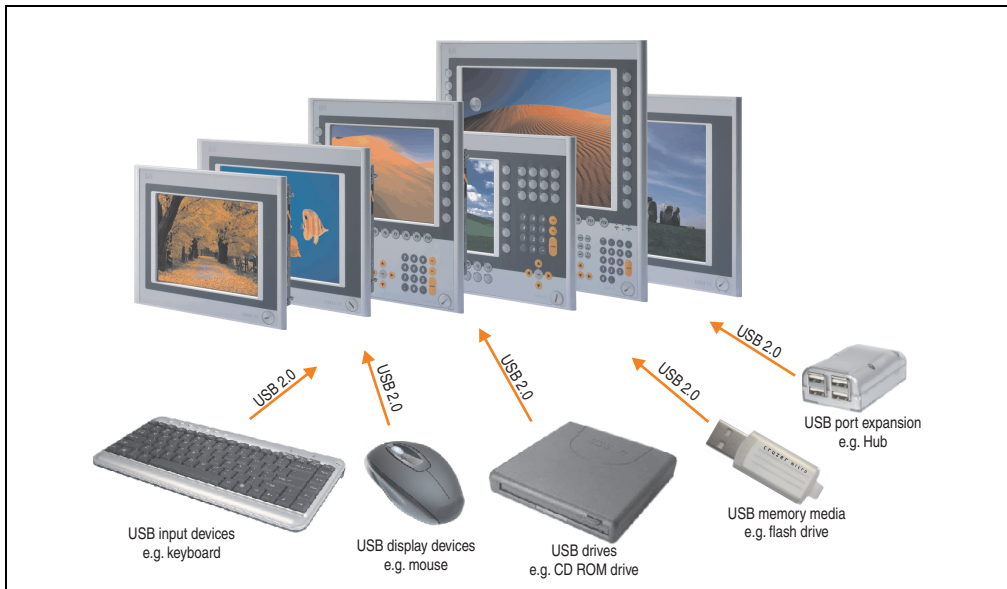
Figure 155: Local connection of USB peripheral devices on the PPC 700
