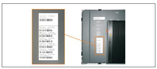
Figure 35: Serial number stickers for individual PPC700 components
