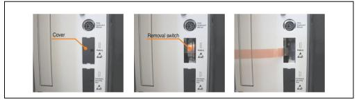
Figure 344: Battery removal
