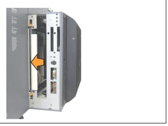
Figure 358: Removing the slide-in dummy module
