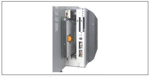
Figure 359: Installing the slide-in drive
