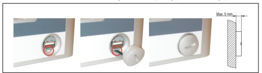
Figure 274: Front side USB interface cover - installation
