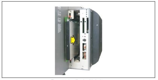
Figure 269: Installing the slide-in drive
