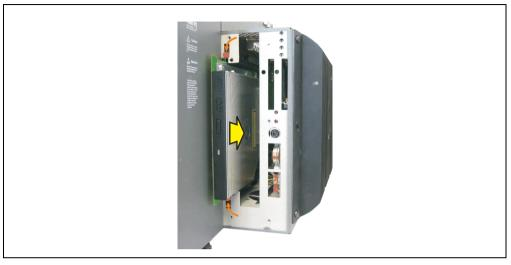
Figure 272: Installing the slide-in drive
