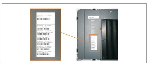
Figure 29: Serial number stickers for individual PPC700 components
