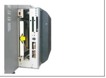
Figure 268: Removing the slide-in dummy module
