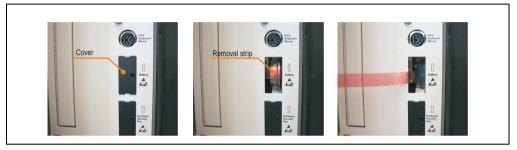
Figure 254: Battery removal
