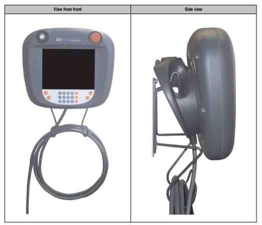
Table 33: Storing a Mobile Panel device on a wall mount
