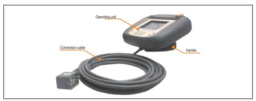
Figure 39: Attachment cable and handle
