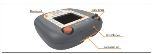
Figure 7: Mobile Panel operating unit
