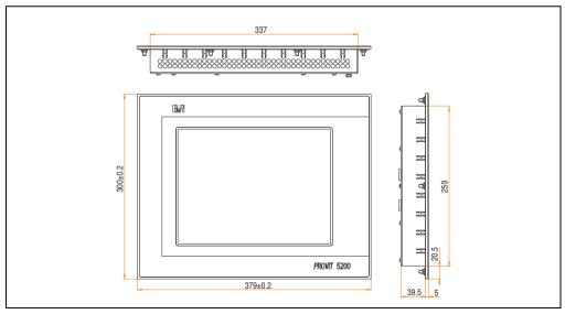
Figure 132: Dimensions - 5D5211.03 starting with Revision J0
