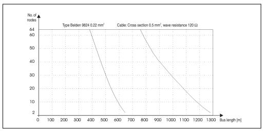
Figure 67: CAN - number of nodes / bus length
