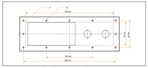
Figure 8: Front plate for external floppy disk drive
