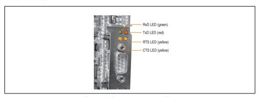
Figure 2: RS232 interface board LEDs
