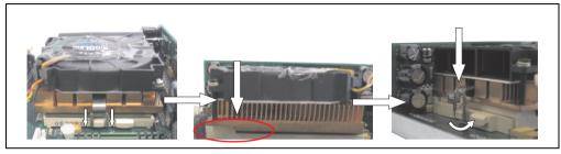
Figure 77: Attaching the new heat sink
