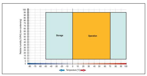
Figure 95: Temperature humidity diagram - CompactFlash cards 5CFCRD.xxxx-03
