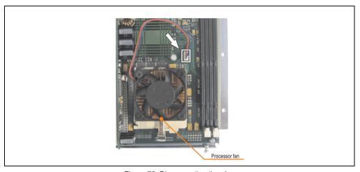
Figure 73: Disconnecting the plug
