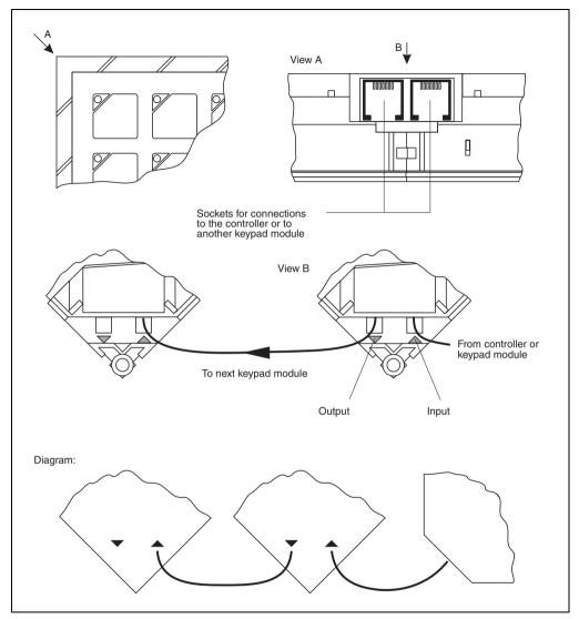
Figure 190: Connection to the controller or other keypad modules.
