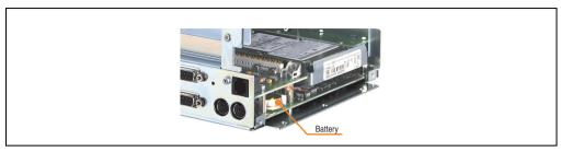
Figure 64: Battery compartment
