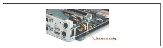
Figure 73: Hardware security key
