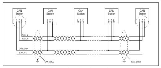
Figure 103: Bus cable - station connection
