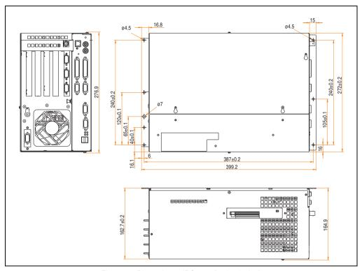
Figure 14: Dimensions - IPC5600 (5-slot design)
