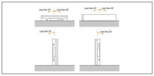
Figure 37: Mounting guidelines - 5A5600.03
