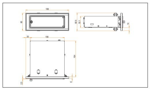
Figure 21: Dimensions - 5A5003.08 with 5A5003.03
