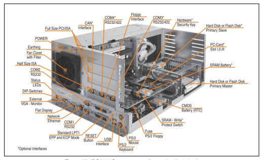
Figure 27: IPC5600C components (bus unit with 4 slots)
