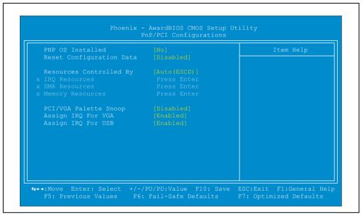
Figure 222: PnP/PCI configurations setup
