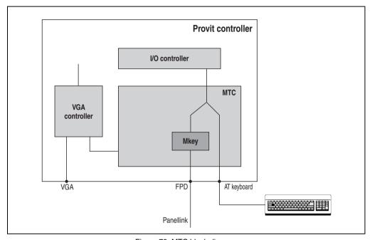
Figure 78: MTC block diagram
