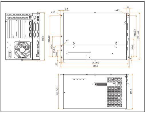
Figure 16: Dimensions - IPC5600 (6-slot design)
