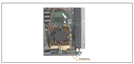
Figure 79: Removing the screws and plug
