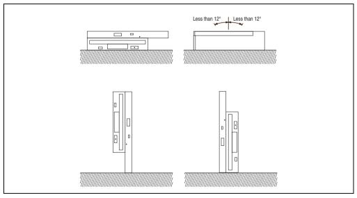
Figure 39: Mounting guidelines - 5A5600.04
