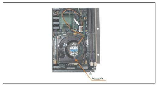
Figure 78: Connecting the plug
