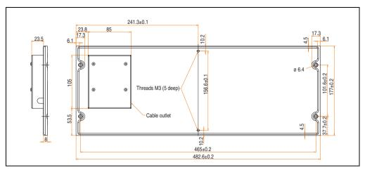
Figure 42: Installation dimensions 19" AT keyboard (figure overleaf)
