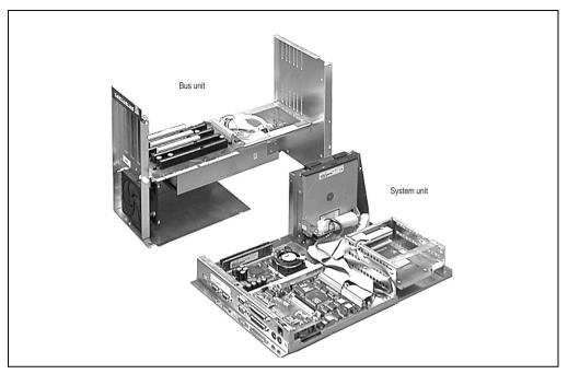
Figure 51: Detaching the bus unit
