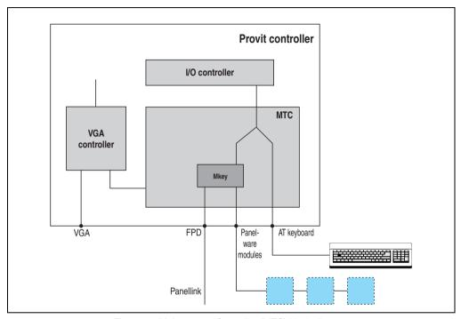
Figure 67: Maintenance Controller (MTC) block diagram
