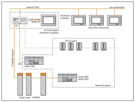
Figure 1: Industrial PC as central controller and visualization
