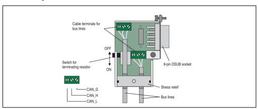
Figure 105: CAN bus connector 7AC911.9
