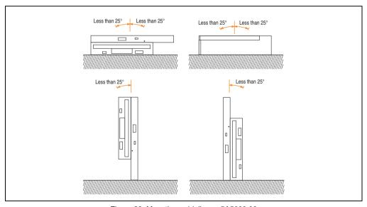
Figure 33: Mounting guidelines - 5A5600.02
