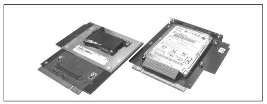
Figure 92: Hard disk - models 5A5001.13, 5A5001.16, 5A5001.18, 5A5001.20
