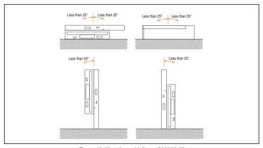
Figure 43: Mounting guidelines - 5A5600.07
