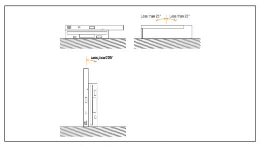
Figure 41: Mounting guidelines - 5A5600.05
