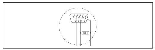
Figure 104: Terminating resistor connections for 9-pin DSUB plug
