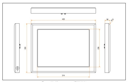
Figure 151: Measurements 5D5212.04
