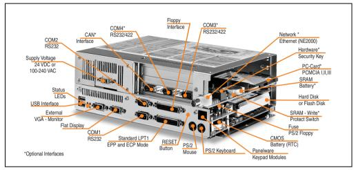
Figure 19: IPC5000 components (bus unit with 2 slots)
