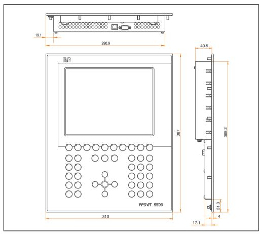
Figure 167: Dimensions - 5D5510 starting with Revision F0
