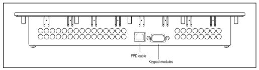
Figure 113: Connections 5D5100.01 and 5D5100.04
