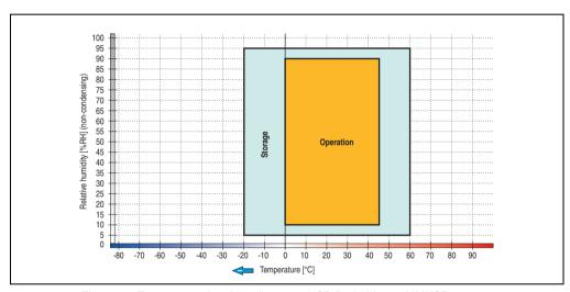
Figure 45: Temperature humidity diagram - USB flash drive - 5MMUSB.xxxx-00
