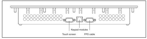
Figure 128: Connections - 5D5211.02 Revision >= F0
