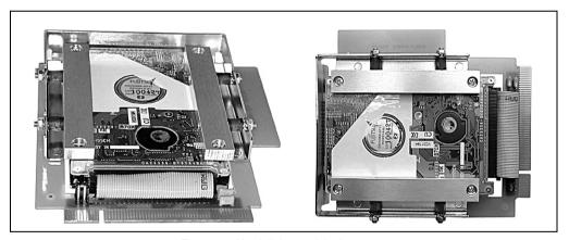
Figure 90: Hard disk - model 5A5001.05
