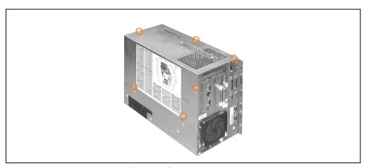
Figure 49: Opening the housing
