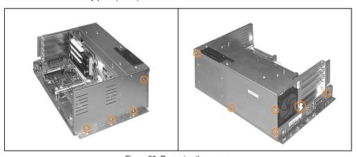
Figure 50: Removing the screws
