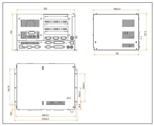
Figure 8: Dimensions - IPC5000 (4-slot design)
