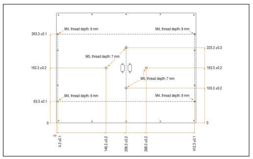
Figure 153: Flange drill holes - 5D5212.04 starting with Revision J0
