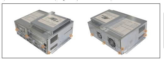
Figure 69: Removing the screws
