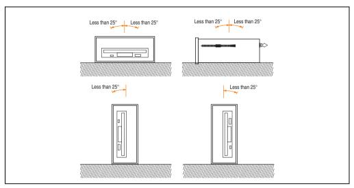
Figure 9: Mounting guidelines - external 3.5" FDD
