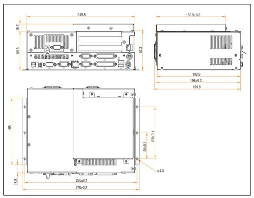
Figure 7: Dimensions - IPC5000C (2 slot design + add-on drive 5A5009.0x)
