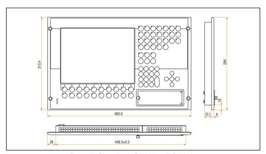
Figure 173: Dimensions - 5D5600.0x and 5D5601.0x
