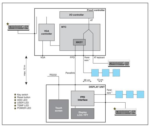
Figure 109: Block diagram for controller, display and peripherals
