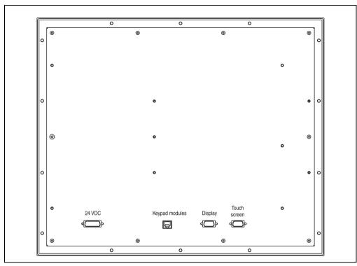
Figure 160: Connections - 5D5213.01 Revision < F0
