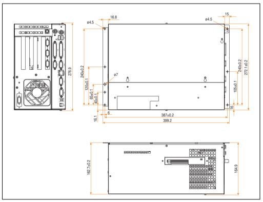
Figure 13: Dimensions - IPC5600C (4-slot design)
