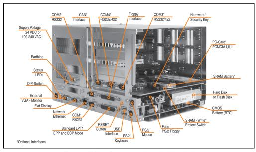
Figure 25: IPC5000C components (bus unit with 4 slots)
