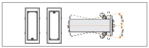
Figure 17: Mounting guidelines - controller R-IDE CD-ROM/LS120 drive (horizontal / vertical)
