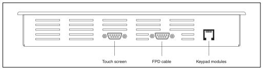
Figure 127: Connections 5D5201.02 and 5D5211.02
