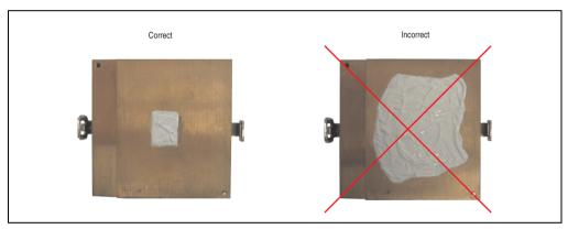
Figure 76: Applying heat conductive paste
