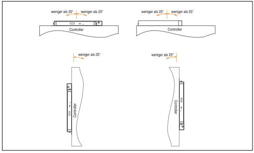
Figure 29: Mounting instructions - add-on CD ROM with controller
