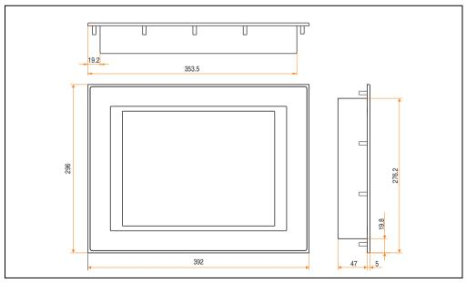
Figure 120: Measurements 5D5200.04
