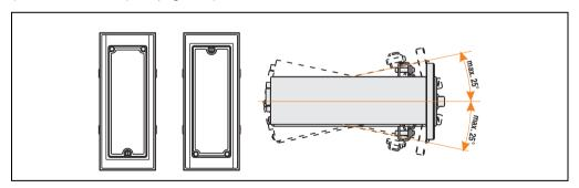
Figure 13: Mounting guidelines - controller R-IDE CD-ROM/LS120 drive (horizontal / vertical)
