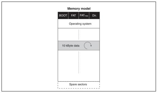
Figure 98: Ring buffer example
