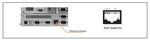
Figure 81: Ethernet connection
