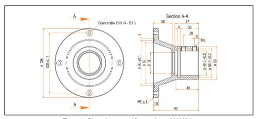
Figure 44: Dimensions - panel flange adapter 5A5007.01
