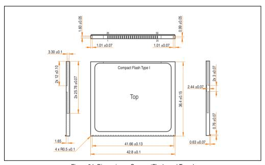
Figure 94: Dimensions - CompactFlash card Type I
