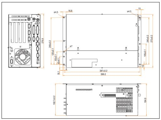
Figure 15: Dimensions - IPC5600C (5-slot design)
