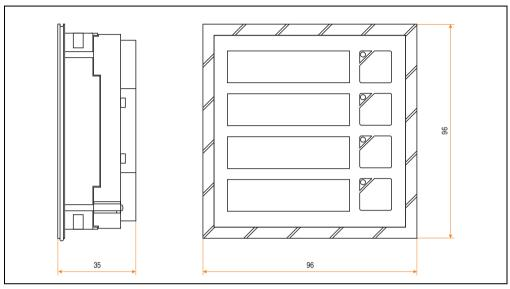
Figure 194: Dimensions - keypad module with 4 keys
