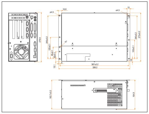
Figure 12: Dimensions - IPC5600 (4-slot design)
