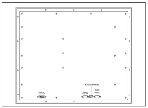
Figure 159: Connections - 5D5213.01 Revision >= F0
