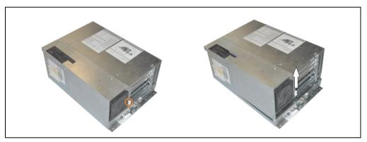
Figure 72: Unlocking the safety pins and removing the bus unit
