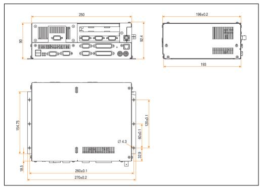
Figure 4: Dimensions - IPC5000 (2-slot design)
