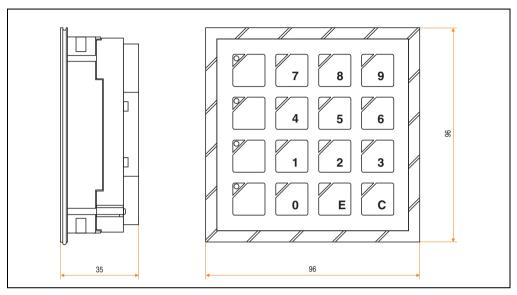
Figure 192: Dimensions - keypad module with 12+4 Keys
