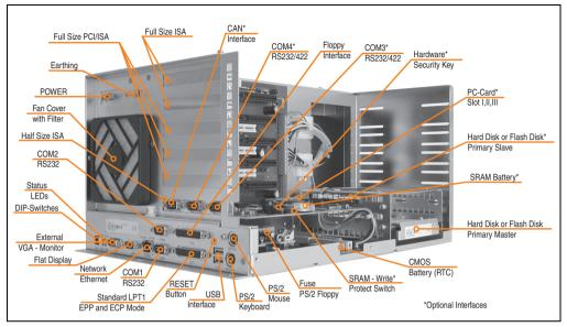
Figure 29: IPC5600C components (bus unit with 6 slots)
