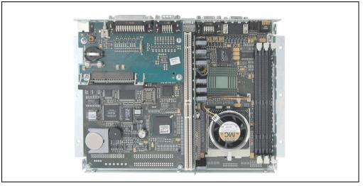
Figure 70: Mainboard system units with socket 370
