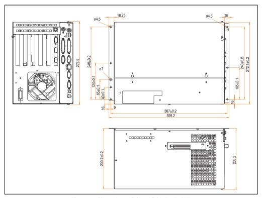
Figure 17: Dimensions - IPC5600C (6-slot design)
