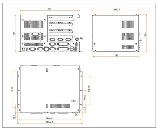
Figure 9: Dimensions - IPC5000C (4-slot design)
