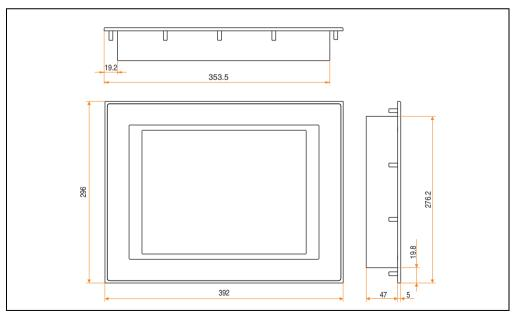
Figure 141: Measurements 5D5202.01, 5D5202.03 and 5D5212.01
