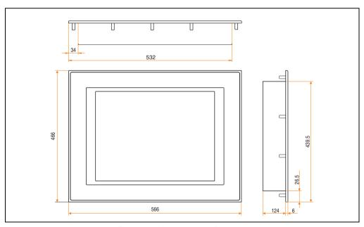
Figure 162: Measurements 5D9200.01
