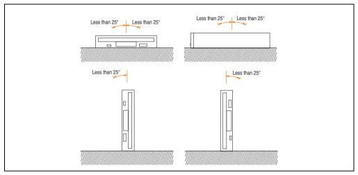
Figure 31: Mounting guidelines - 5A5600.01
