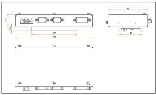
Figure 39: Dimensions - GS link remote unit 5A5010.02
