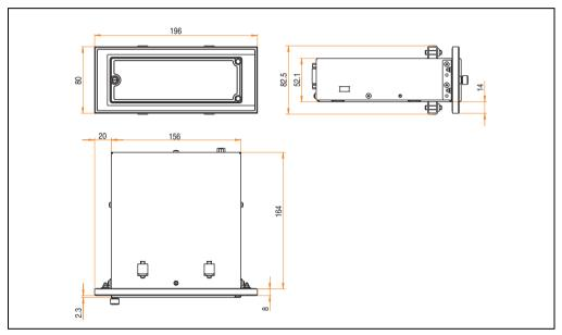
Figure 16: Dimensions - 5A5003.07 with front cover 5A5003.03
