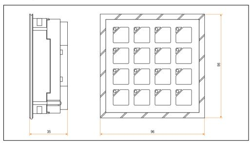
Figure 189: Dimensions for standard keypad modules
