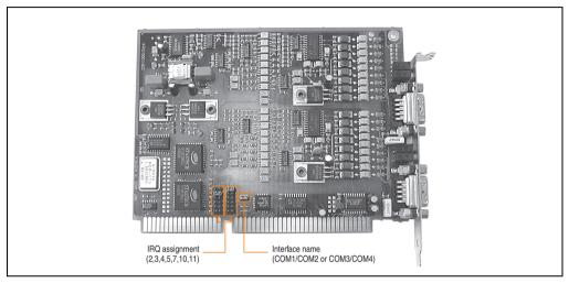
Figure 3: Jumper position
