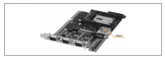
5) Remove the battery from the holder by pulling the removal strip (do not use uninsulated tools -> risk of short circuiting). The battery should not be held by its edges. **Insulated** tweezers may also be used for removing the battery.
