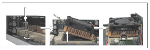
Figure 75: Removing the heat sink
