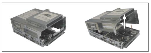
Figure 70: Removing the cover and bus unit
