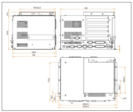
Figure 11: Dimensions - IPC5000C (5-slot design + add-on drive 5A5009.0x)
