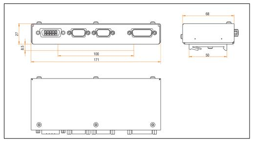
Figure 36: Remote display adapter - local unit 5A5010.01 - dimensions
