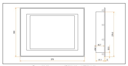
Figure 130: Measurements 5D5201.03 and 5D5211.03
