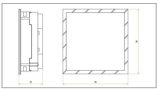
Figure 195: Dimensions - dummy module
