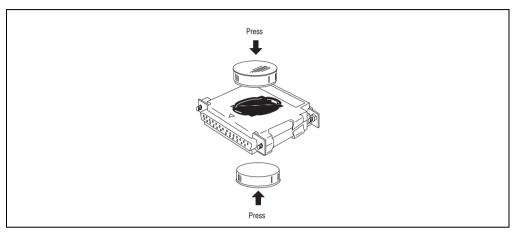
Figure 40: Hardware security key parallel adapter
