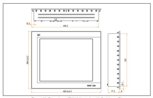
Figure 156: Dimensions - 5D5213.01 starting with Revision >= F0
