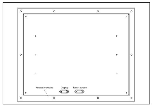
Figure 134: Connections - 5D5201.03 and 5D5211.03
