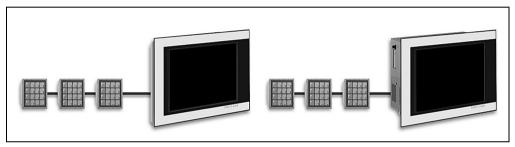
Figure 108: Connection of Panelware modules
