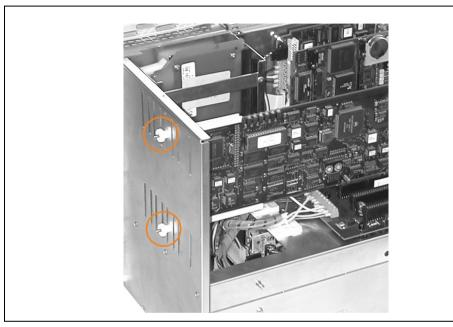
Figure 84: Fasteners for full-size cards
