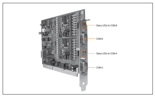
Figure 1: RS232 interface board
