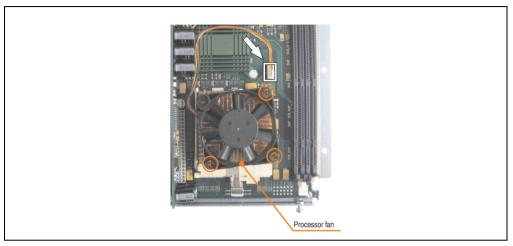
Figure 80: Fastening the fan and connecting the plug
