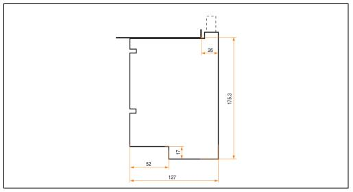
Figure 101: Dimensions - interface board
