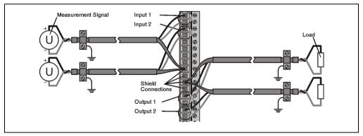
Figure 145: AM050 signal cable connection
