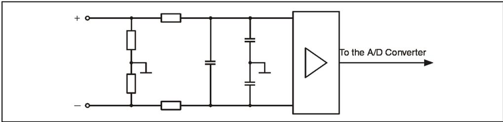
Figure 155: AM055 input circuit diagram
