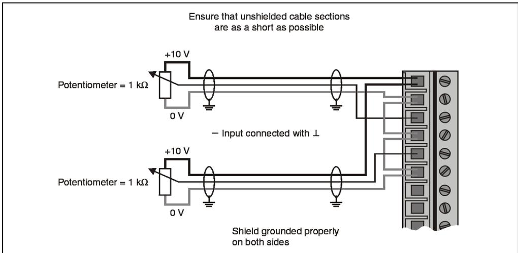
Figure 154: AM055 potentiometer operation
