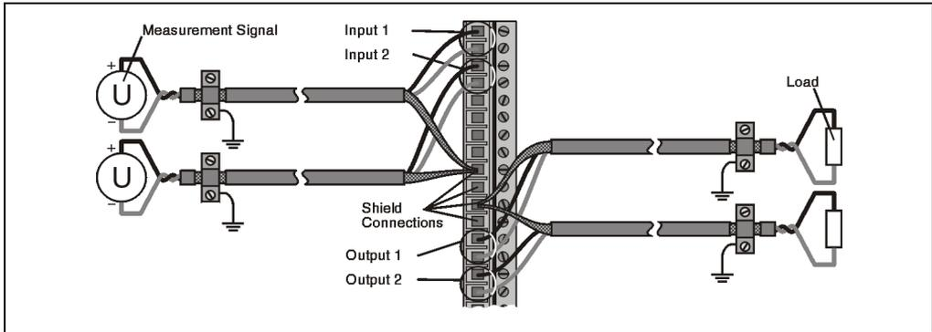
Figure 153: AM055 signal cable connection
