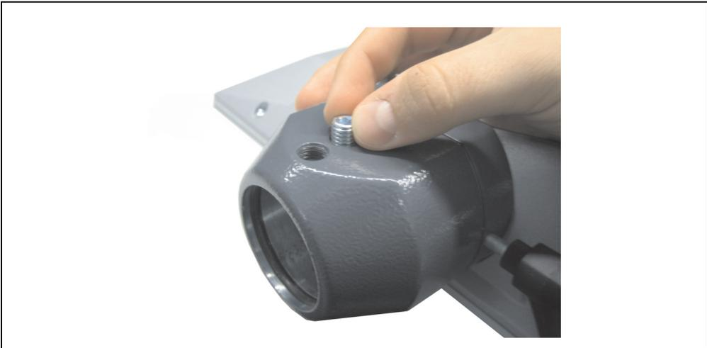
Figure 25: Mounting the screws on the flange
