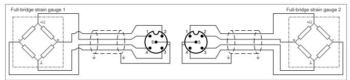
When connecting 3 or more full-bridge strain gauges in parallel, 2 lines must be consolidated in one connector.
