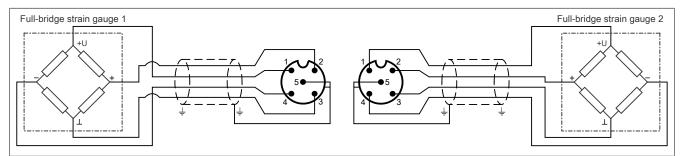
When connecting 3 or more full-bridge strain gauges in parallel, 2 lines must be consolidated in one connector.
