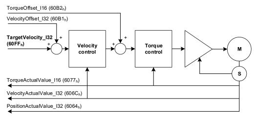
Figure 24: Cyclic synchronous velocity mode overview
