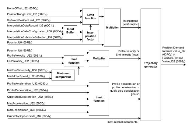
Figure 19: Interpolation controller
