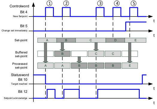
Figure 13: Set-point handling for two set-points
