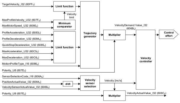
Figure 17: Profile velocity mode
