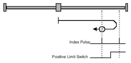
Figure 30: Homing on the positive limit switch and index pulse
