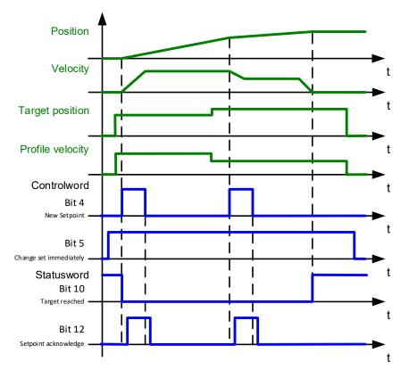
Figure 11: Handshaking procedure for the single set-point method
