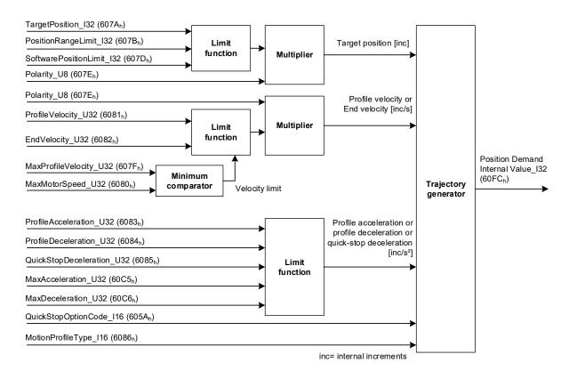
Figure 9: Trajectory generator for profile position mode
