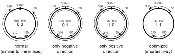
Figure 39: Rotary axis positioning
