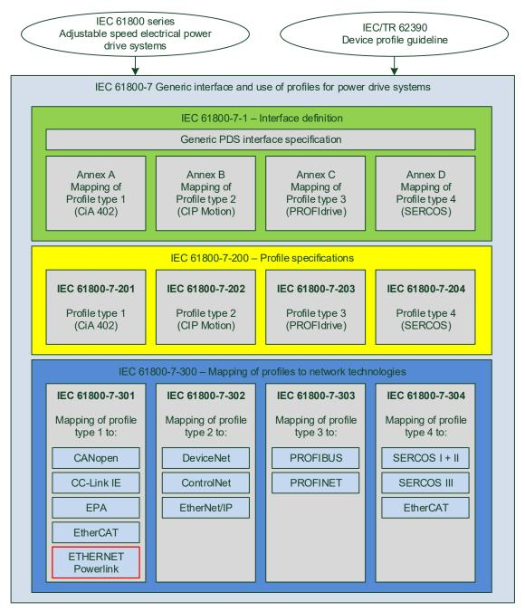
Figure 1: Structure of the IEC 61800-7
