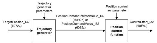
Figure 8: Trajectory generator and position control function
