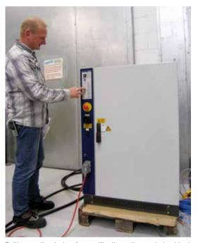
Built according to b+m's specifications, the control cabinet takes up less space and is faster to install and wire thanks to the B&R solution. The reduced number of moving parts and the use of cold plate cooling extended the service life of the system.
