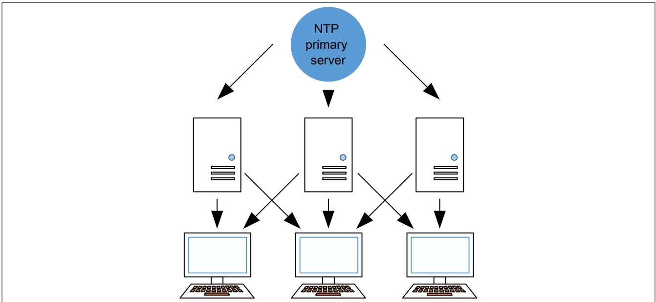
NTP is not suitable for industrial real-time Ethernet with accuracy requirements in the microsecond and sub-microsecond range, however, so most technologies use their own mechanisms for time synchronization. POWER-LINK, for example, uses the first frame in the cycle (SoC) that is sent by the master at highly precise, equidistant times to synchronize the stations. In other technologies (e.g. PROFINET, CIP Sync with EtherNet/IP), IEEE 1588 is used.
