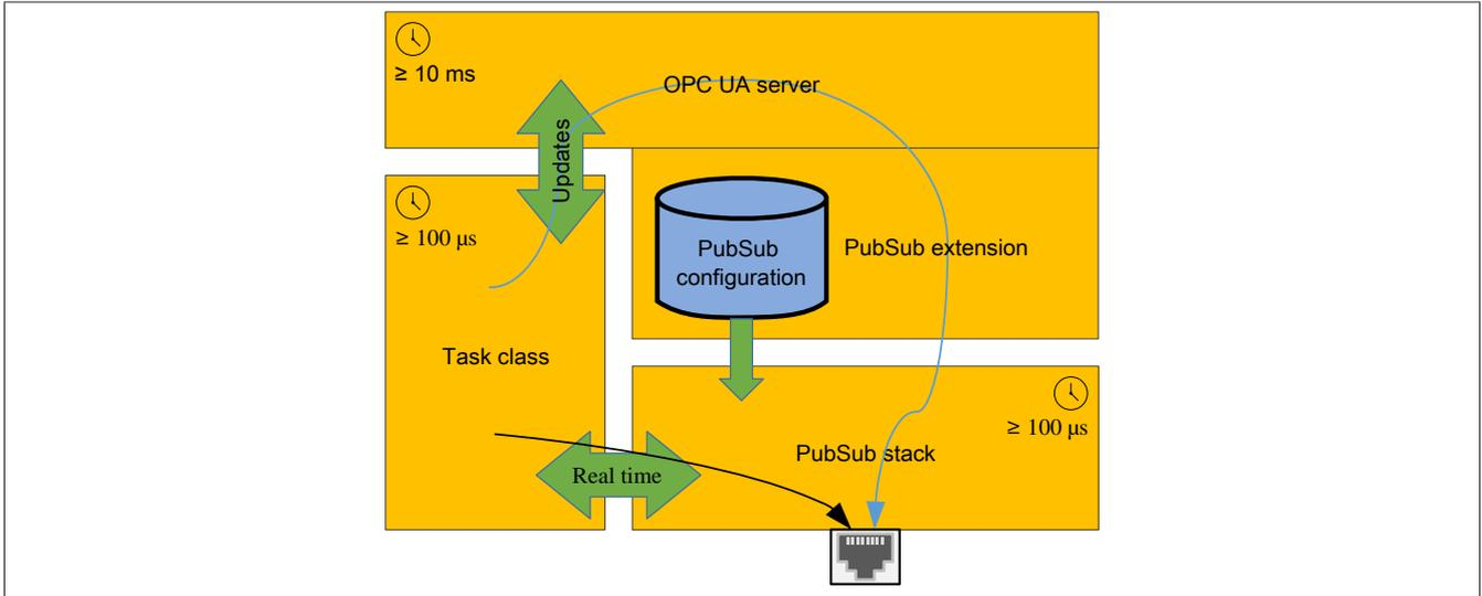
Each PubSub frame can be sent with its own cycle time and a time offset within the cycle. The network must provide appropriate mechanisms to also guarantee these hard real-time requirements on the receiver side of the network. These mechanisms are described in the following chapter about TSN.
