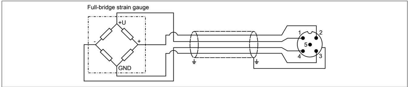
**6-wire strain gauge connection - Connection example**
