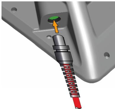
5. Secure the bushing with a size 19 wrench and a torque of 3 Nm.
