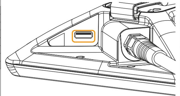
1) The USB interface is protected by a maintenance-free "USB current-limiting switch" (max. 0.5 A).
