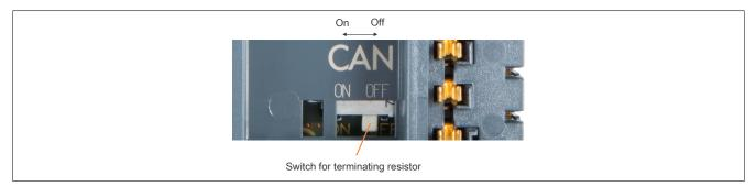
The bus module has an integrated CAN bus terminating resistor. The terminating resistor is switched on or off with a switch. An enabled terminating resistor is indicated on the power supply module by LED "T".
