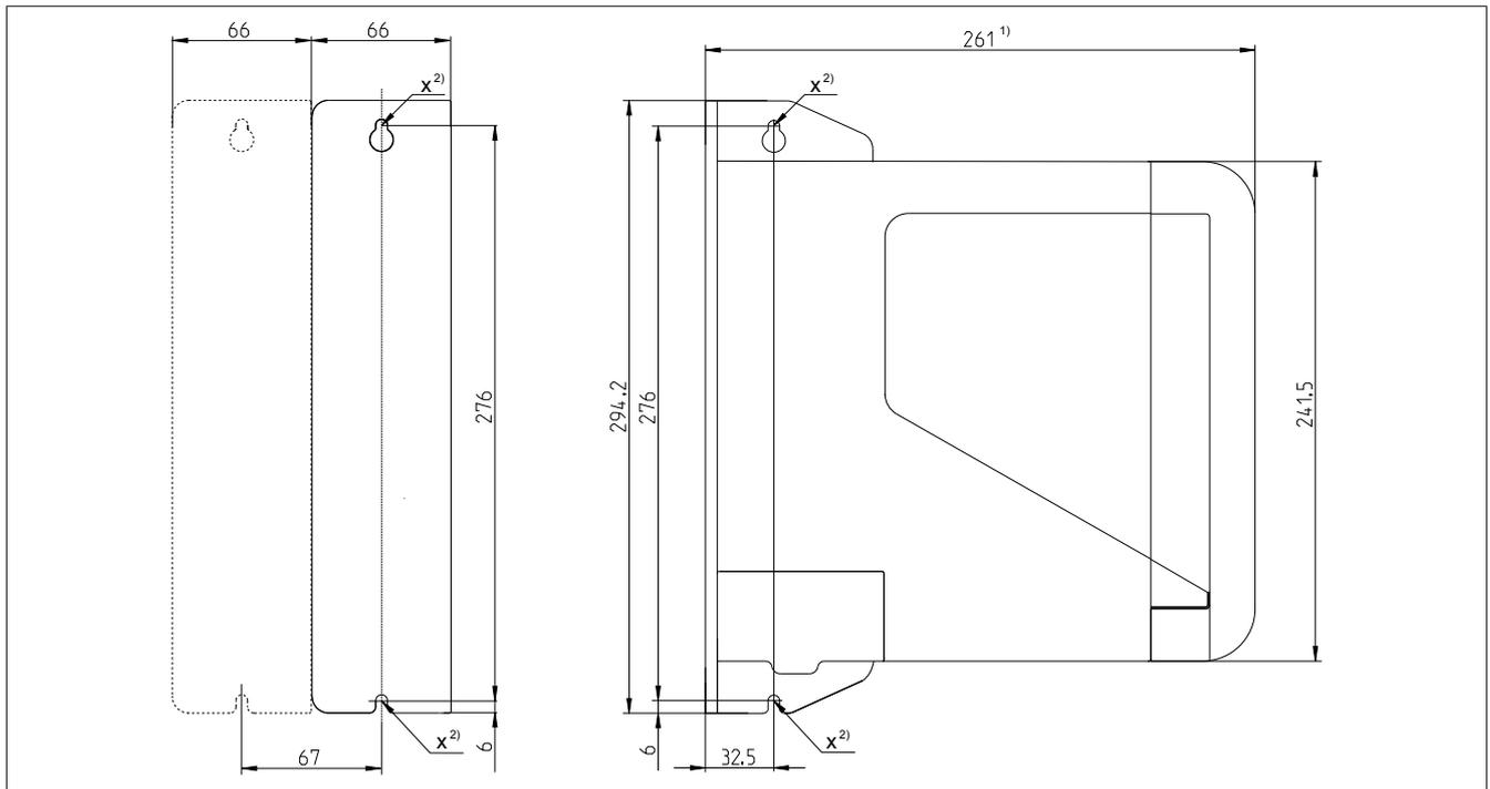
Figure 2: 1-axis module up to 4 kW - Dimension diagram
