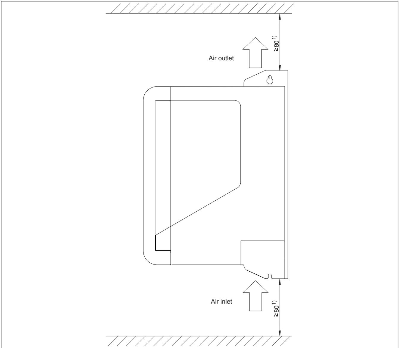
Figure 3: ACOPOS P3 8EI servo drives - Installation dimensions
