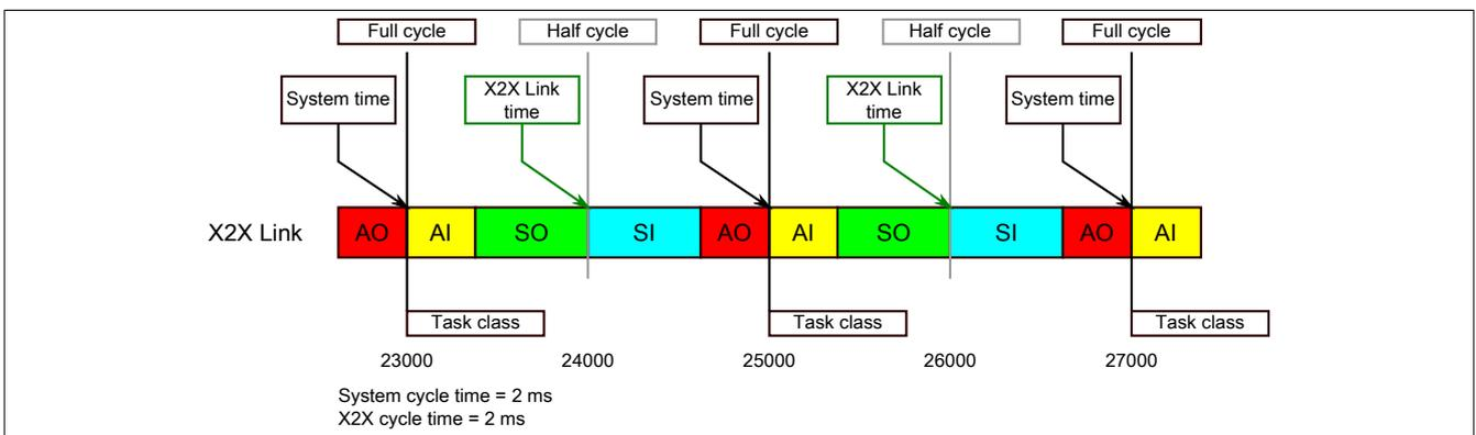
The reference moment on the X2X Link network is always calculated at the half cycle of the X2X Link cycle. This results in a difference between the system time and the X2X Link reference moment when the reference time is read out.
