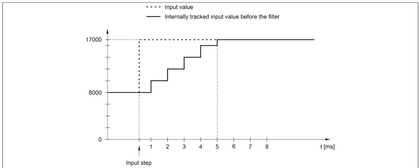
Figure 1: Tracked input value for input step
