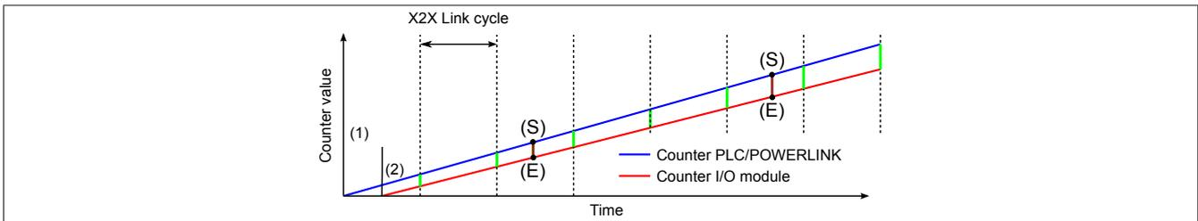
At startup, the internal counters for the PLC/POWERLINK (1) and the I/O module (2) start at different times and increase the values with microsecond resolution.
