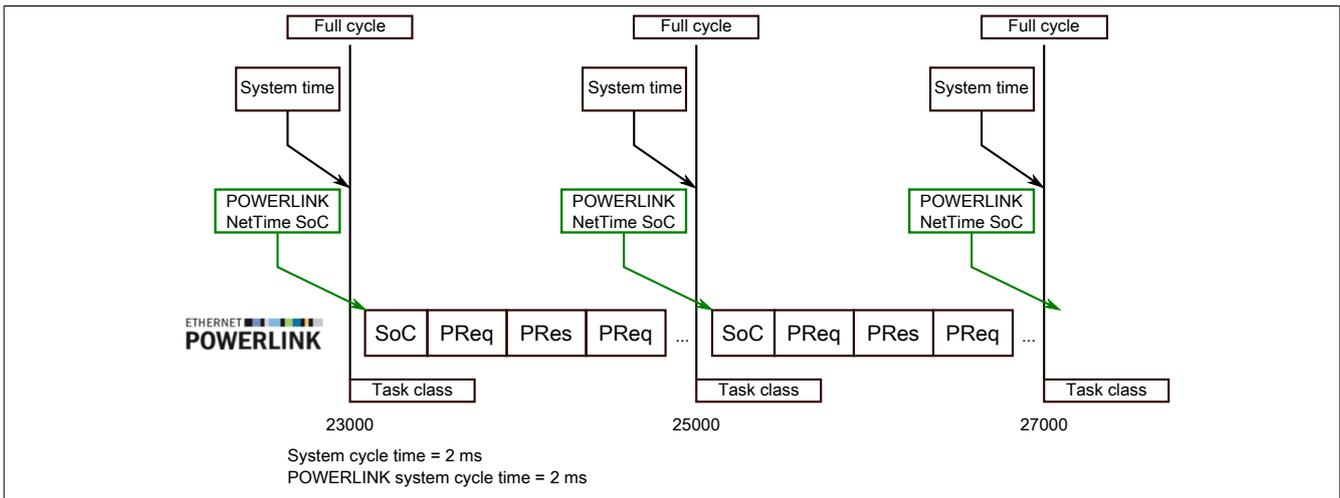
The reference moment on the POWERLINK network is always calculated at the start of cycle (SoC) of the POWERLINK network. The SoC starts 20  $\mu$ s after the system tick. This results in the following difference between the system time and the POWERLINK reference time:
