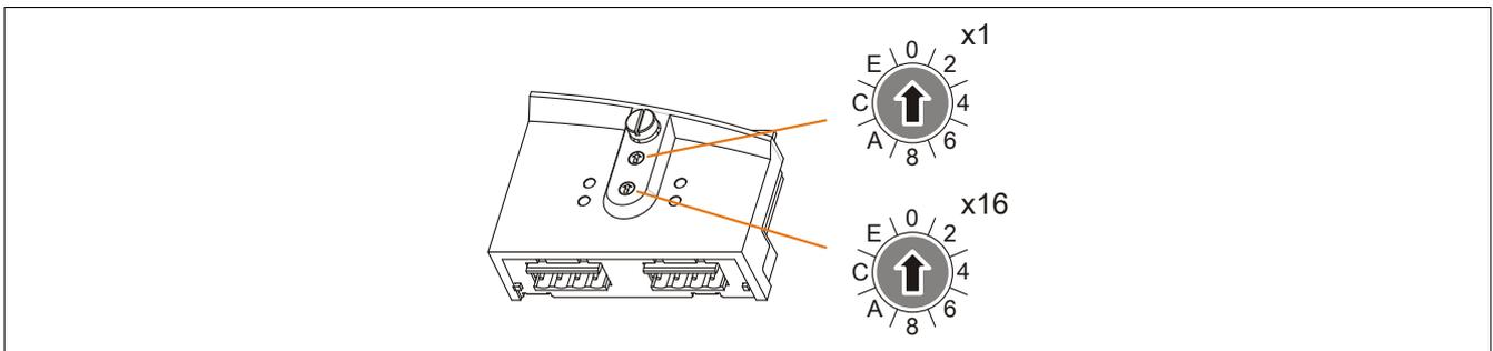
The node number for the CAN bus interfaces is set with the two hex switches. The configured node number applies to both interfaces.
