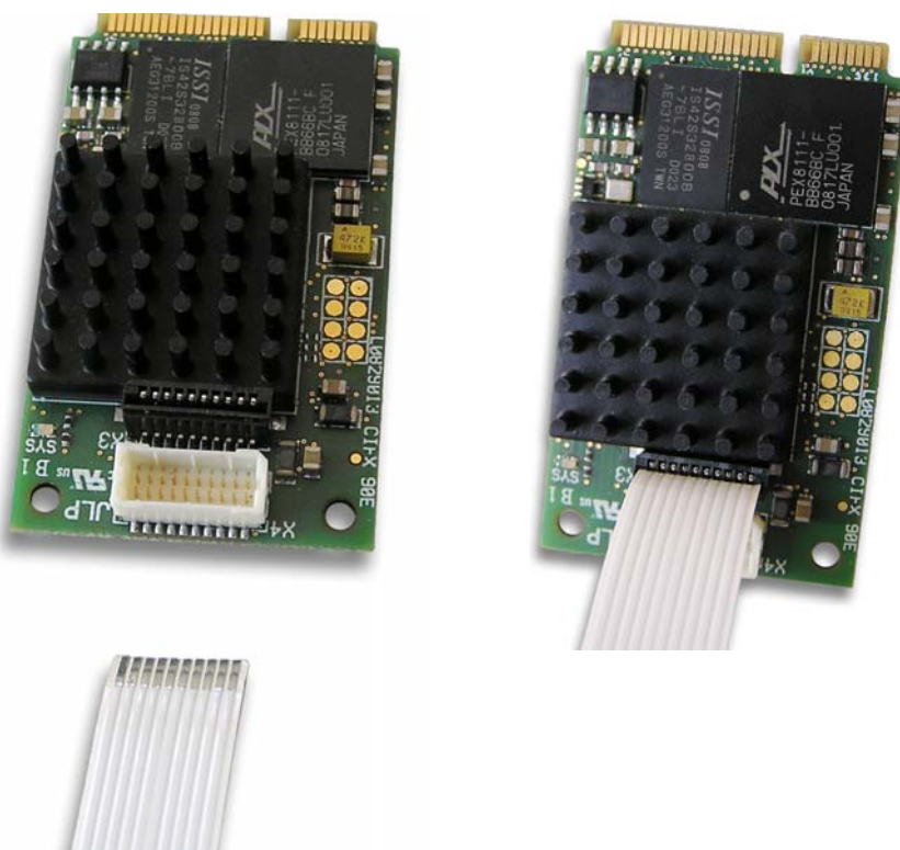
Figure 66: Connect the cable connector fieldbus X3 on the CIFX 90E card fieldbus* with the cable. (*Example in this figure)
