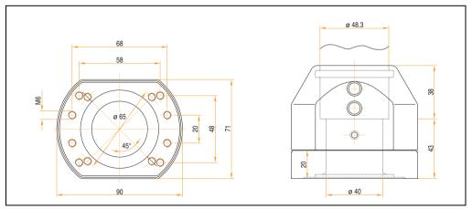
Figure 15: Dimensions - Flange 5AC725.FLGC-00
