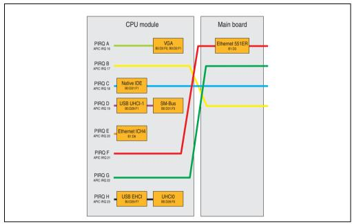
Figure 56: PCI Routing with activated APIC CPU board X945
