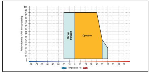
Figure 10: Temperature humidity diagram - PPC725
