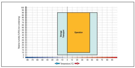
Figure 77: Temperature humidity diagram - USB flash drive - 5MMUSB.2048-00
