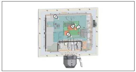
Figure 81: Temperature sensor locations
