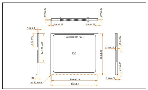
Figure 72: Dimensions - CompactFlash card Type I
