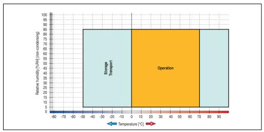
Figure 78: Temperature humidity diagram - USB flash drive - 5MMUSB.2048-01
