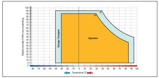
Figure 19: Temperature humidity diagram - Add-on hard disk 5AC600.HDDI-06
