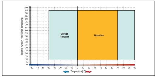
5.3.1 Temperature humidity diagram - Operation and storage
