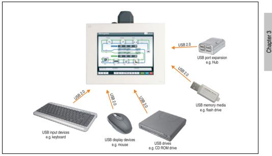
Figure 26: Local connection of USB peripheral devices on the PPC 725
