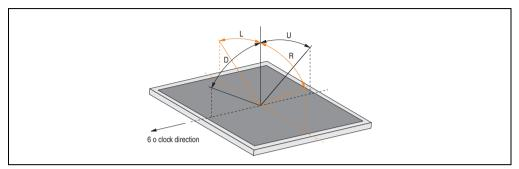
Figure 85: Viewing angle definition
