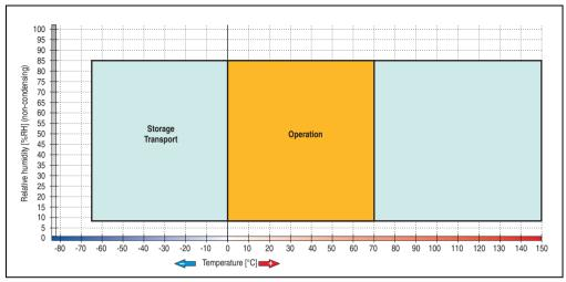
4.3.1 Temperature humidity diagram - Operation and storage
