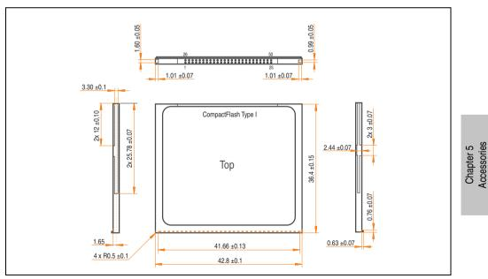
Figure 76: Dimensions - CompactFlash card Type I
