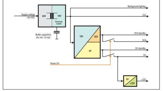
The following block diagram shows the simplified structure of the PPC725 supply voltage.
