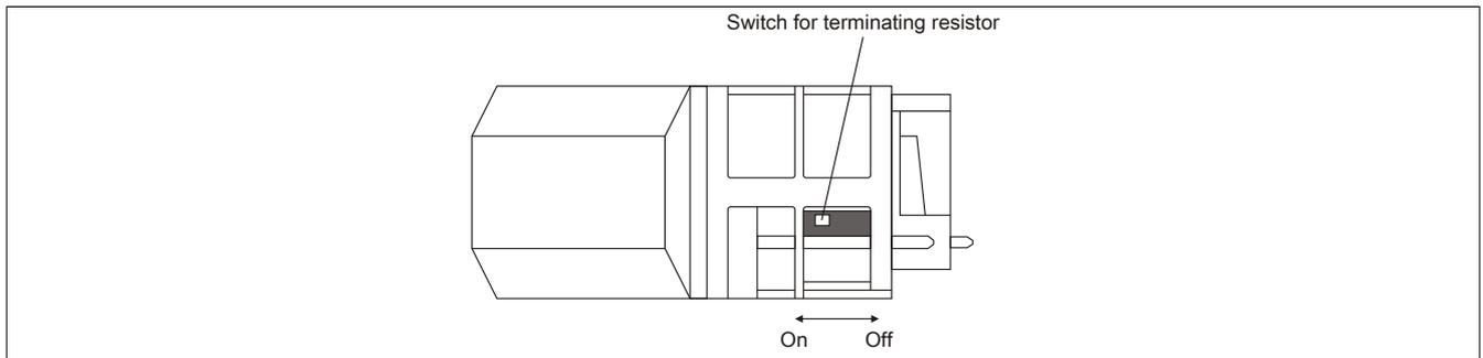
A terminating resistor is integrated in the interface module. It can be switched on or off with a switch on the bottom of the housing. A switched-on terminating resistor is indicated by LED "TERM".
