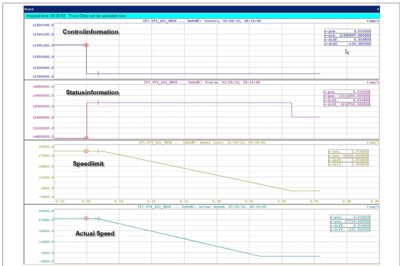
Figure 64: ACOPOSmulti Trace: Example with SafeMOTION data
