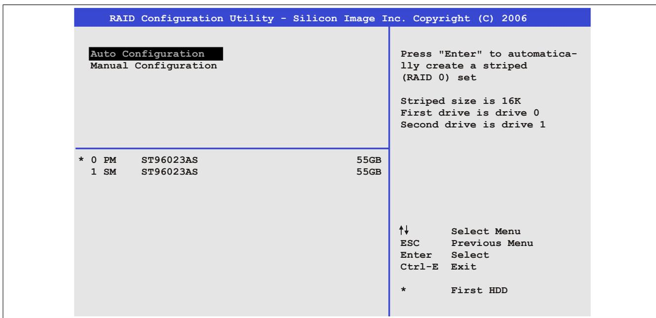
Abbildung 108: RAID Configuration Utility - Create RAID set - Striped
