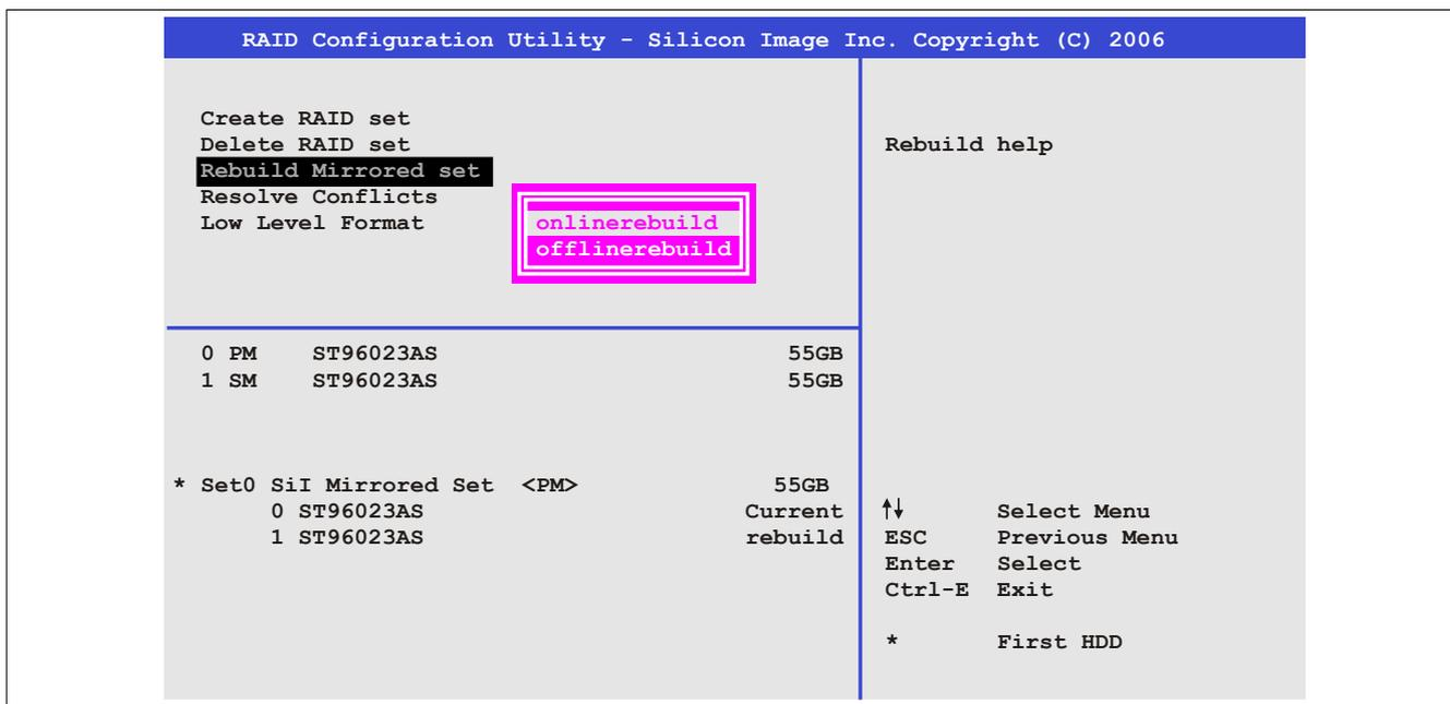
Abbildung 111: RAID Configuration Utility - Rebuild Mirrored set
