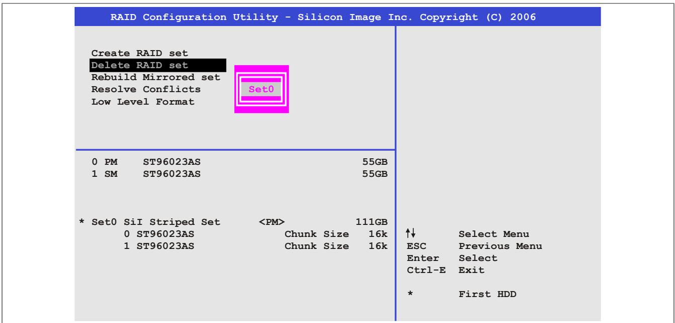
Abbildung 110: RAID Configuration Utility - Delete RAID set
