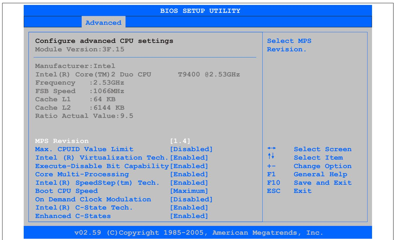
Abbildung 123: GM45 Advanced CPU Board Monitor
