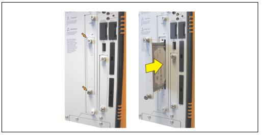
Figure 206: Mounting the slide-in compact drive
