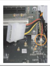
Figure 256: Connector location for external devices
