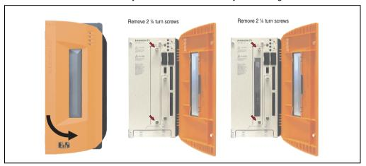
Figure 204: Loosening the 1/4 turn screws
