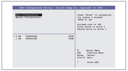
Figure 101: RAID Configuration Utility - Create RAID set - striped
