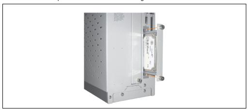
Figure 201: Inserting the compact SATA drive
