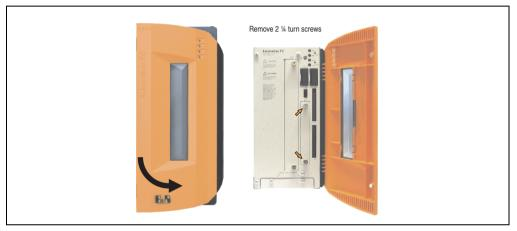
Figure 200: Loosening the 1/4 turn screws
