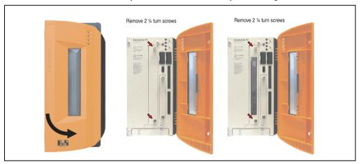
Figure 202: Loosening the 1/4 turn screws
