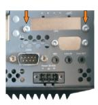
Figure 228: Remove UPS module cover
