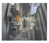
Figure 225: Install UPS module
