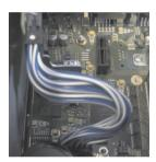
Figure 226: Plug in connection cable
