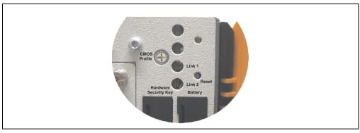
Figure 139: CMOS Profile Hex Switch
