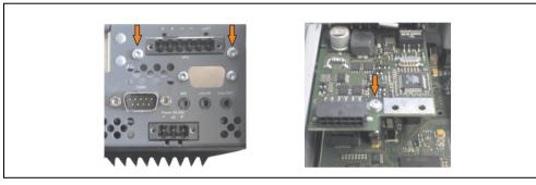
Figure 213: Install UPS module
