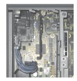
Figure 243: Plug in connection cable
