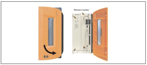
Figure 246: Mounting the side cover - APC810 2 card slot
