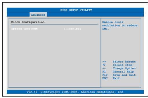
Figure 119: 945GME Advanced Clock Configuration
