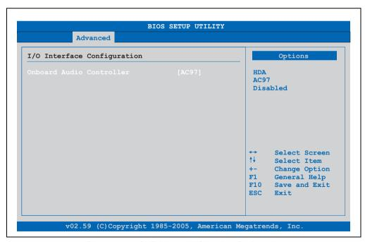
Figure 118: 945GME Advanced I/O Interface Configuration
