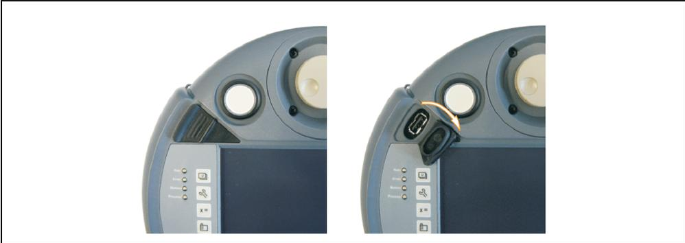
Figure 43: USB interface - open protective cap
