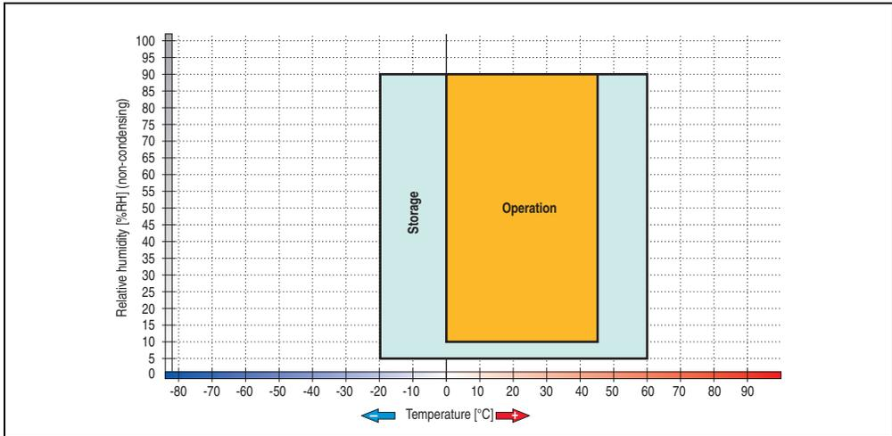
Figure 59: Temperature humidity diagram - USB flash drive - 5MMUSB.xxxx-00
