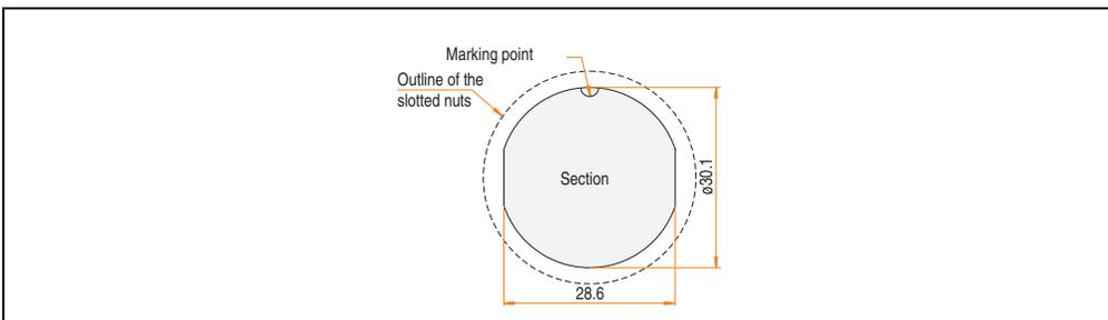
Figure 34: Drilling template - Receptacle
