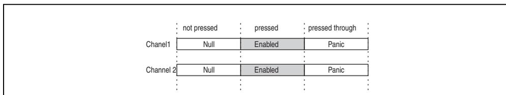
Figure 17: Possible enable switch positions
