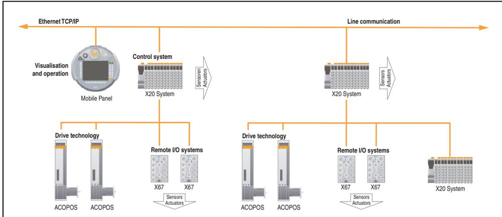
Figure 2: Mobile operation and monitoring
