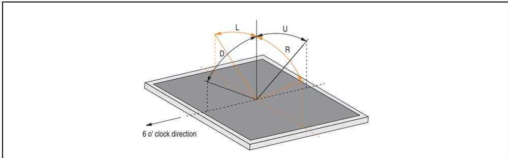
Figure 70: Viewing angle definition
