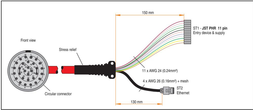
Figure 28: Attachment cable specifications 5CAMPH.0xxx-30
