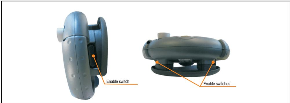
Figure 16: Enabling device
