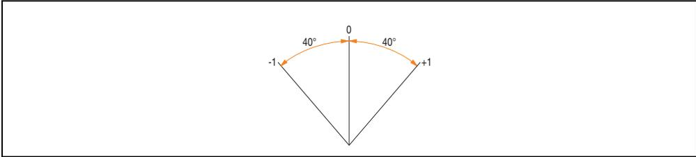
Figure 8: Key switch - Angle of rotation
