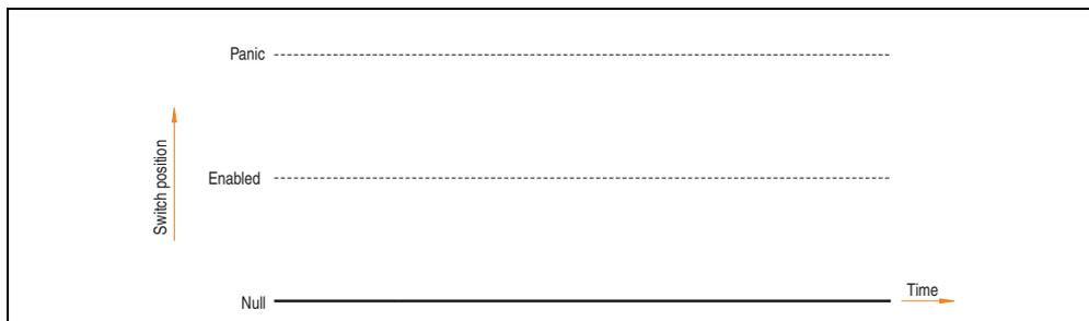
Figure 18: Enable switch - zero position
