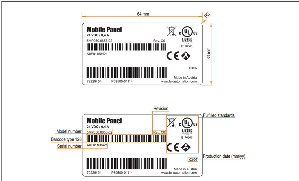
Figure 11: Design / dimensions - Serial number sticker
