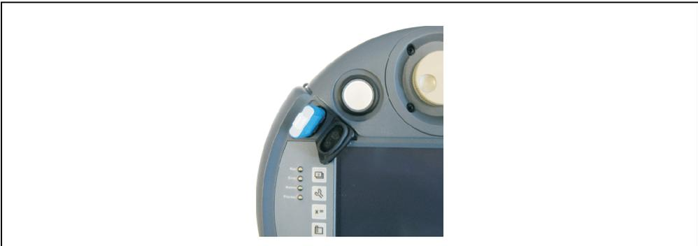
Figure 44: USB interface - insert flash drive
