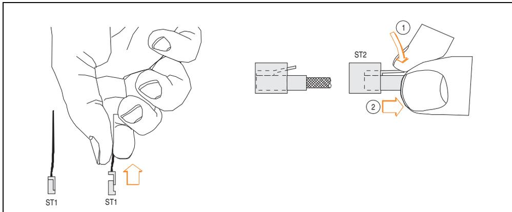
Figure 38: Removing ST1 and ST2
