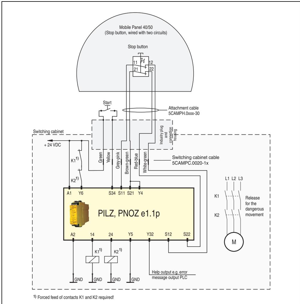
Figure 41: Connection example for stop button
