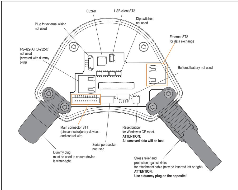
Figure 37: Attachment shaft
