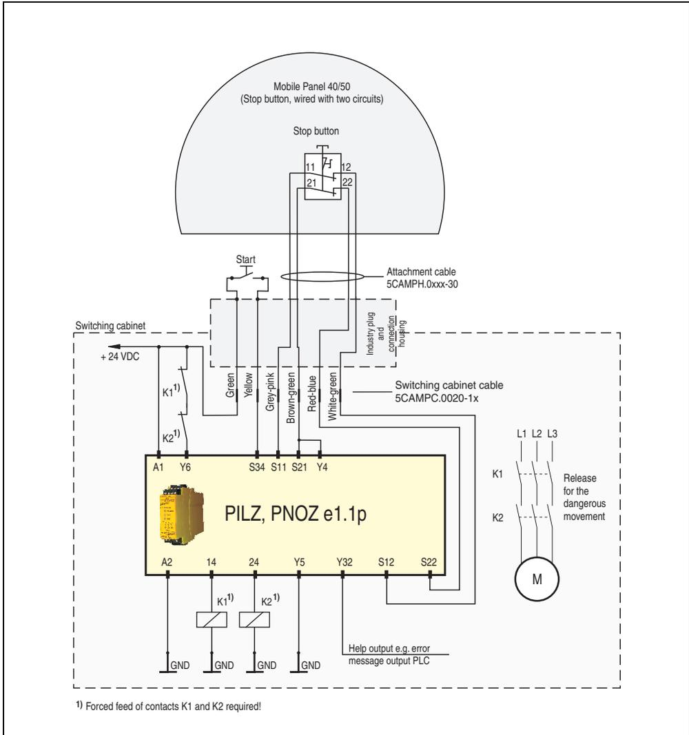
Figure 42: Connection example - Enable switch
