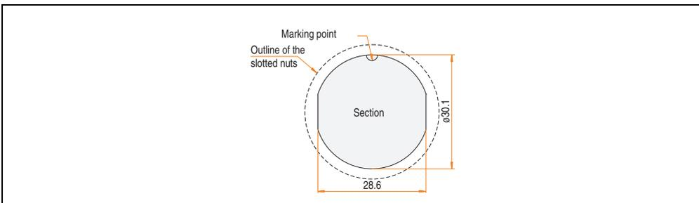
Figure 31: Drilling template - Receptacle
