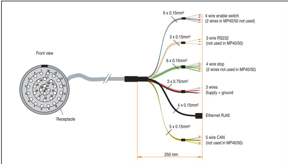
Figure 33: Cable layout - switching cabinet cable 5CAMPC.0020-11
