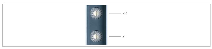
The X2X Link address of the module is set using the node number switches (0x01 to 0xFD).
