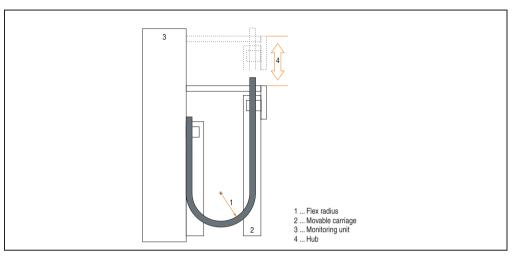
Figure 113: Test structure - cable drag chain
