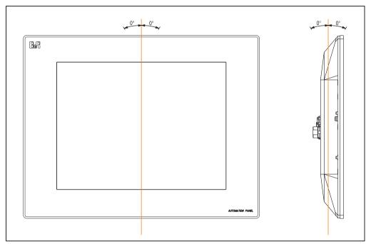
Figure 95: Mounting orientation 0°
