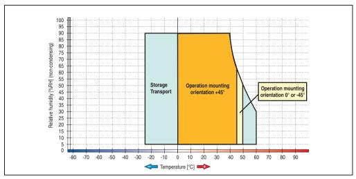
Figure 20: Temperature humidity diagram - 5AP880.1505-00
