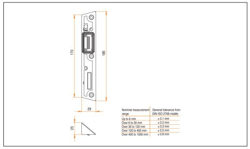
Figure 61: Dimensions - extension cover 5AC800.COV1-00
