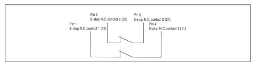
Figure 23: E-stop circuit connections
