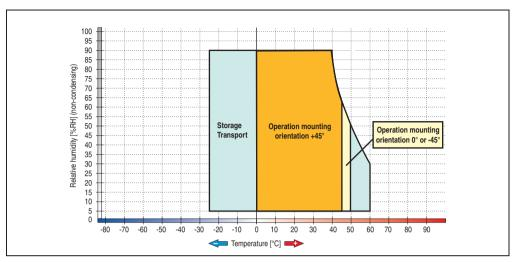
Figure 16: Temperature humidity diagram - 5AP820.1505-00
