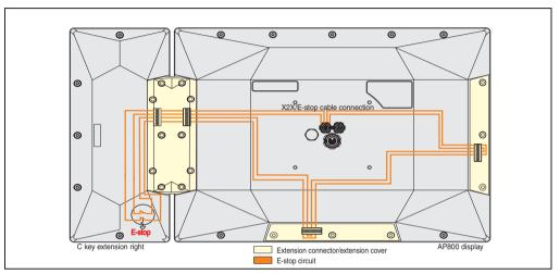
Figure 91: E-stop wiring diagram for the extension unit with E-stop - rear view
