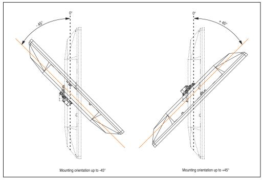
Figure 96: Mounting orientation -45° and +45°.
