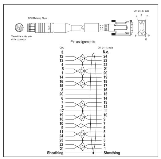
Figure 78: Pin assignments - SDL cable 5CASDL.0xxx-20 Rev. ≥ A5
