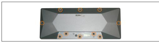
Figure 119: Remove screws
