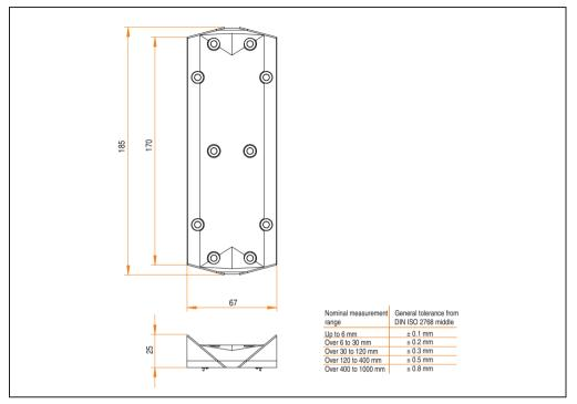
Figure 65: Dimensions - extension connector 5AC800.CON1-00
