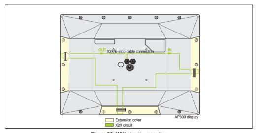
Figure 88: X2X circuit - rear view
