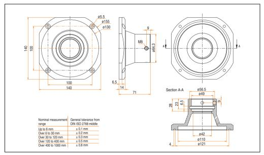
Figure 69: Dimensions - extension flange 5AC800.FLG1-00
