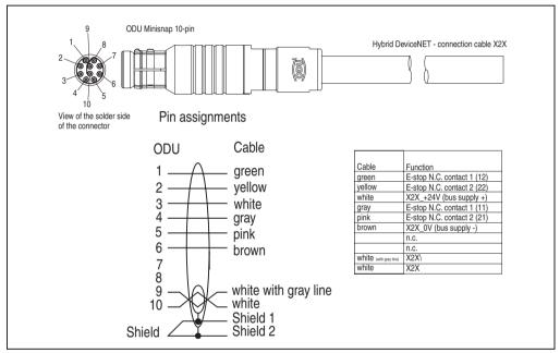
Figure 87: Pin assignments - X2X cable 5CAX2X.0xxx-00
