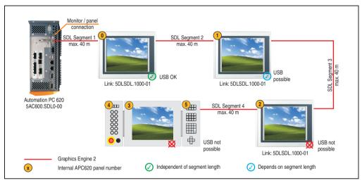
Figure 99: Configuration - Three AP900 devices and an AP800 via SDL (onboard)
