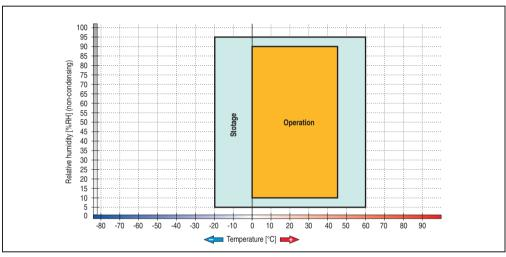
Figure 114: Temperature humidity diagram - USB flash drive - 5MMUSB.xxxx-00
