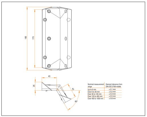
Figure 67: Dimensions - extension connector 60° 5AC800.CON2-00
