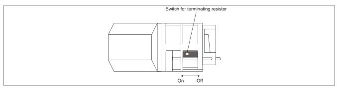
A terminating resistor is already integrated on the bus controller. It can be turned on and off with a switch on the bottom of the housing. An active terminating resistor is indicated by the "TERM" LED.
