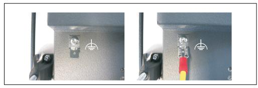
Figure 99: Functional grounding clip
