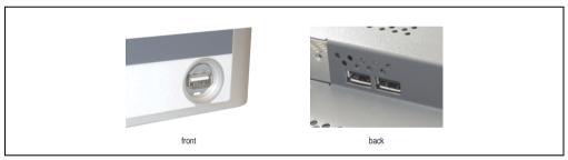
Figure 3: Automation Panel USB connections (front side - back side)
