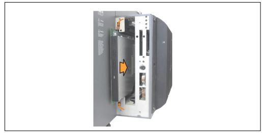
Figure 368: Installing the slide-in drive
