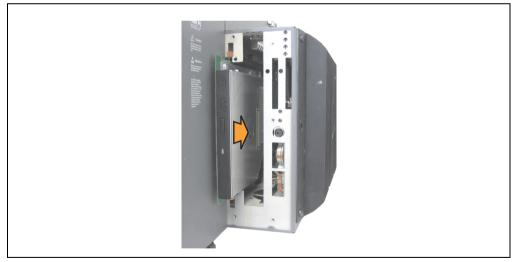
Figure 365: Installing the slide-in drive
