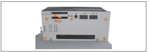
Figure 361: Removing the side cover
