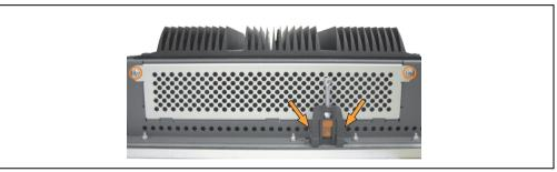
Figure 353: Removing the fan kit cover
