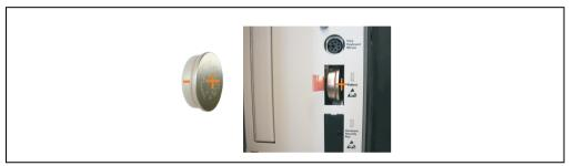
Figure 352: Battery polarity
