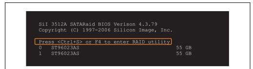
Figure 154: Open the RAID Configuration Utility
