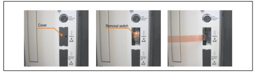
Figure 350: Battery removal
