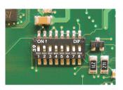
Figure 198: DIP switch on system unit
