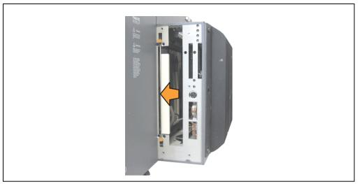
Figure 364: Removing the slide-in dummy module
