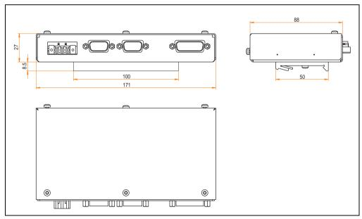
Figure 292: Dimensions - GS link remote unit 5A5010.02
