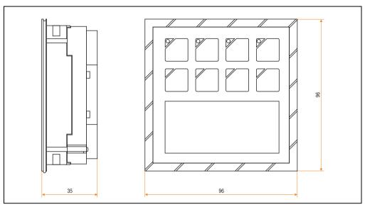
Figure 193: Dimensions - keypad module with 8 keys
