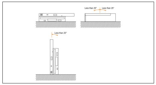
Figure 41: Mounting guidelines - 5A5600.05
