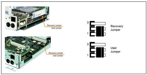
Figure 66: Recovery jumper / User jumper IPC5000 (above) and IPC5600 (below)
