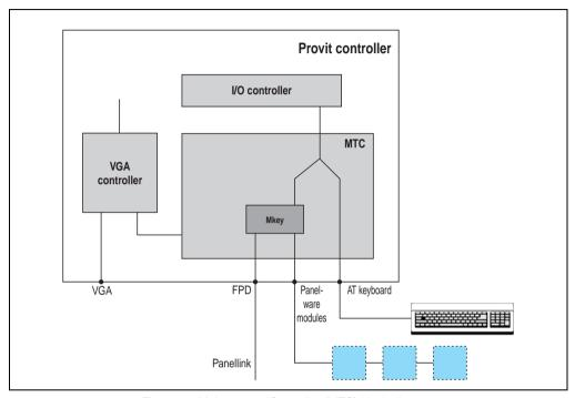
Figure 67: Maintenance Controller (MTC) block diagram
