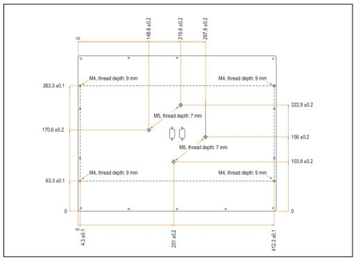
Figure 154: Flange drill holes - 5D5212.04 revision G0 and later
