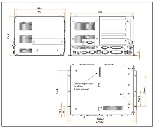
Figure 10: Dimensions - IPC5000C (5-slot design + optional add-on drive)
