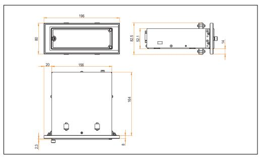
Figure 265: Dimensions - 5A5003.02 with front cover 5A5003.03
