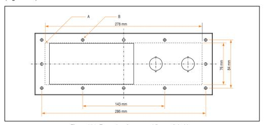
Figure 261: Front plate for external floppy disk drive
