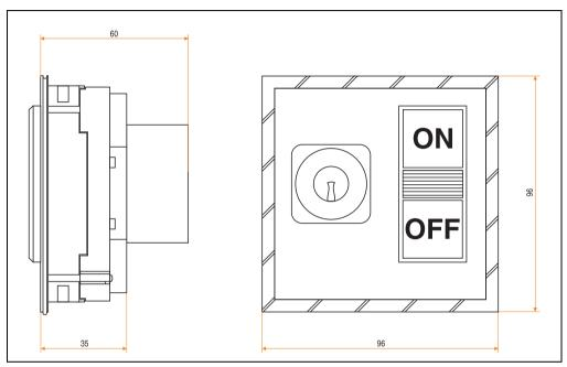
Figure 197: Dimensions - keypad module with key switch
