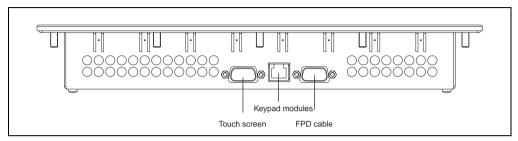
Figure 117: Connections 5D5200.01 and 5D5210.01 revision >= G0
