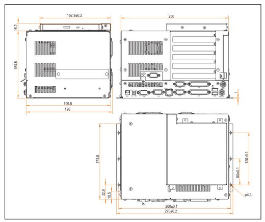
Figure 11: Dimensions - IPC5000C (5-slot design + add-on drive 5A5009.0x)
