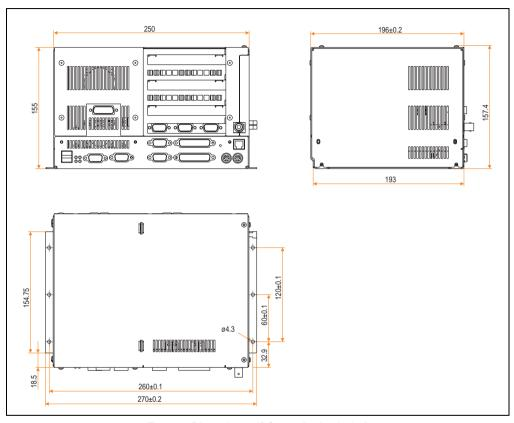
Figure 8: Dimensions - IPC5000 (4-slot design)
