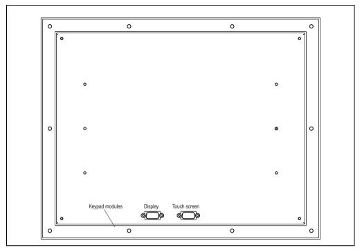
Figure 149: Connections - 5D5212.02 revision < I0
