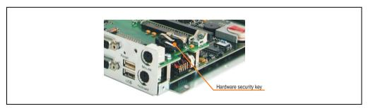
Figure 73: Hardware security key
