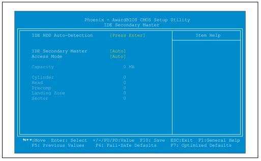
Figure 212: IDE secondary master setup
