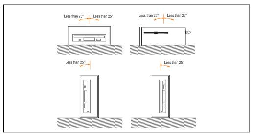
Figure 262: Mounting guidelines - external 3.5" FDD
