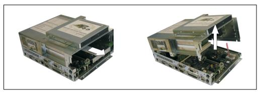
Figure 319: Removing the cover and bus unit
