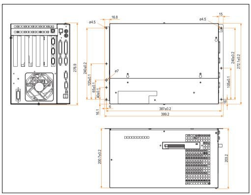
Figure 16: Dimensions - IPC5600 (6-slot design)
