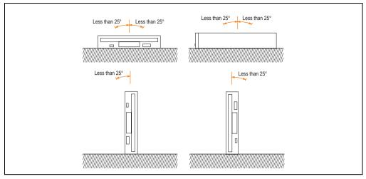
Figure 37: Mounting guidelines - 5A5600.03
