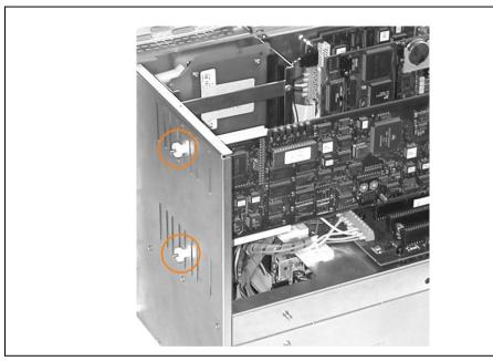
Figure 84: Fasteners for full-size cards
