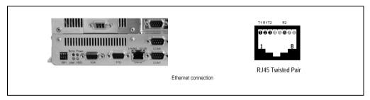
Figure 81: Ethernet connection
