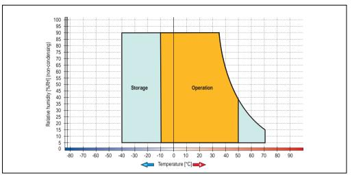
Figure 317: Temperature humidity diagram - Elo Accu touch screen 5-wire
