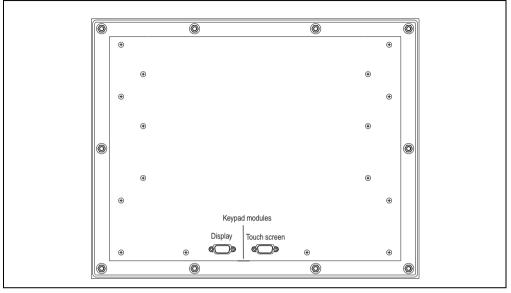
Figure 135: Connections - 5D5211.03 revision I0
