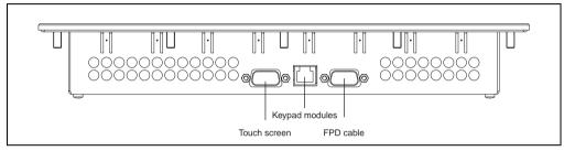
Figure 128: Connections - 5D5211.02 revision >= F0
