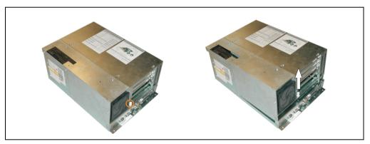
Figure 321: Unlocking the safety pins and removing the bus unit
