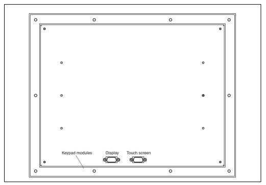
Figure 134: Connections - 5D5201.03 and 5D5211.03
