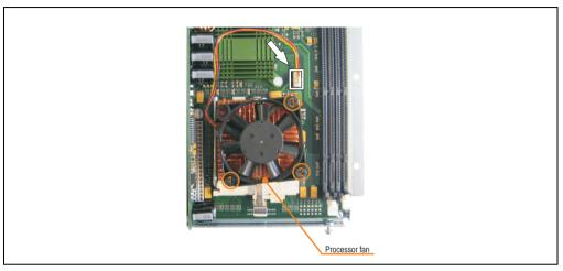
Figure 329: Fastening the fan and connecting the plug
