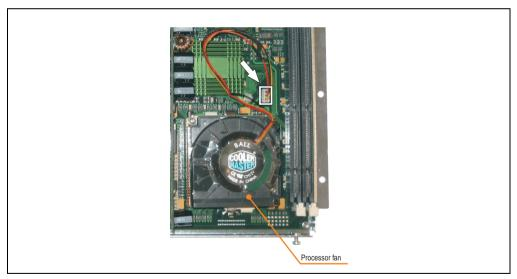
Figure 327: Connecting the plug
