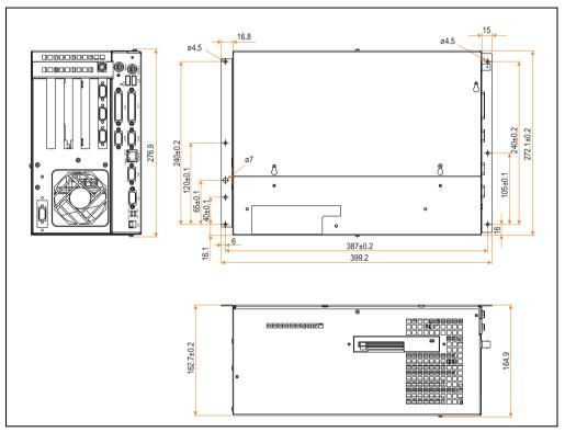
Figure 13: Dimensions - IPC5600C (4-slot design)
