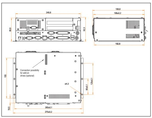
Figure 6: Dimensions - IPC5000C (2-slot design + optional add-on drive)
