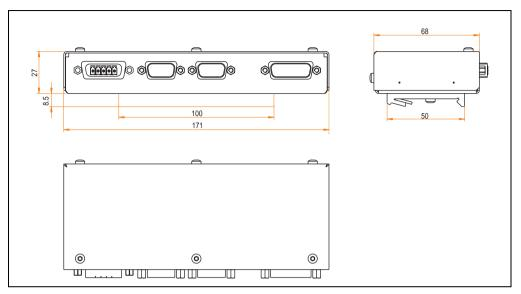
Figure 289: Remote display adapter - local unit 5A5010.01 - dimensions
