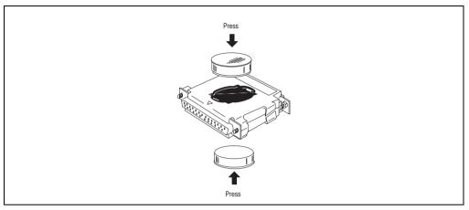
Figure 293: Hardware security key parallel adapter
