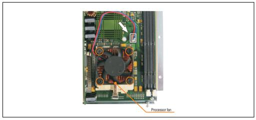
Figure 328: Removing the screws and plug
