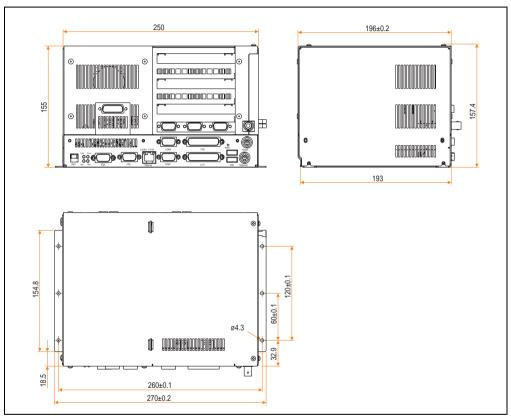
Figure 9: Dimensions - IPC5000C (4-slot design)
