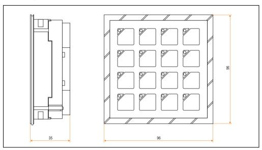
Figure 189: Dimensions for standard keypad modules
