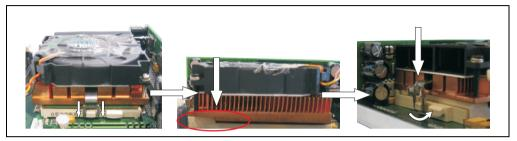
Figure 326: Attaching the new heat sink
