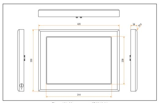
Figure 151: Measurements 5D5212.04
