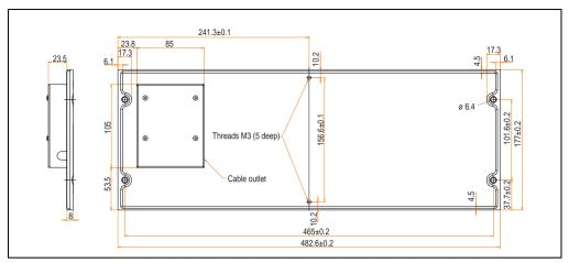
Figure 295: Installation dimensions 19" AT keyboard (figure overleaf)
