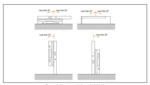
Figure 43: Mounting guidelines - 5A5600.07
