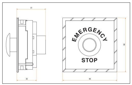
Figure 196: Dimensions - keypad module with E-stop button
