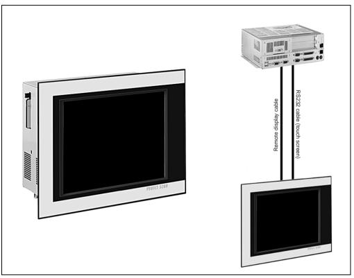
Figure 107: Standard mounting (left) and remote mounting (right)
