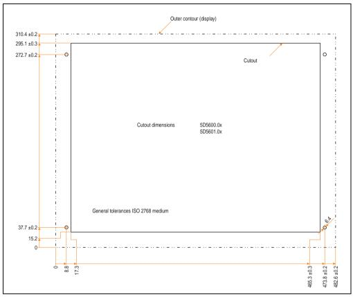
Figure 174: Cutout installation - 5D5600.0x and 5D5601.0x
