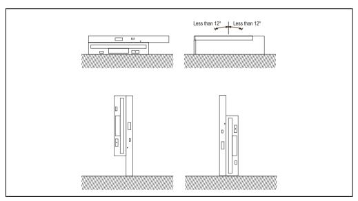
Figure 39: Mounting guidelines - 5A5600.04
