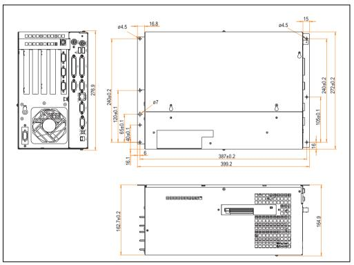
Figure 15: Dimensions - IPC5600C (5-slot design)
