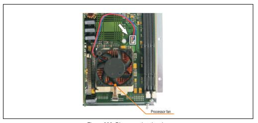
Figure 322: Disconnecting the plug
