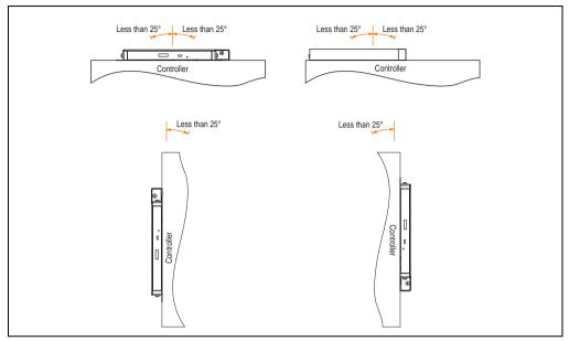
Figure 282: Mounting instructions - add-on CD ROM with controller
