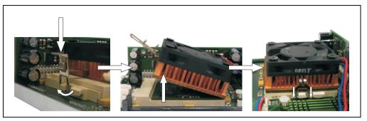
Figure 324: Removing the heat sink
