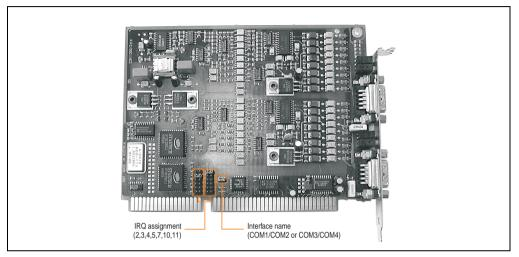
Figure 256: Jumper position
