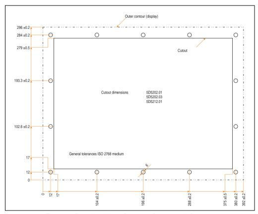
Figure 142: Cutout installation - 5D5202.01, 5D5202.03 and 5D5212.01
