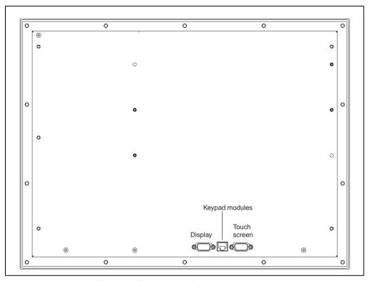
Figure 148: Connections - 5D5212.02 revision >= I0
