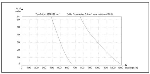
Figure 316: CAN - number of nodes / bus length
