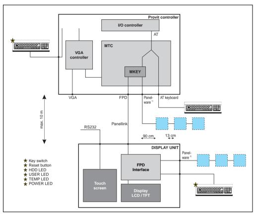
Figure 109: Block diagram for controller, display and peripherals
