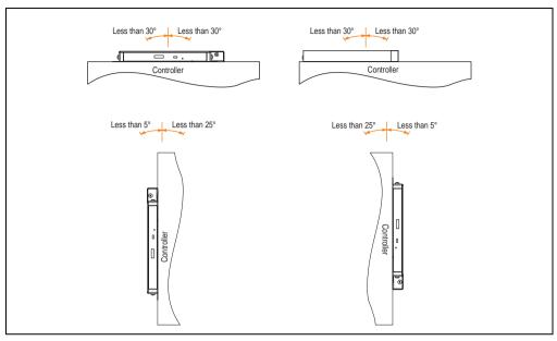
Figure 287: Mounting instructions - add-on CD RW (revision D0 and later) with controller
