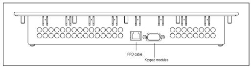
Figure 113: Connections 5D5100.01 and 5D5100.04
