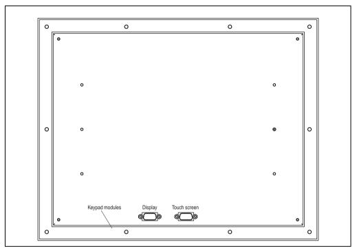
Figure 143: Connections 5D5202.01, 5D5202.03 and 5D5212.01
