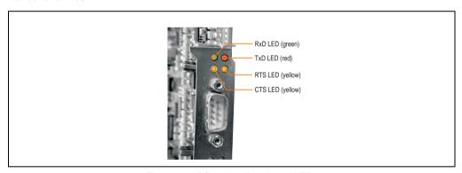
Figure 255: RS232 interface board LEDs
