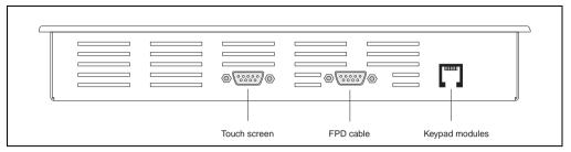
Figure 127: Connections 5D5201.02 and 5D5211.02
