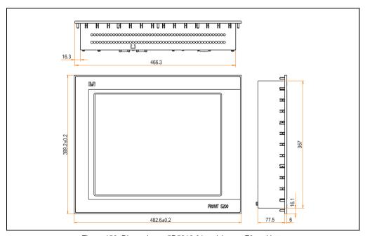
Figure 156: Dimensions - 5D5213.01 revision >= F0 and later
