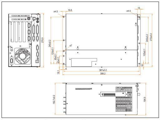
Figure 14: Dimensions - IPC5600 (5-slot design)
