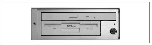
Figure 44: 5A5600.09 flush with a display unit 5D560x.0x
