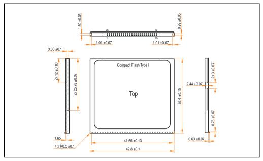
Figure 96: Dimensions - CompactFlash card Type I
