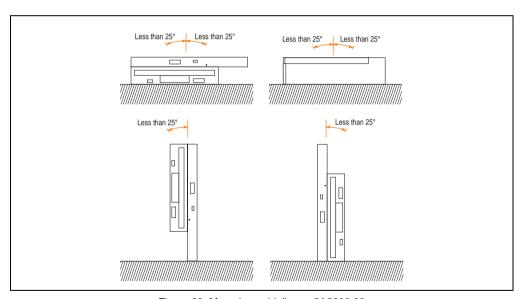
Figure 33: Mounting guidelines - 5A5600.02
