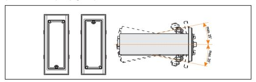
Figure 266: Mounting guidelines - controller R-IDE CD-ROM/LS120 drive (horizontal / vertical)
