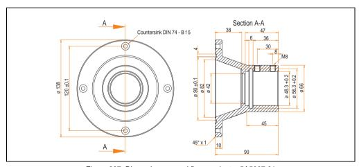
Figure 297: Dimensions - panel flange adapter 5A5007.01
