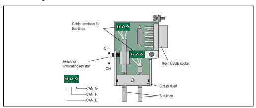
Figure 105: CAN bus connector 7AC911.9
