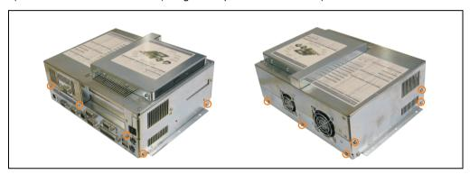
Figure 318: Removing the screws
