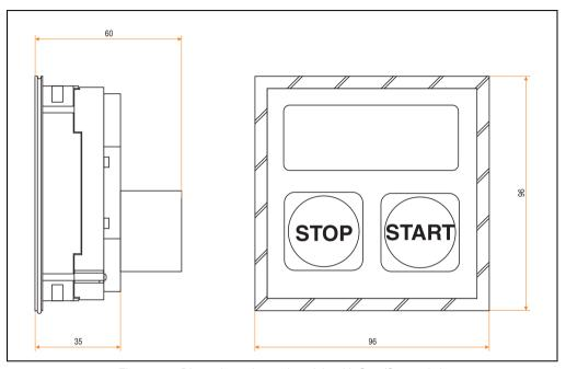
Figure 198: Dimensions - keypad module with Start/Stop switch
