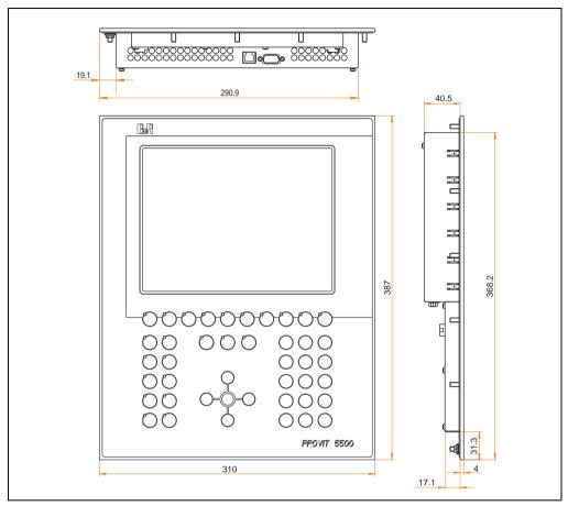
Figure 167: Dimensions - 5D5510 revision F0 and later
