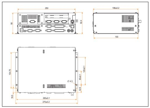
Figure 4: Dimensions - IPC5000 (2-slot design)
