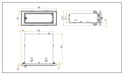
Figure 274: Dimensions - 5A5003.08 with 5A5003.03
