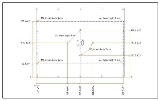
Figure 153: Flange drill holes - 5D5212.04 revision J0 and later
