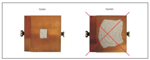
Figure 325: Applying heat conductive paste
