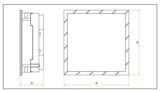
Figure 195: Dimensions - dummy module
