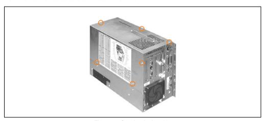
Figure 49: Opening the housing
