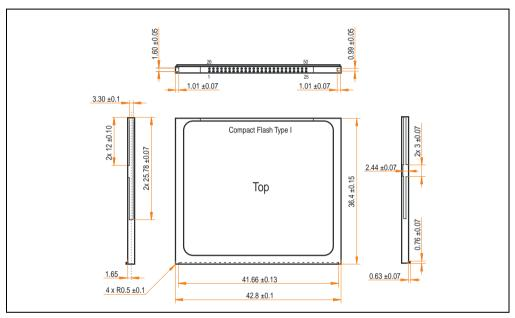
Figure 94: Dimensions - CompactFlash card Type I
