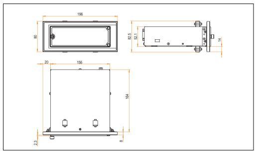
Figure 269: Dimensions - 5A5003.07 with front cover 5A5003.03
