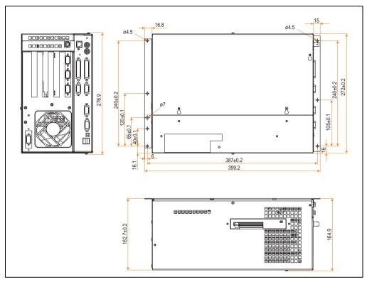
Figure 12: Dimensions - IPC5600 (4-slot design)
