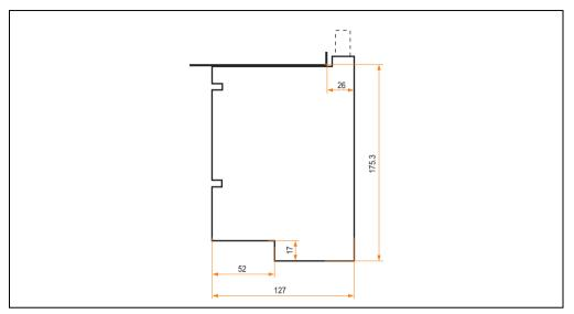
Figure 101: Dimensions - interface board
