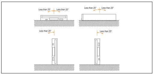
Figure 31: Mounting guidelines - 5A5600.01
