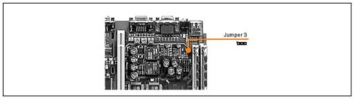
Figure 60: Location of the jumpers for DRAM operating voltage
