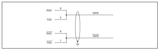
Figure 102: Operation of COM3 or COM4 interface in RS485 mode
