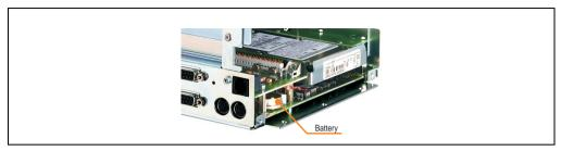
Figure 64: Battery compartment
