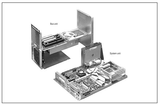
Figure 51: Detaching the bus unit
