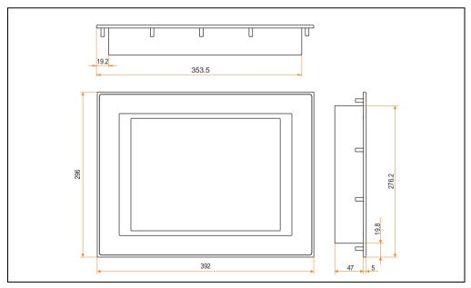
Figure 141: Measurements 5D5202.01, 5D5202.03 and 5D5212.01
