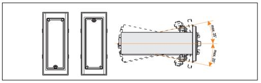
Figure 270: Mounting guidelines - controller R-IDE CD-ROM/LS120 drive (horizontal / vertical)
