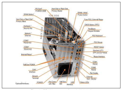
Figure 21: IPC5600 components (bus unit with 4 slots)
