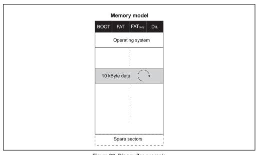
Figure 98: Ring buffer example
