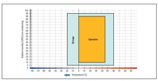
Figure 298: Temperature humidity diagram - USB flash drive - 5MMUSB.xxxx-00
