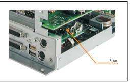
Figure 72: Fuse position for IPC5000C (left) and IPC5600C (right)
