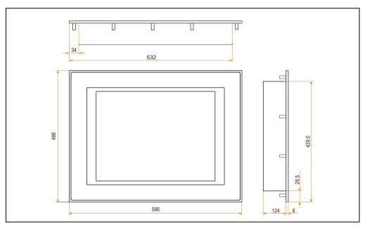
Figure 162: Measurements 5D9200.01
