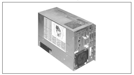
Figure 46: Drives accessible from the back of the controller
