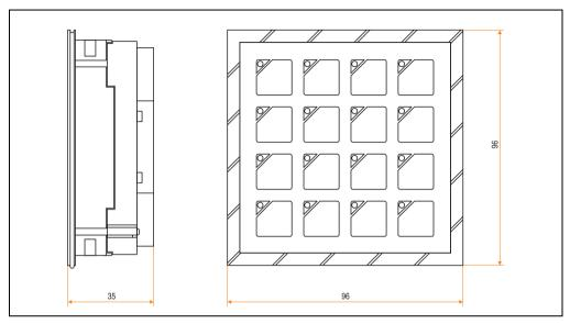
Figure 191: Dimensions - keypad module with 16 keys
