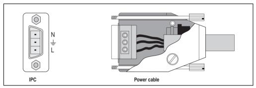
Figure 86: Plug and socket (3-pin) for AC supply
