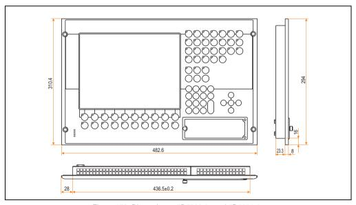
Figure 173: Dimensions - 5D5600.0x and 5D5601.0x
