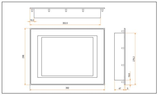
Figure 120: Measurements 5D5200.04
