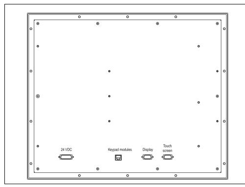
Figure 160: Connections - 5D5213.01 revision < F0
