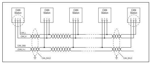
Figure 103: Bus cable - station connection
