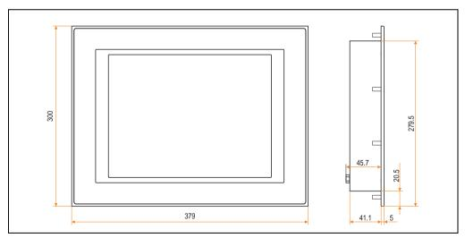
Figure 130: Measurements 5D5201.03 and 5D5211.03
