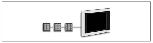
Figure 79: Connecting Panelware keypad modules
