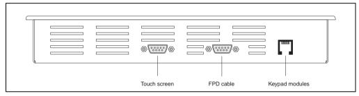
Figure 118: Connections 5D5200.01 and 5D5210.01 revision <G0
