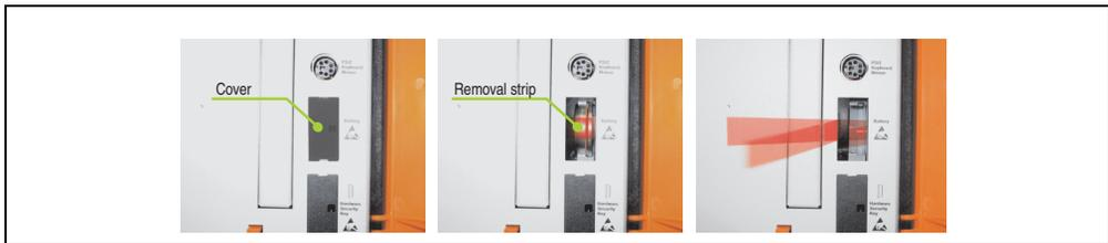
Figure 372: Battery removal
