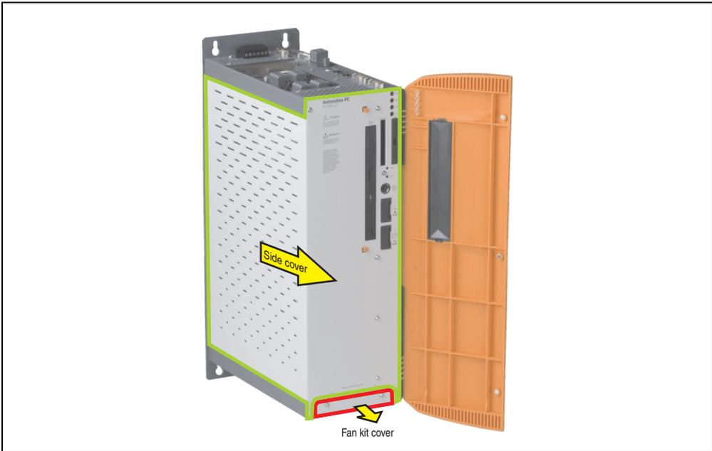
Figure 388: APC620 3PCI slots - Remove side cover and fan kit cover
