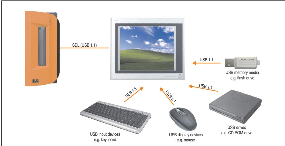
Figure 161: Remote connection of USB peripheral devices to the APC800/900 via SDL
