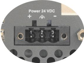
Figure 37: Supply voltage connection
