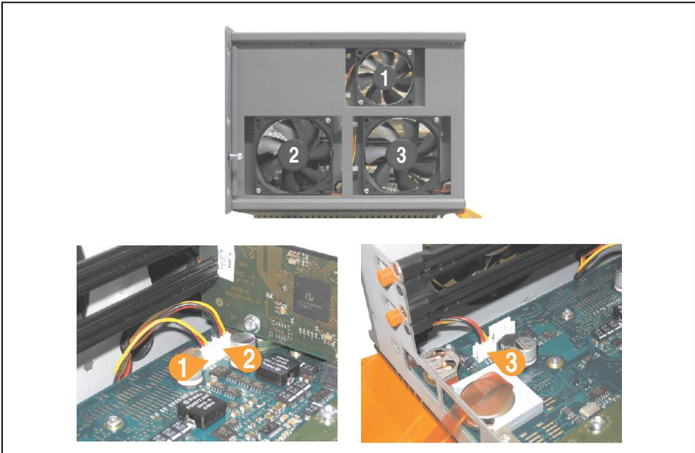
Figure 398: APC620 5PCI slot - Fan cable connection to the main board
