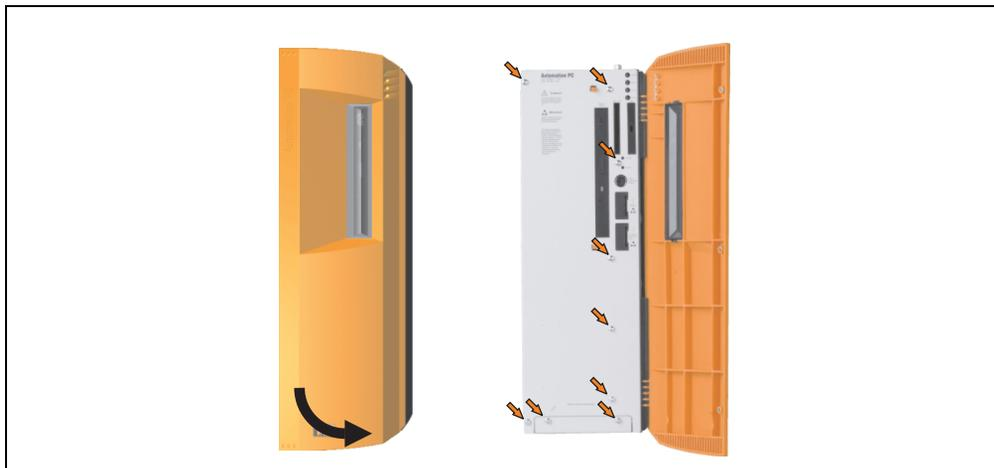
Figure 387: APC620 3PCI slot - Remove screws to install/ remove filter kit
