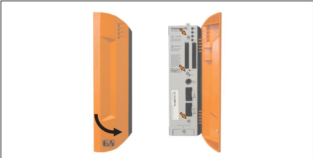
Figure 444: Mounting the side cover - APC620, 1 PCI slot
