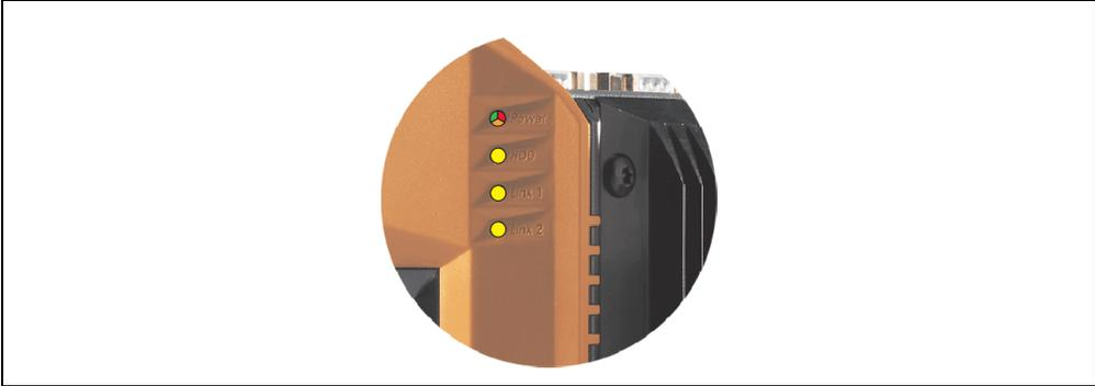
Figure 46: Front-side status LEDs
