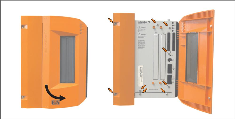
Figure 393: APC620 5PCI slot - Remove screws to install/ remove filter kit
