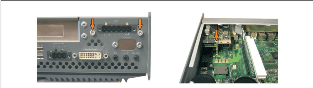
Figure 408: Install UPS module
