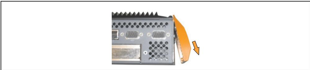
Figure 453: Removing the APC620 front cover
