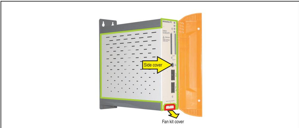
Figure 377: APC620 1PCI slot - Remove side cover and fan kit cover
