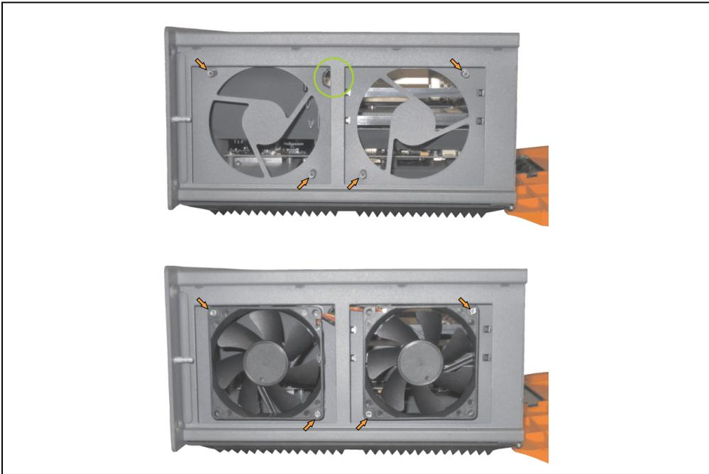
Figure 390: APC620 3PCI slot - Fan installation
