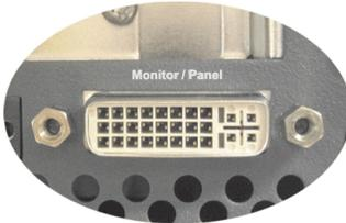
Figure 39: Monitor / Panel connection
