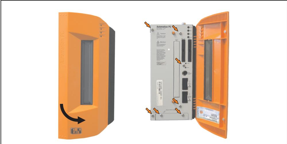
Figure 381: APC620 2PCI slots - Remove screws to install/ remove filter kit
