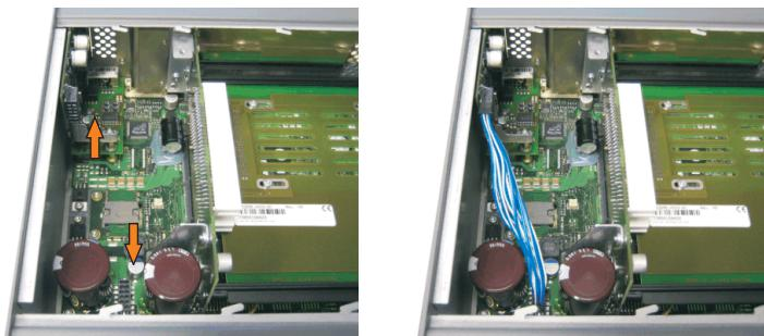
Figure 409: Plug in connection cable
