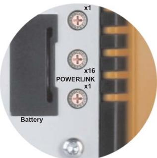
Table 39: Ethernet POWERLINK station number (x1, x16) - only APC620 embedded
