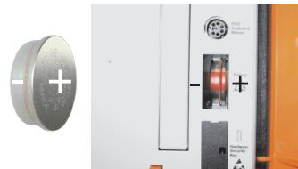
Figure 368: Battery polarity
