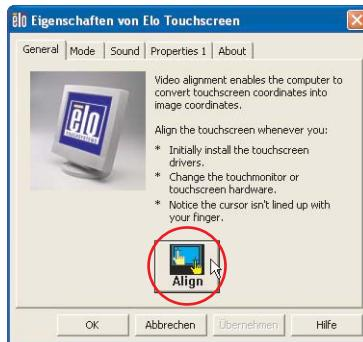
Figure 271: Touch screen calibration
