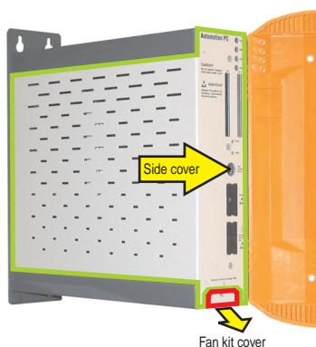
Figure 370: APC620 1PCI slot - Remove side cover and fan kit cover
