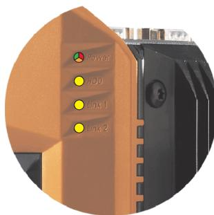
Figure 44: Front-side status LEDs
