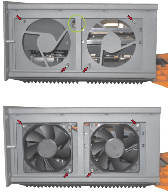
Figure 383: APC620 3PCI slot - Fan installation
