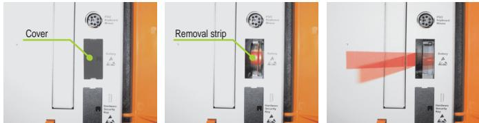
Figure 366: Battery removal
