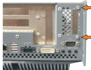
Figure 423: Remove UPS module cover
