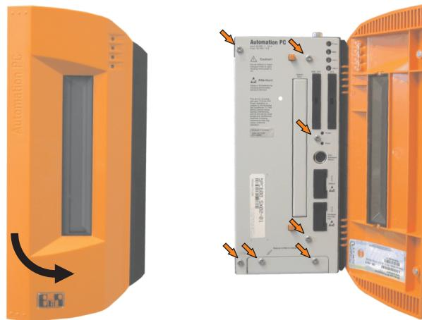
Figure 374: APC620 2PCI slots - Remove screws to install/ remove filter kit
