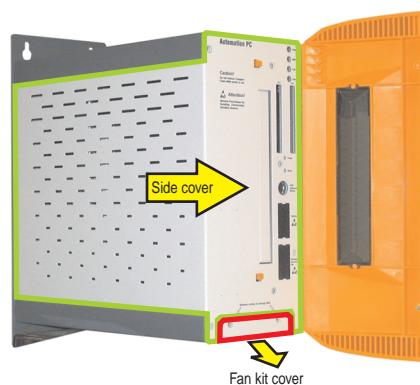
Figure 375: APC620 2PCI slots - Remove side cover and fan kit cover
