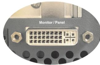
Figure 37: Monitor / Panel connection
