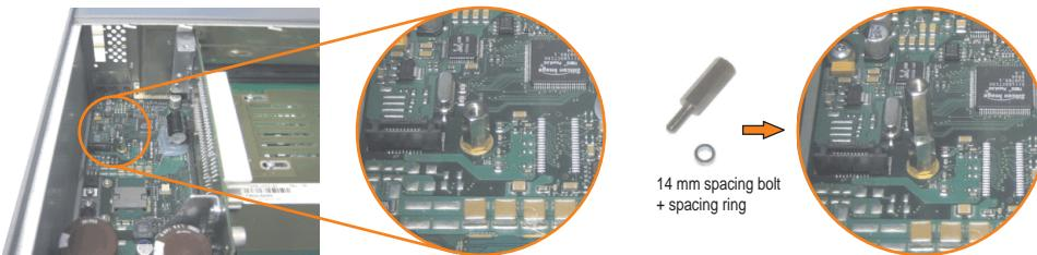
Figure 406: Screw in spacing bolt and spacing ring
