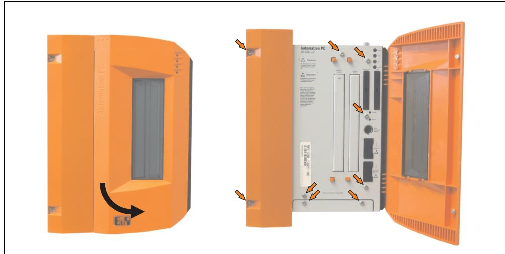
Figure 386: APC620 5PCI slot - Remove screws to install/ remove filter kit
