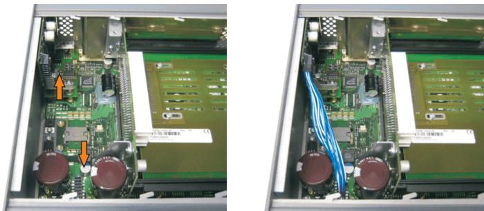
Figure 428: Plug in connection cable
