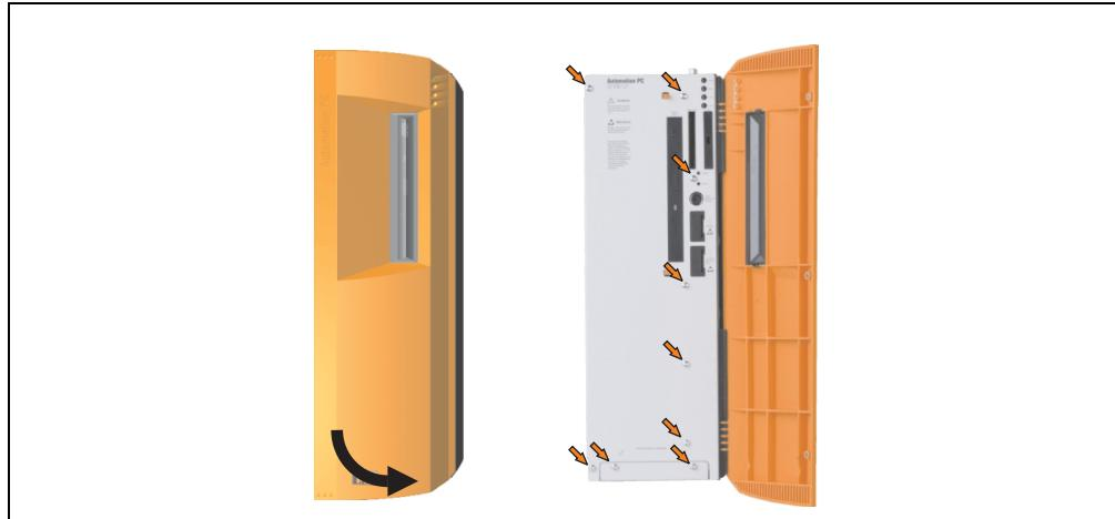
Figure 380: APC620 3PCI slot - Remove screws to install/ remove filter kit
