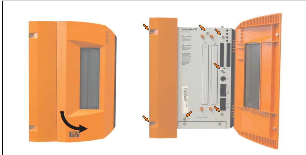
Figure 440: Mounting the side cover - APC620, 5 PCI slot
