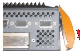
Figure 446: Removing the APC620 front cover
