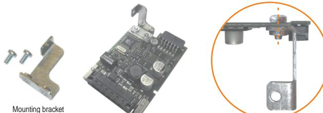
Figure 426: Install mounting bracket
