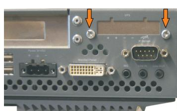
Figure 418: Remove UPS module cover
