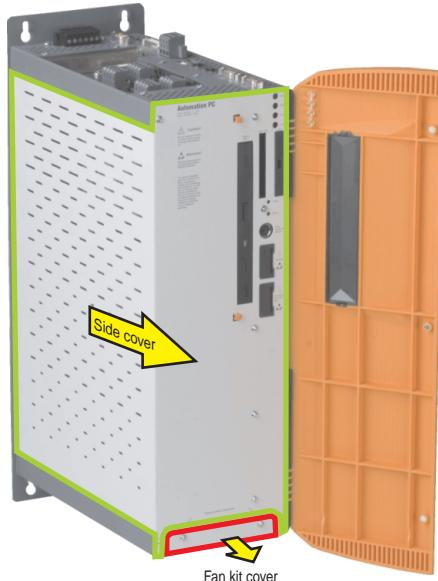
Figure 381: APC620 3PCI slots - Remove side cover and fan kit cover
