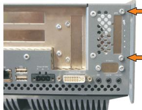
Figure 404: Remove UPS module cover
