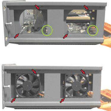
Figure 377: APC620 2PCI slots - Fan installation
