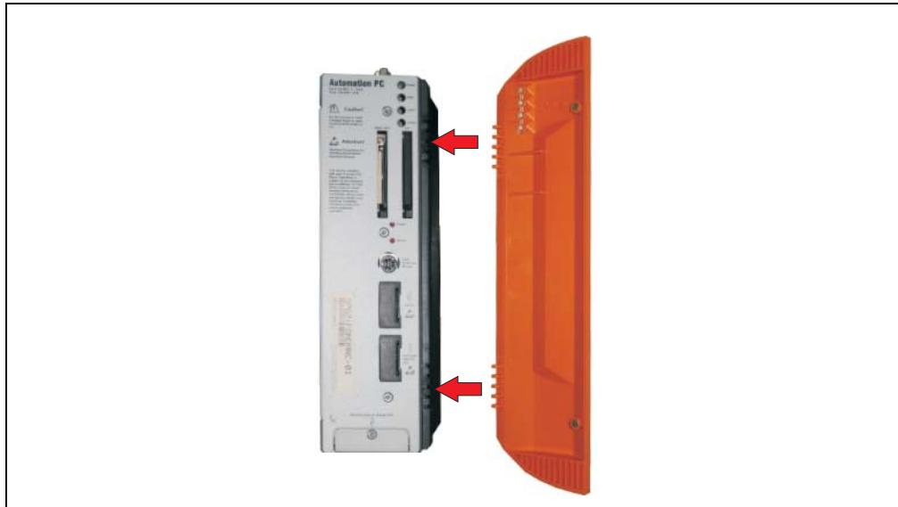
Figure 447: Attaching the front cover
