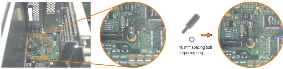
Figure 413: Screw in spacing bolt and spacing ring
