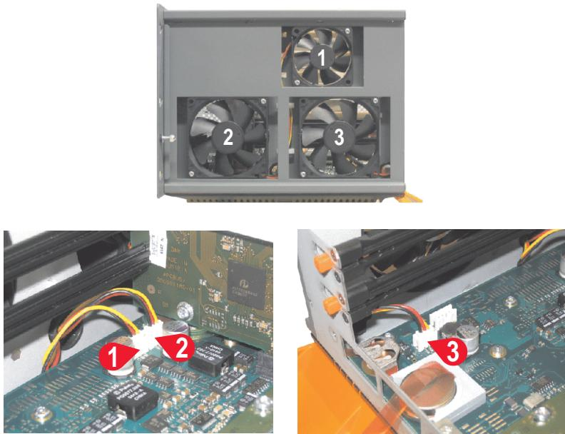
Figure 391: APC620 5PCI slot - Fan cable connection to the main board
