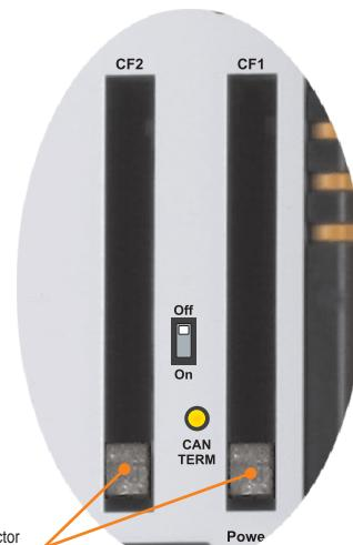
Table 63: CompactFlash slots (CF1 / CF2) - APC620 embedded
