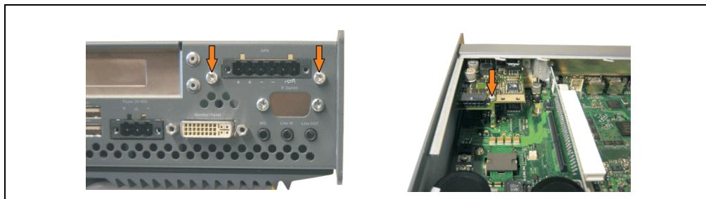
Figure 401: Install UPS module
