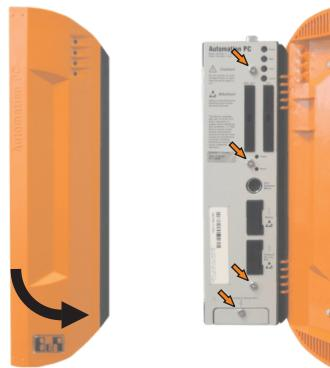
Figure 369: APC620 1PCI slot - Remove screws to install/ remove filter kit
