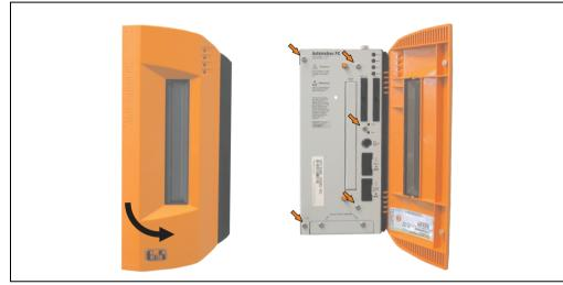
Figure 396: Mounting the side cover - APC620, 2 PCI slot
