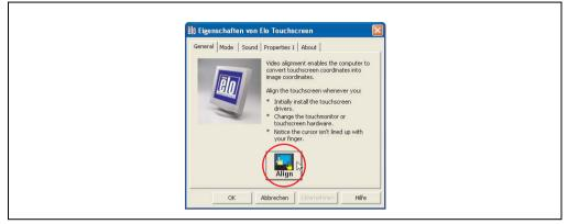
Figure 240: Touch screen calibration
