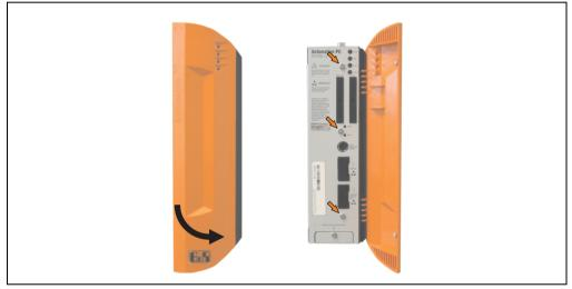
Figure 395: Mounting the side cover - APC620, 1 PCI slot
