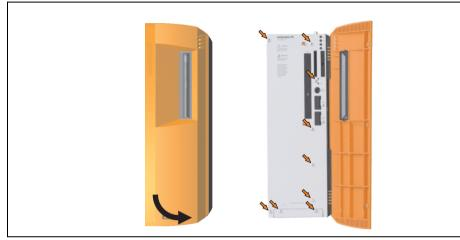
Figure 338: APC620 3PCI slot - Remove screws to install/ remove filter kit
