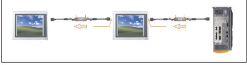
Figure 305: Example of the signal direction display - SDL flex cable with extender
