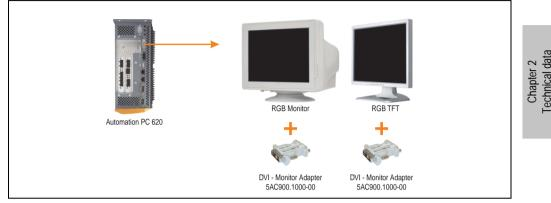
Figure 30: Monitor / Panel connection with RGB video signal
