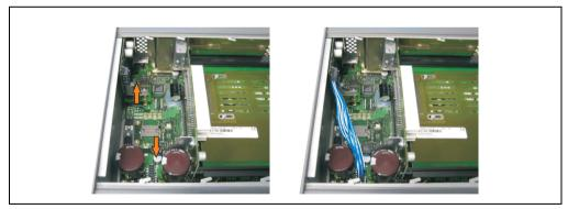
Figure 367: Plug in connection cable
