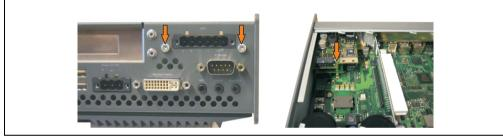
Figure 378: Install UPS module
