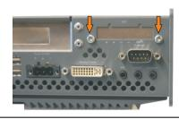
Figure 376: Remove UPS module cover
