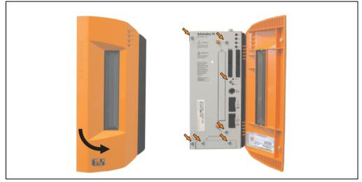
Figure 332: APC620 2PCI slots - Remove screws to install/ remove filter kit
