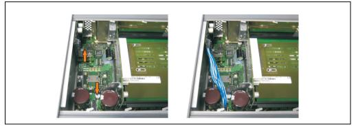
Figure 386: Plug in connection cable
