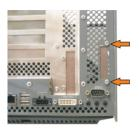
Figure 388: Remove UPS module cover
