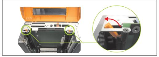
Figure 353: Release the slide-in slot releasing mechanisms
