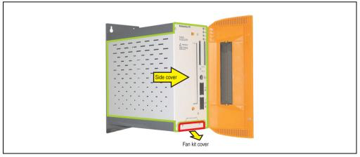
Figure 333: APC620 2PCI slots - Remove side cover and fan kit cover
