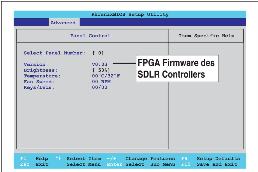
Abbildung 120: Firmwareversion des Automation Panel Link SDL Transceiver/Receiver
